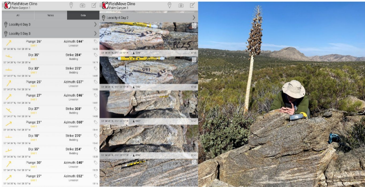
Figure 5: Left: FieldMove Clino application used to record field observations and verified in image on right with Standard Transit Brunton Compass.
