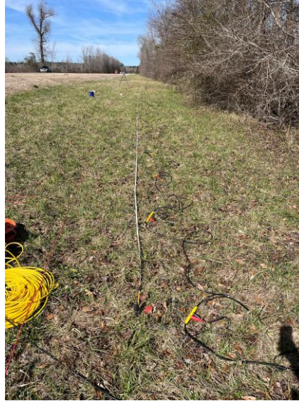
Figure 4-14: Greensboro seismic survey line
