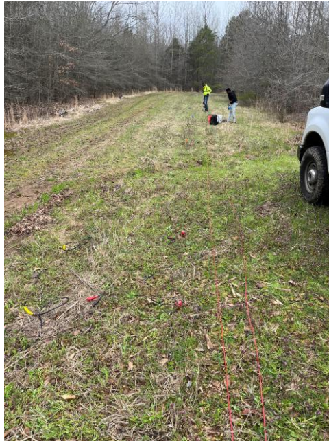
Figure 4-22: Seismic refraction survey line at Lauderdale County site
