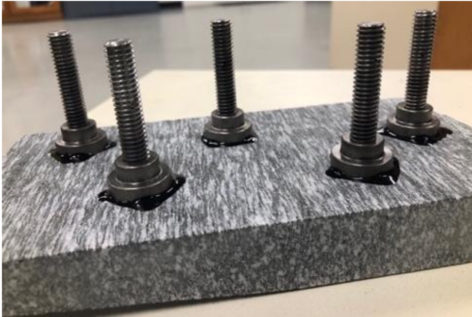
Figure 7. BBS Specimen Assembly showing Pull-off Stubs bonded to a Granite Substrate
