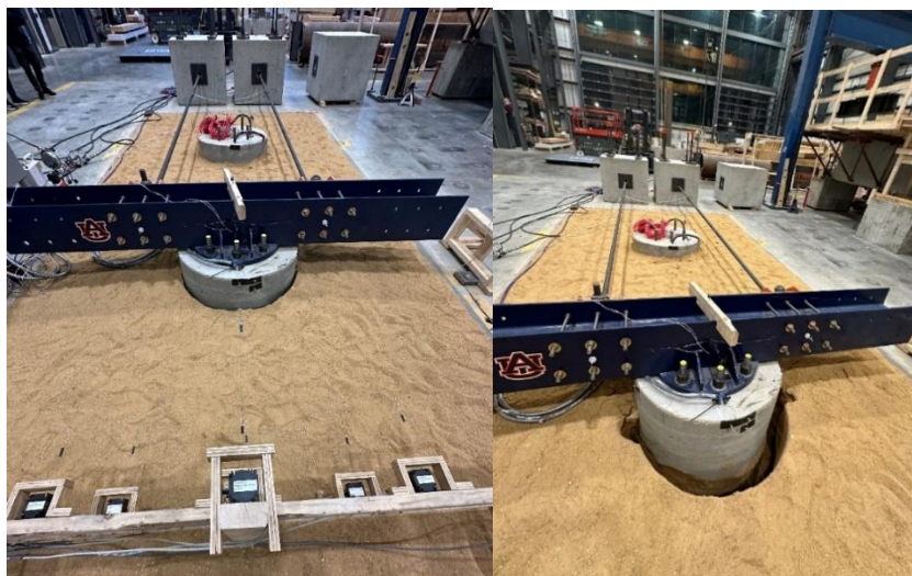
Figure 4-21. Purely lateral test B prior to and after failure.
