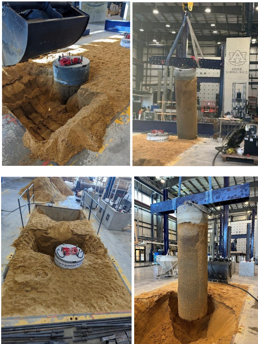
Figure 4-18. Excavation and exhumation of the shafts
