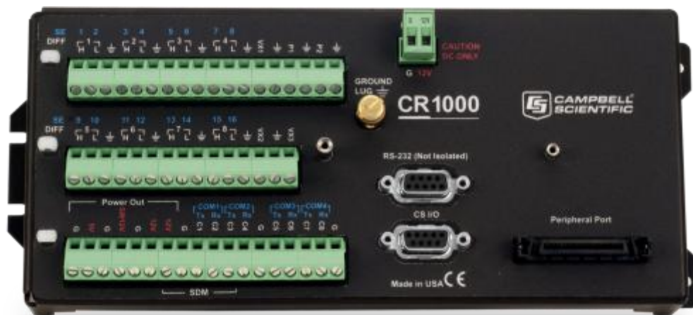
Figure 3-31. CR1000 data logger (Campbell Scientific, n.d.)
