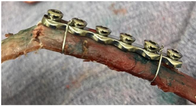
Figure 25 New fracture at the dorsal plate and bone interface in the MRP.
