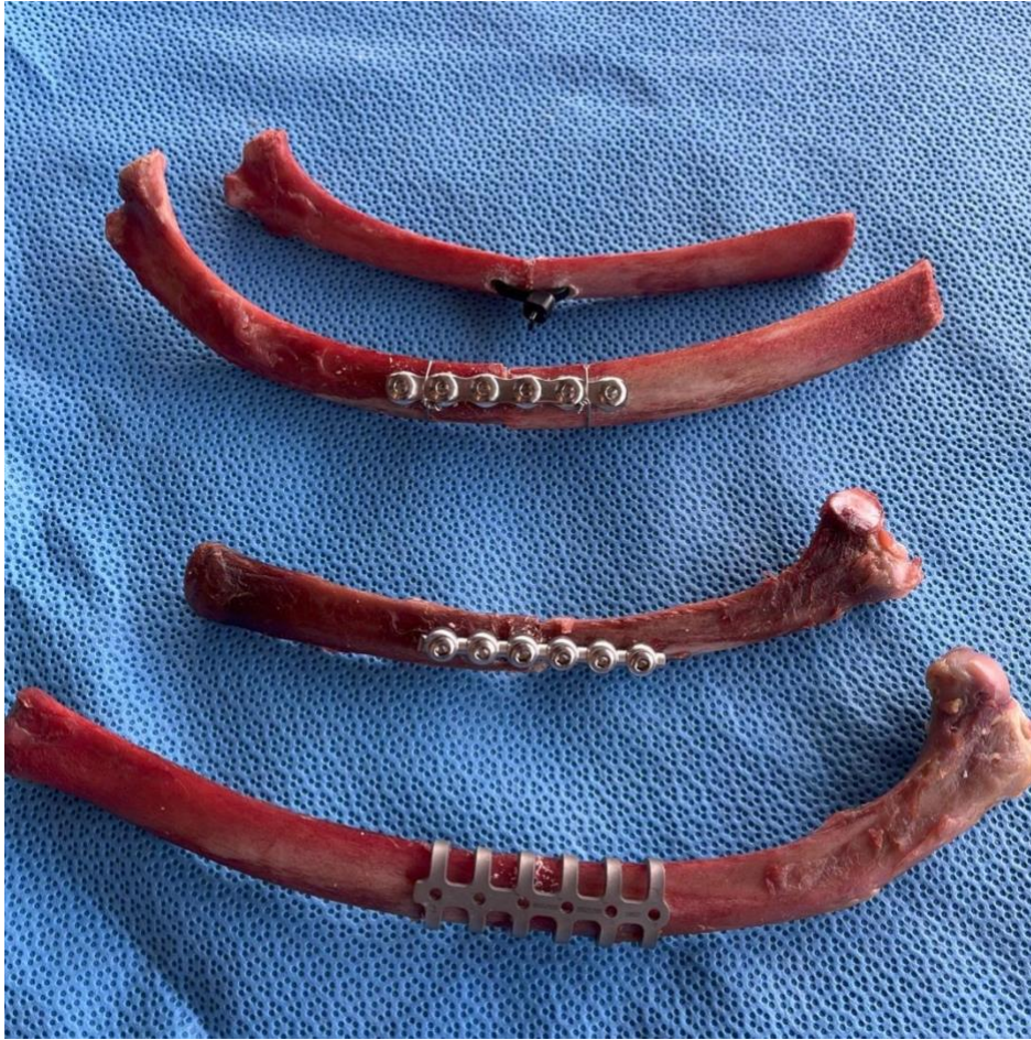
Figure 17 Resected ribs that have been fractured and then repaired using the following methods described from top to bottom: 4 mm nylon cable tie (NCT), 2.7 mm string of pearls veterinary locking plate (SOP), 2.7 mm reconstruction plate modified to accommodate 3.2 cortical screws with cerclage wire applied (MRP), and STRACOS™ Titanium 3D rib clip (RC).
