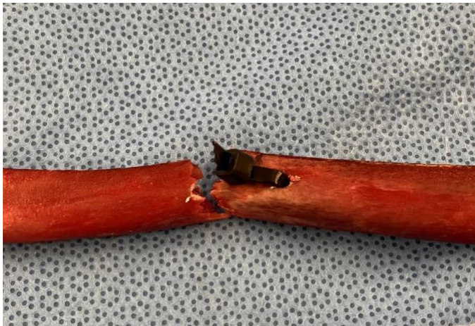
Figure 23 Fail at the original fracture line for the NCT.
