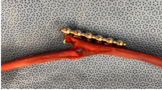
Figure 24 Screw pullout in the SOP plate.
