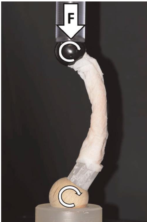
Figure 9 Axial compression testing of a human rib. (Mischler, 2022)
