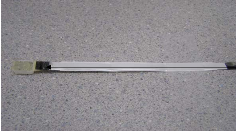
Figure 3.3 Electrode array in glass substrates with vacuum attachment.
