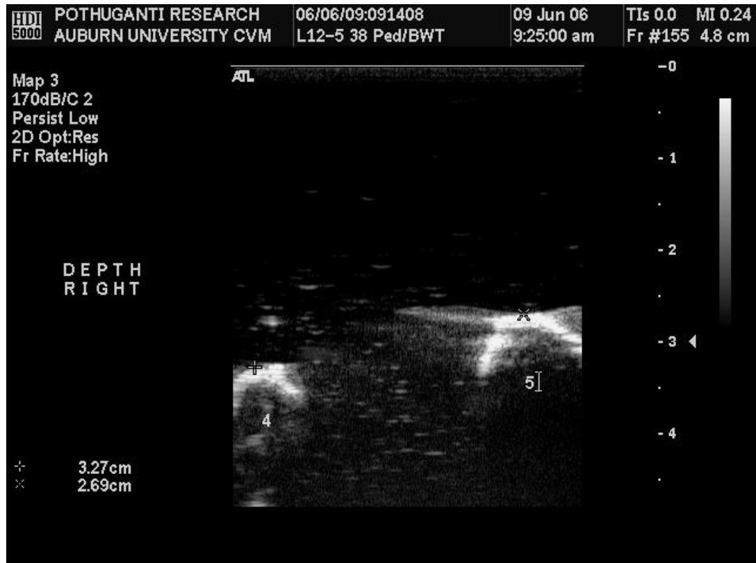
Figure 6.18: Depth of L4 and L5 transverse process from the gelatin surface
