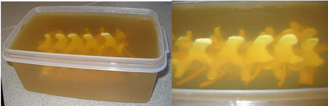
Figure 6.10: Artificial lumbar spine in the gelatin solution
