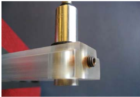
Figure 6.4: Slider holding the transducer at a fixed position
