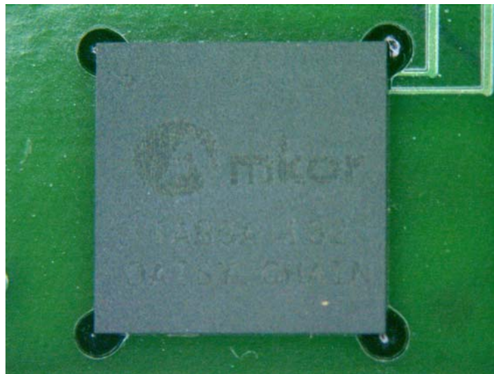
Figure 2.8 CSP Placed into Corner Dot Underfill.
