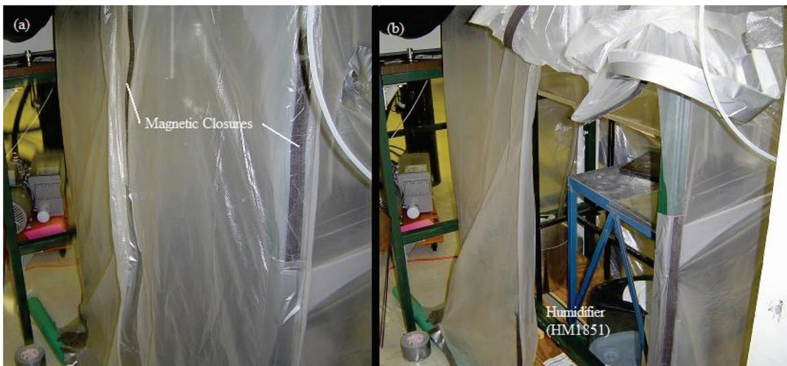
Figure 4.14. An image of the constant humidity enclosure access flap (a) closed (b) open.
