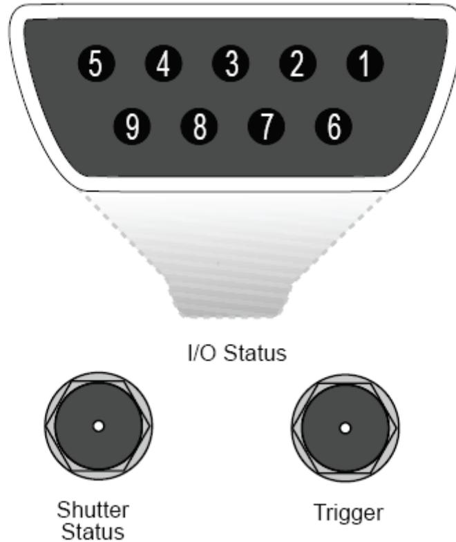
Figure A.1. Diagram of Photometrics 300 CCD camera controller outputs and inputs.
