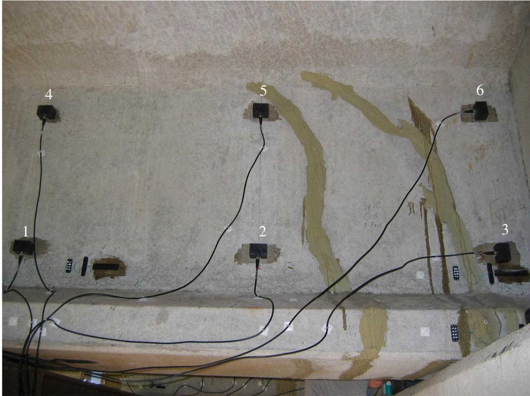
**Figure 7-8:** Sensor locations on Span 10 Girder 8
