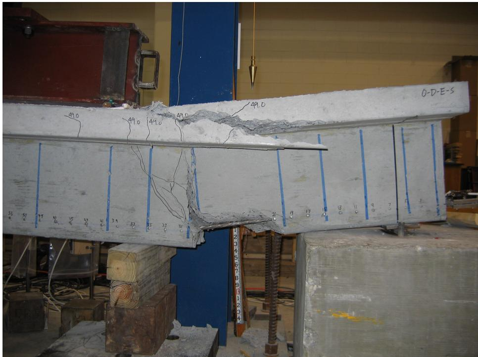
**Figure 3-16:** STD-M-D shear-tension failure (Levy 2007)
