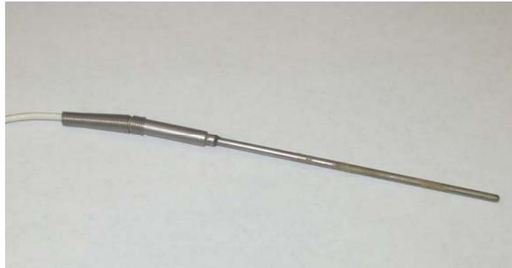
**Figure 4.8:** Thermistor Probe
