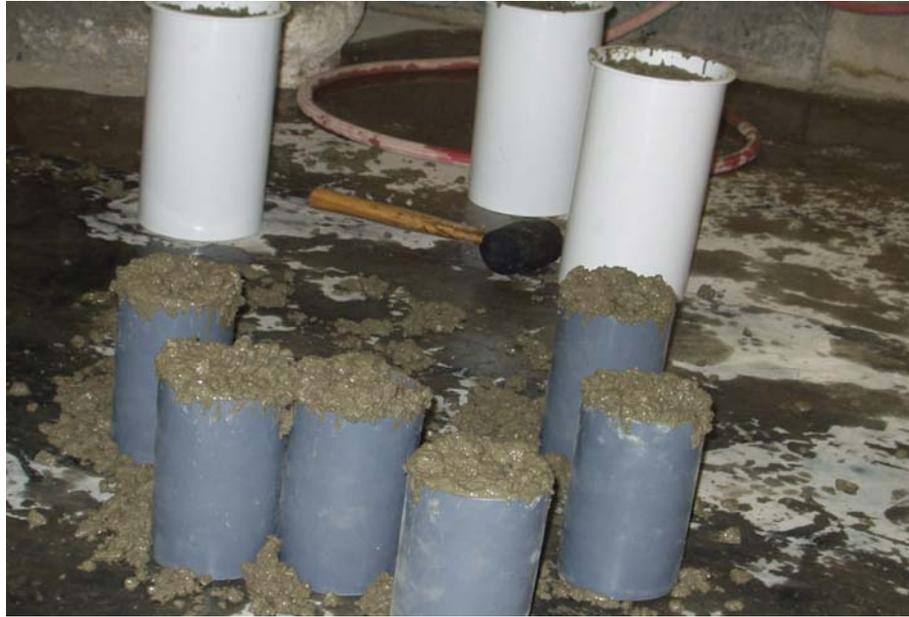
**Figure 4.13:** Concrete samples being made in the Laboratory
