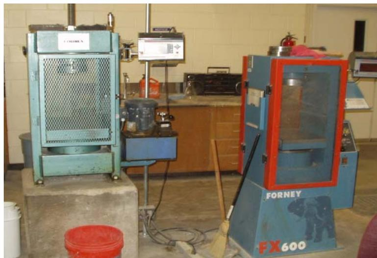
**Figure 4.15:** Forney compressive testing machines
