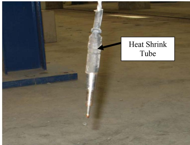
**Figure 4.4:** Typical Linear Variable Differential Transformer
