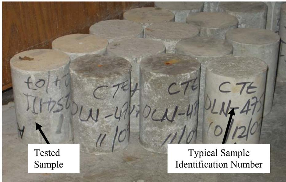
**Figure 4.14:** Typical tested samples ready to be discarded
