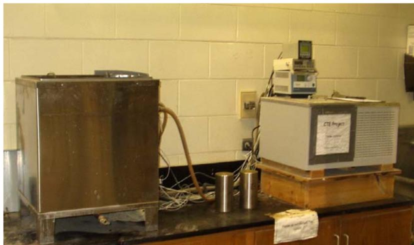
**Figure 4.10:** AASHTO TP 60 (2004) Test setup
