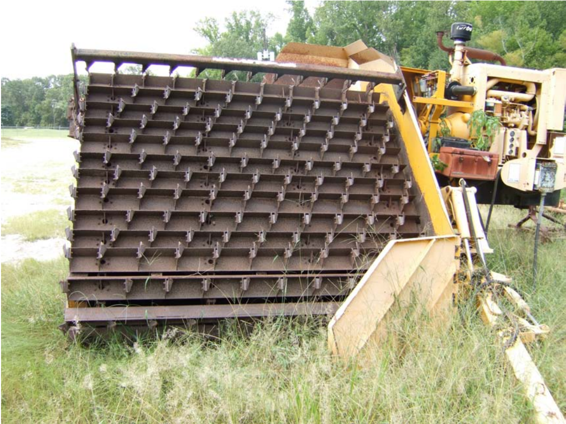
Figure 2. Picture of windrow turning machine (SCAT Engineering, Inc., Hopkinton, IA). Machine is pulled by a tractor of at least 100 horsepower.
