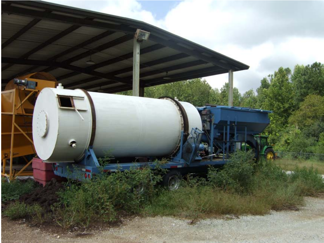
Figure 3. Picture of in-vessel composter (BW Organics, Inc., Sulphur Springs, TX).
