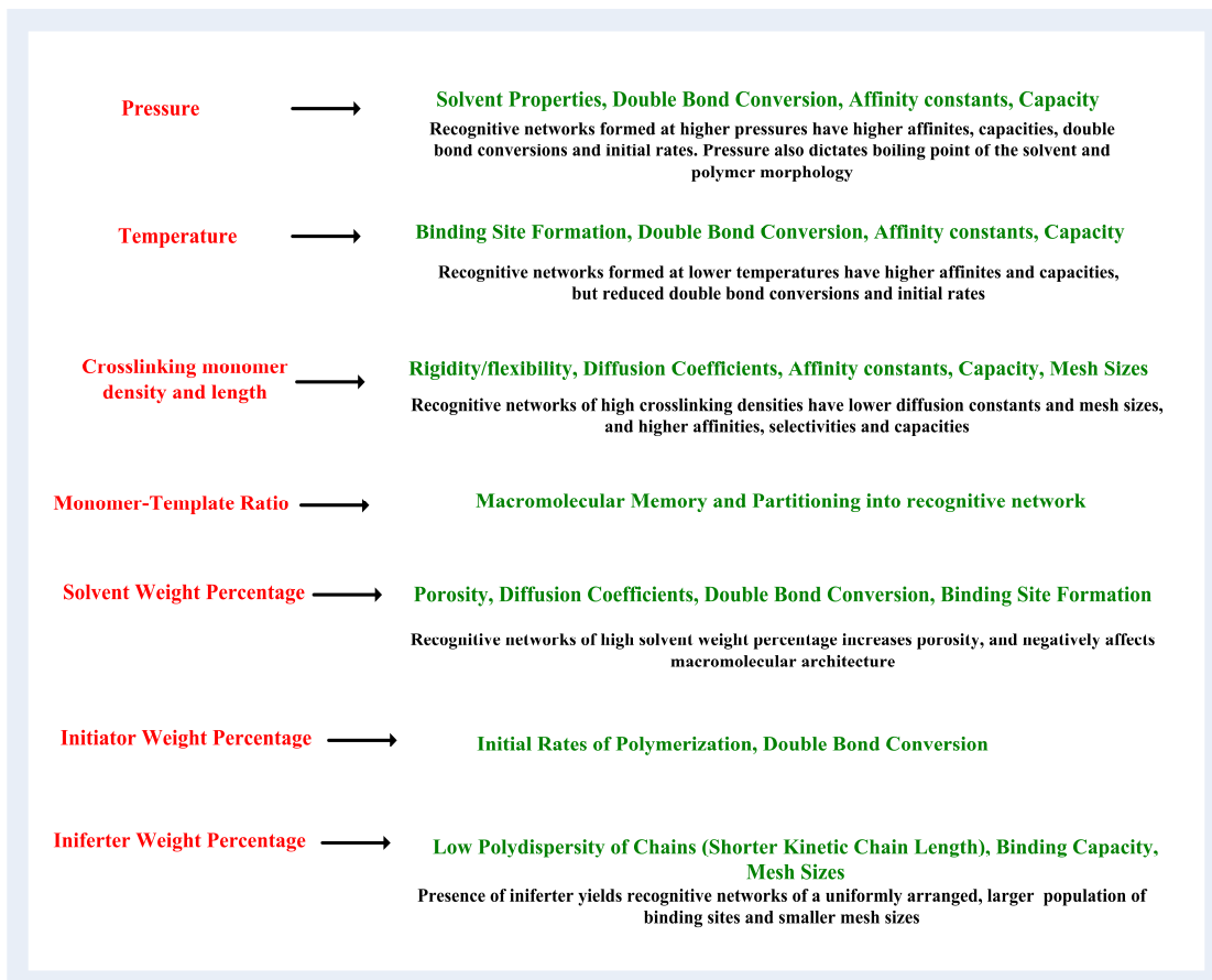
Figure 3.3 Design Parameters of a Hydrogel. The macromolecular structure of imprinted polymer networks, and hence in effect the template binding parameters, can be controlled by tuning various environmental and compositional parameters.
