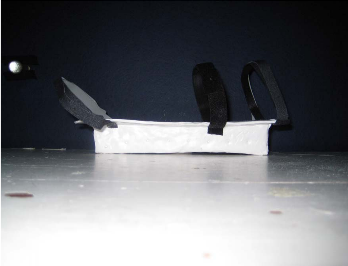
Figure 9- Outersole and fulcrum for creating 25° of inversion upon landing, side view.
