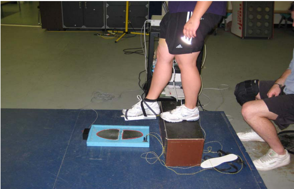
Figure 21- Participant waiting to perform drop landing with outsole and fulcrum, side view.
