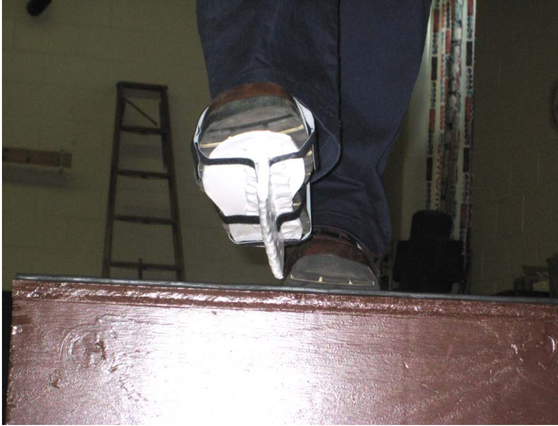
Figure 10- Box and outersole with fulcrum used for testing.
