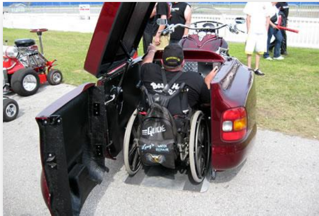
Figure 25 Motorcycle/Trike for the Handicapped, the door on the back of the motorcycle opens up wide enough to drive a wheelchair onto the lift for storage during transportation. (Crowe, 2008)
