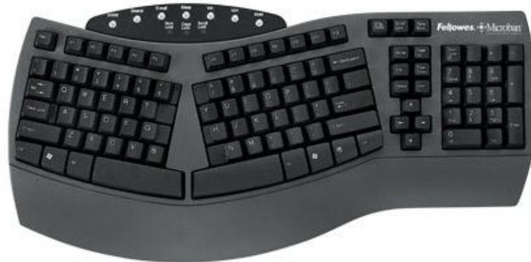
Figure 24 Split, angled keyboard allows user to maintain neutral position from elbow to fingers. (ergoware, 2008)
