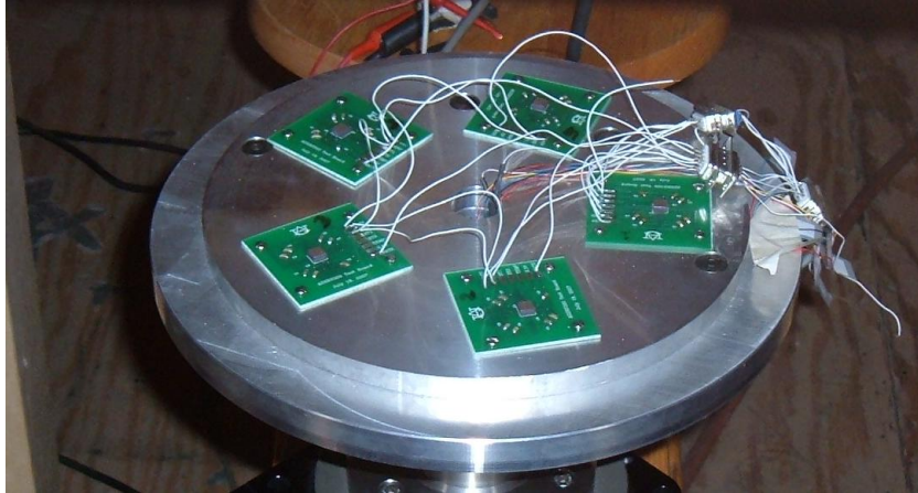
Figure 4.1: Gyroscopes mounted to the rate table
