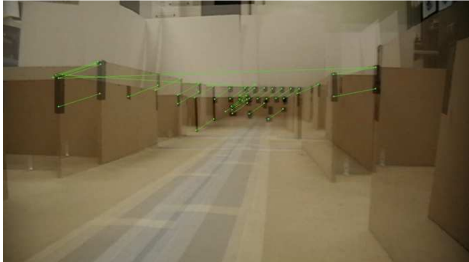
Figure 5.4: SIFT feature matches between left and right images at (20,0) .
