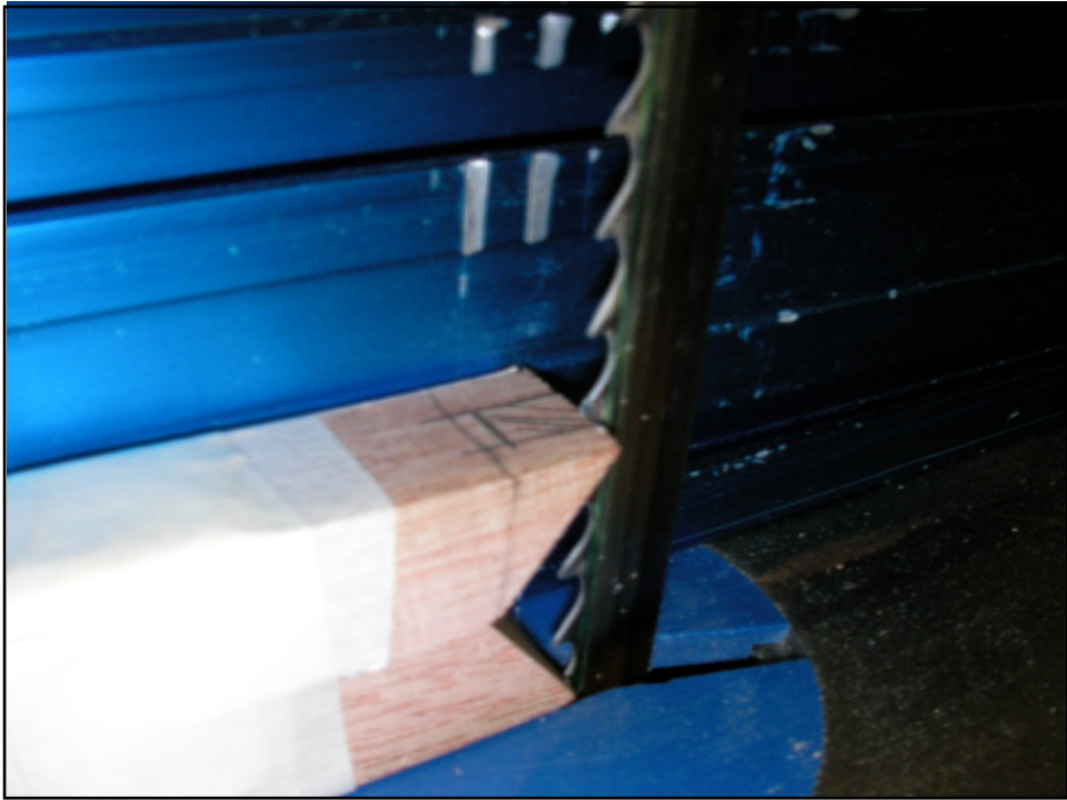
Figure 78: Cut the hole for the tenon joint
