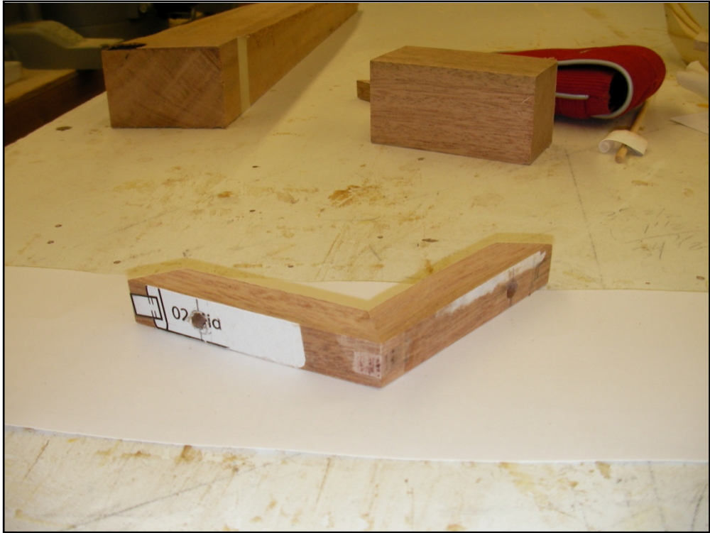
Figure 82: Finished tenon joint
