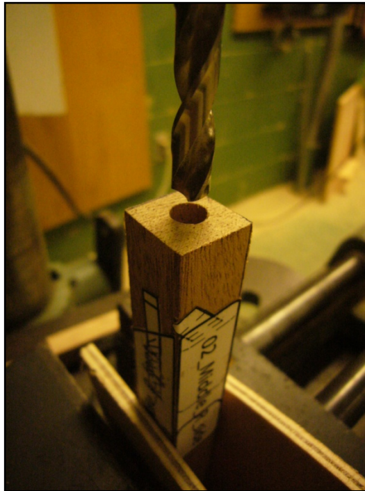
Figure 76: Before cutting this wood, the dowel joint must be drilled
