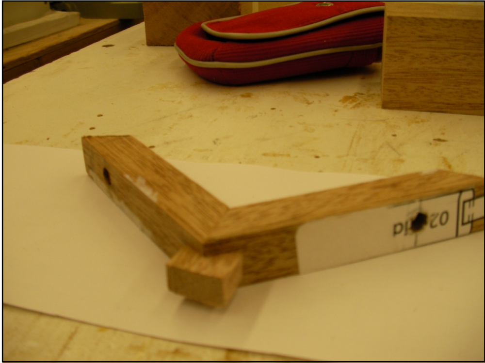
Figure 80: Insert a piece of wood into the hole to form the tenon joint
