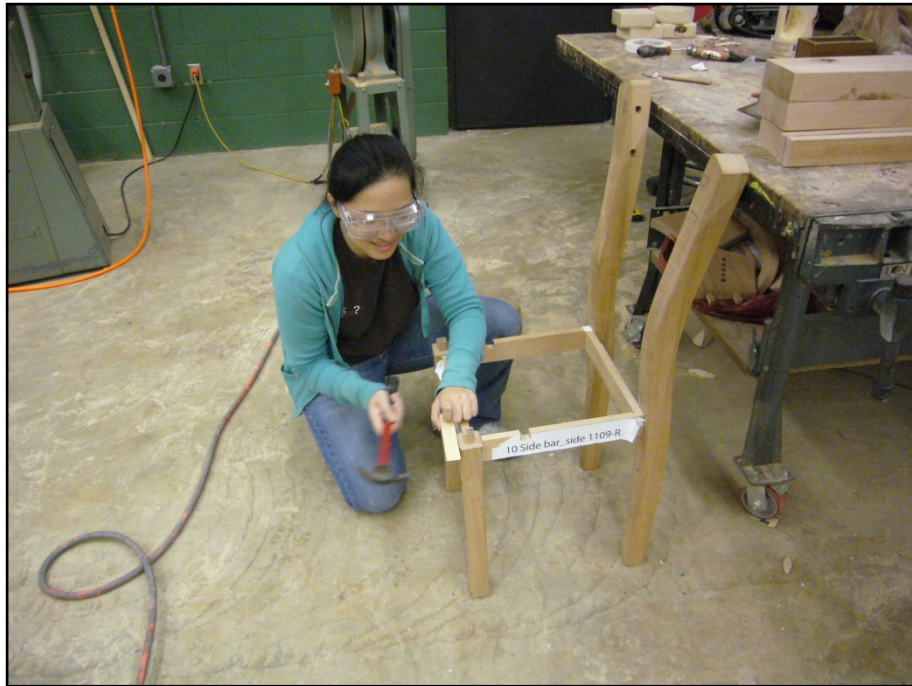
Figure 84: Securing the tenon joint using a hammer
