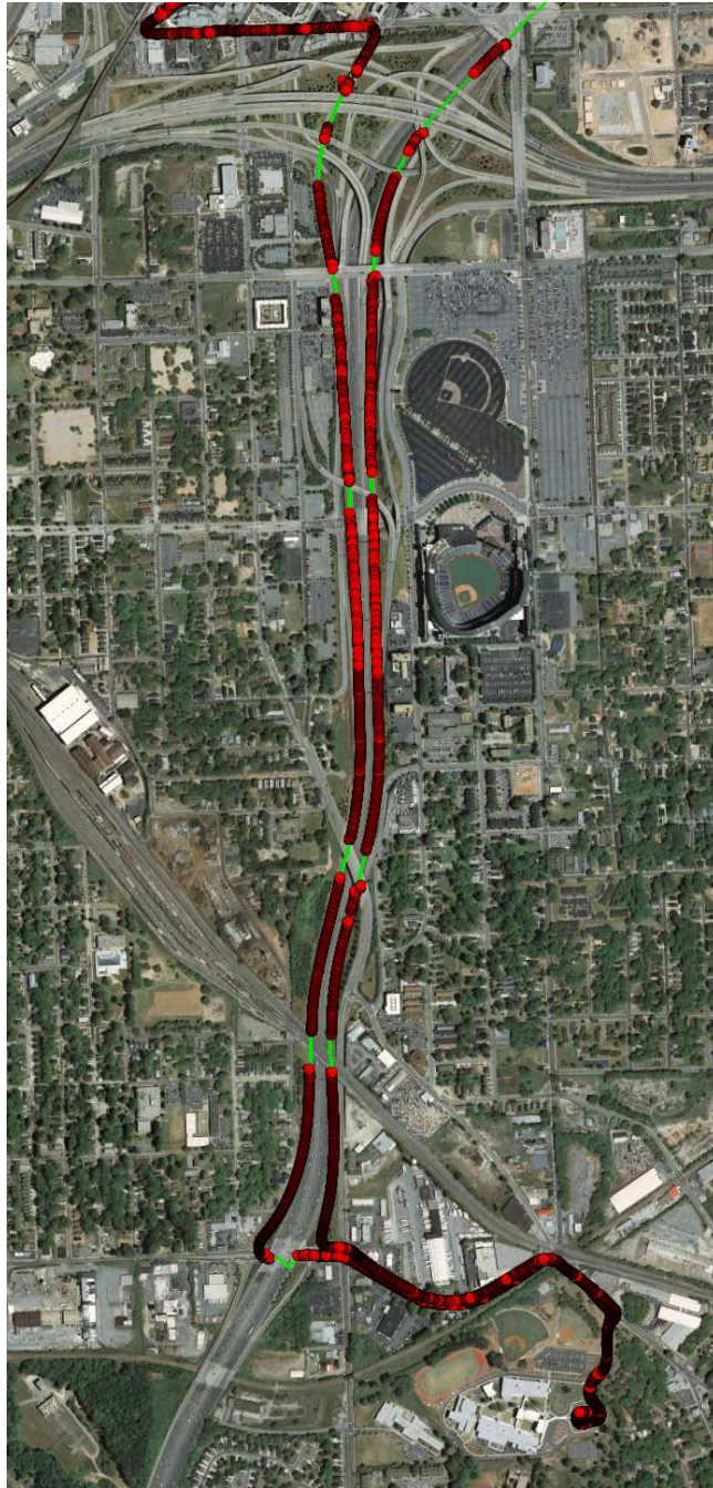
Figure 10.26: Position Estimates of the VDFLL and NovAtel Overladed on a Map of Atlanta (from Google Earth and GPS Visualizer)
