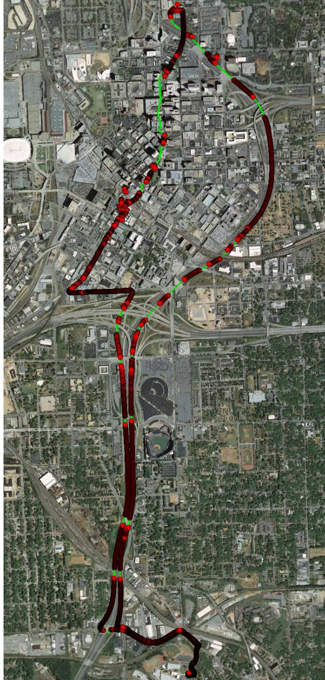
Figure 10.21: Position Estimates of the VDFLL and NovAtel Overladed on a Map of Downtown Atlanta (from Google Earth and GPS Visualizer)
