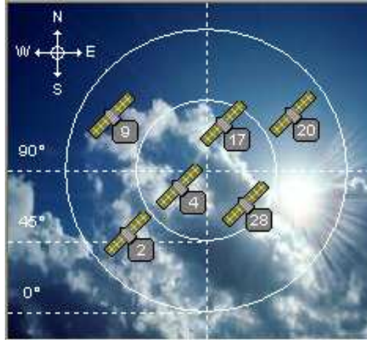
Figure 10.10: Skyplot of Visible Satellites for the Second Data Set (from NordNav Receiver)
