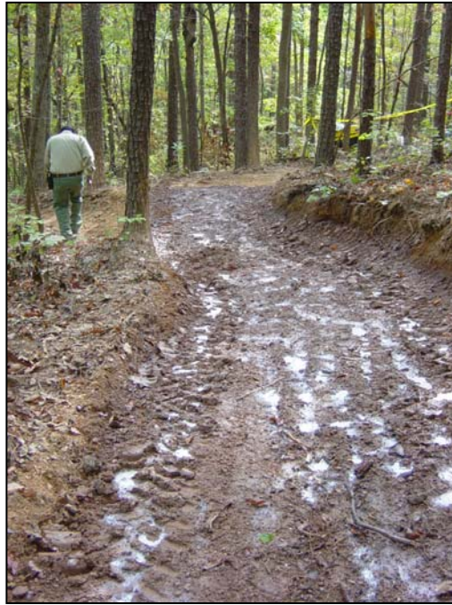
Figure 3.9 – Plot soaked in Envirotac II
