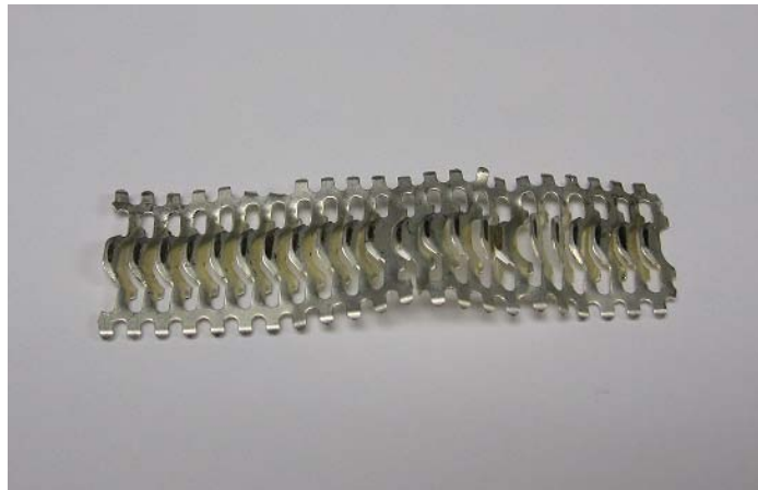
Figure 7 – Connector Spring in Round Pin, High Power Connector.
