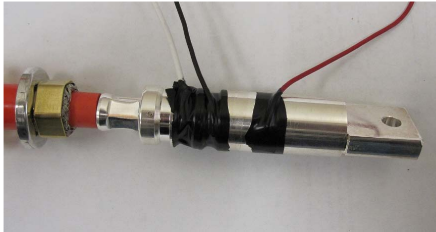
Figure 11 – Placement of the Thermocouples on Connector for the Experiment.
