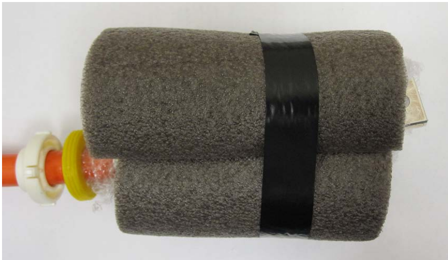
Figure 10 – Connector with bubble wrap and insulating foam.
