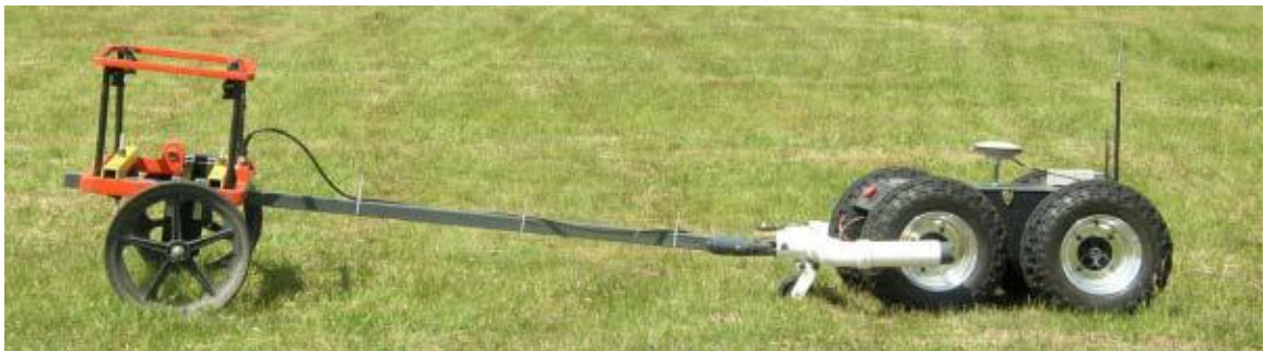
Figure C.1: A Segway RMP towing a trailer containing geophysical equipment.
