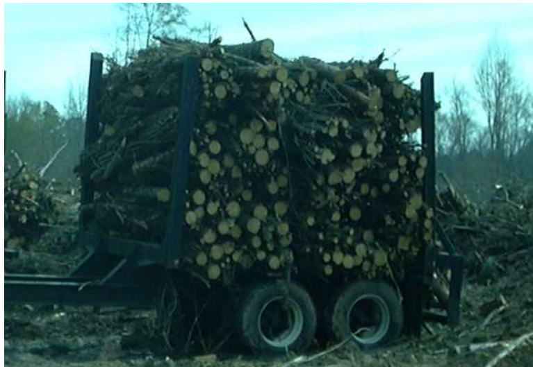
Figure 9. Eight-foot bundle load configuration
