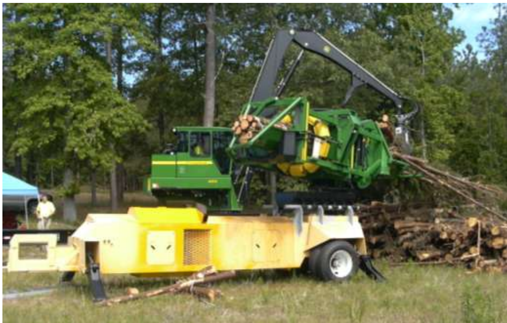
Figure 6. First bundle produced by the prototype bundler in Auburn, Alabama.
