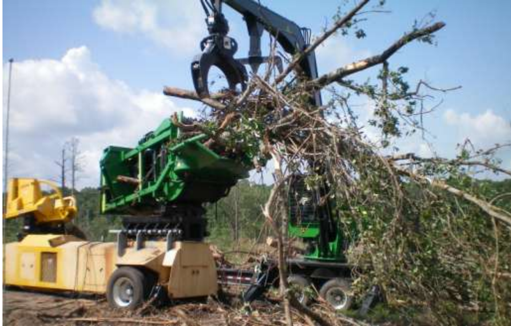
Figure 7. Bundling hardwood slash at the Midway, AL test site.
