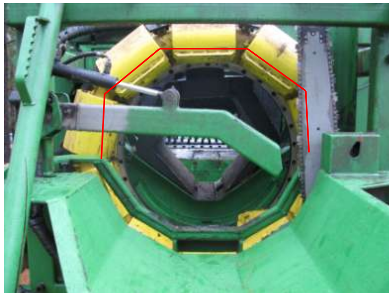
Figure 13. Location of the hold down bar protection.
