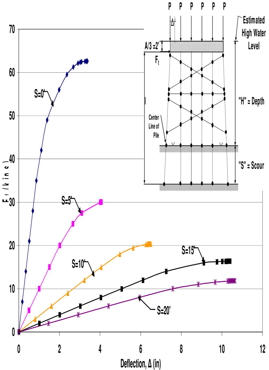
Figure A.98 HP10x42 Two-Story Single X-Braced 6-Pile Bent with  $H=21'$ ,  $P=120$ kips and  $A=6'$  Pushover Analysis Results
