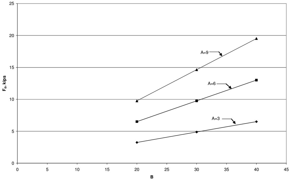
Figure 2.5 Debris Raft Force,  $F_T$ , for Various Debris Raft Dimensions (B) and (A) with  $V_{\text{design}} = 6$  mph
