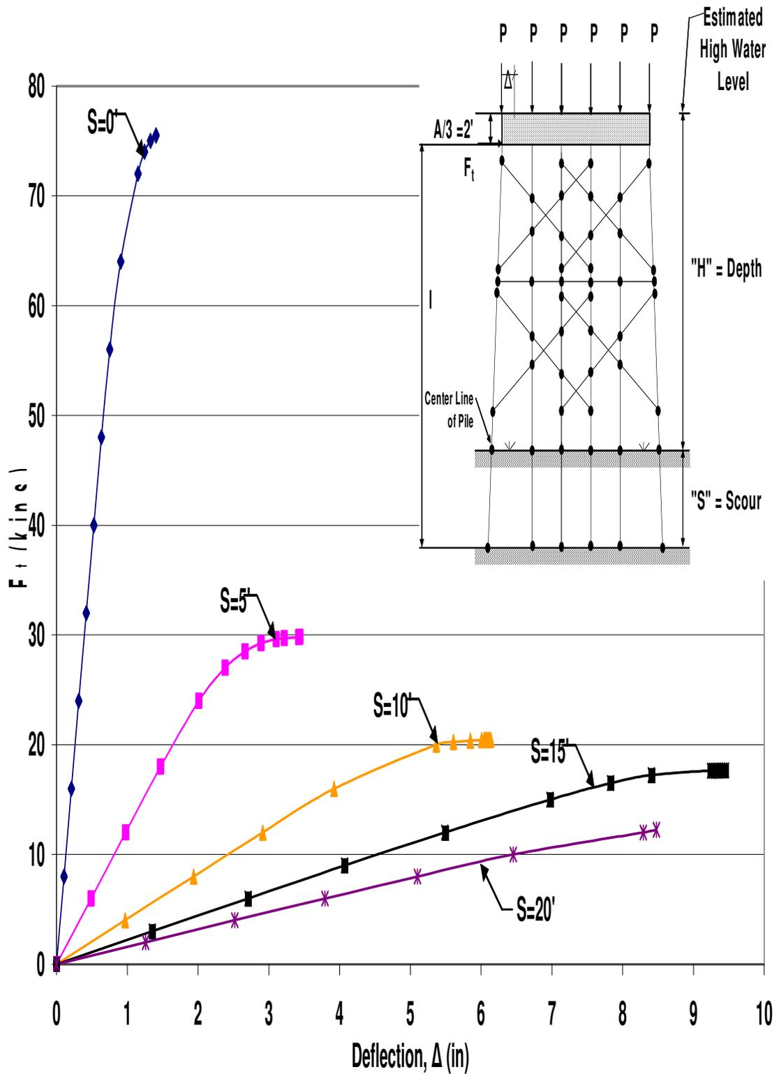
Figure A.110 HP10x42 Two-Story Double X-Braced 6-Pile Bent with  $H=25'$ ,  $P=120$ kips and  $A=6'$  Pushover Analysis Results
