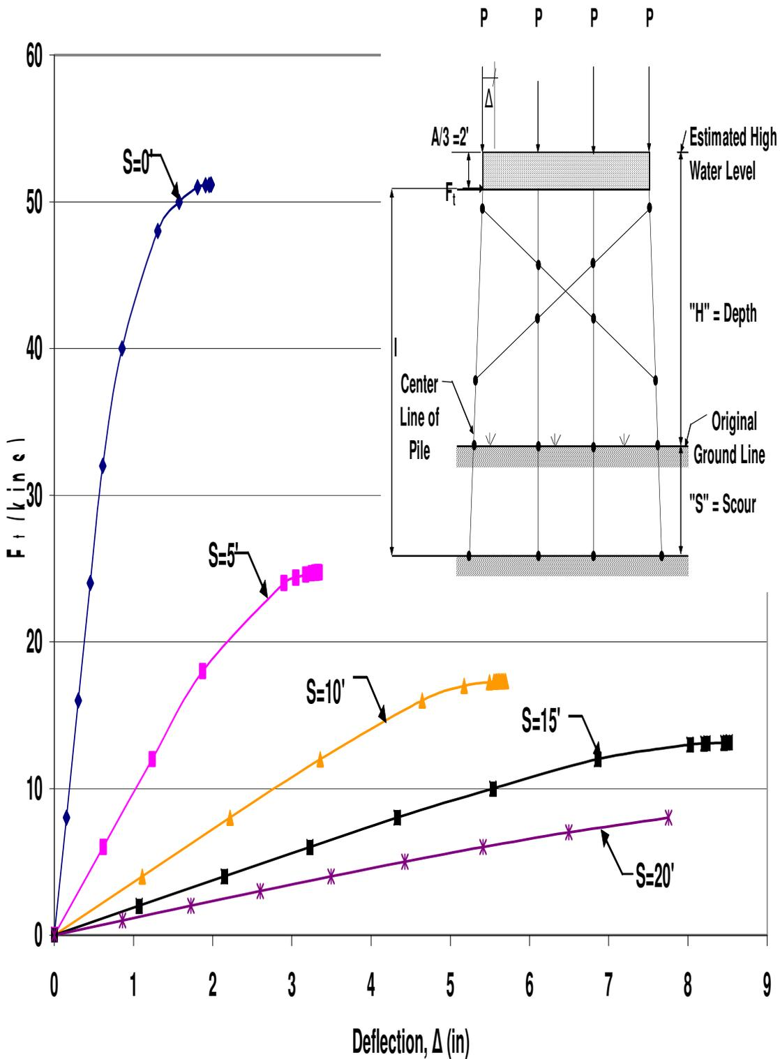
Figure A.34 HP10x42 X-Braced 4-Pile Bent with  $H=13'$ ,  $P=120$ kips and  $A=6'$
