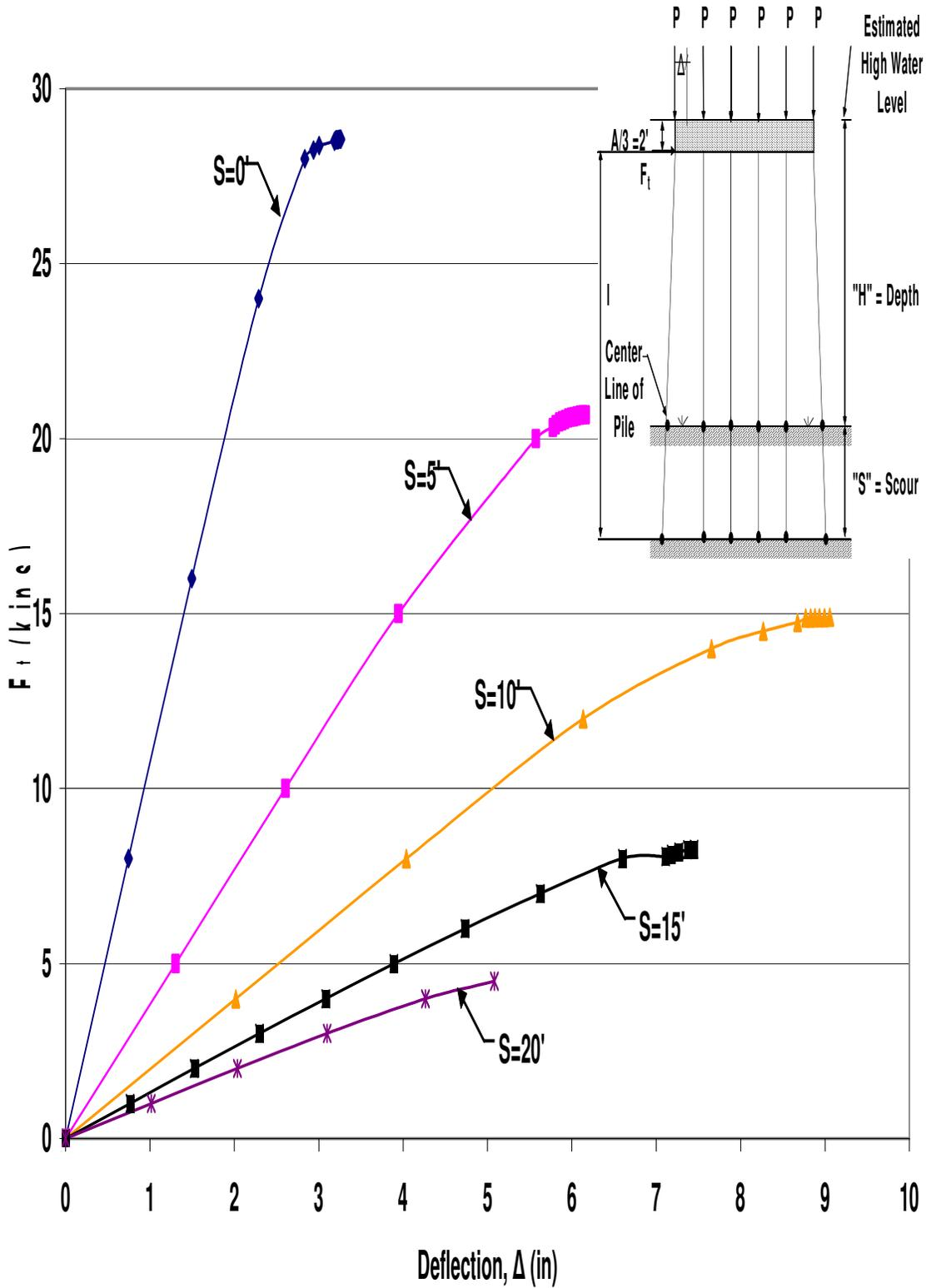
Figure A.80 HP10x42 Unbraced 6-Pile Bent with  $H=13'$ ,  $P=160$ kips and  $A=6'$
