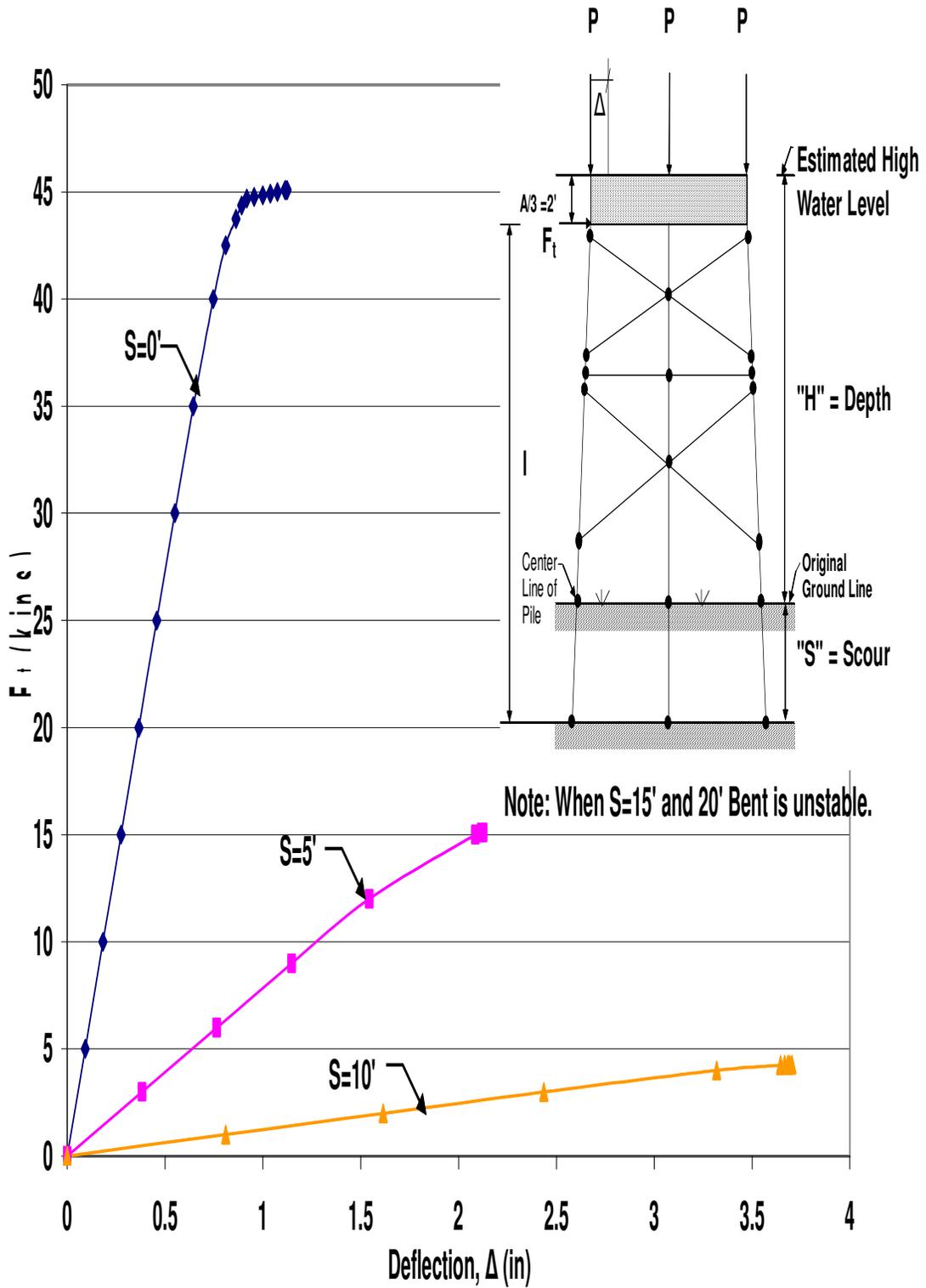
Figure A.18 HP10x42 Two-Story X-Braced 3-Pile Bent with  $H=21'$ ,  $P=120$ kips, and  $A=6'$
