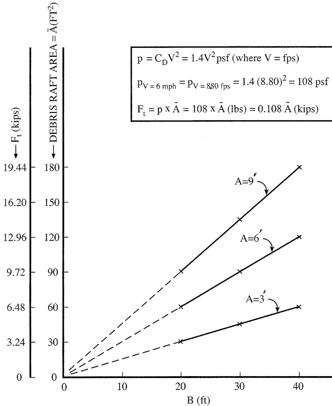
Figure 4.6 Bent  $F_t$  Force for Various Debris Raft Dimensions for  $V_{\text{Design}} = 6\text{mph}$
