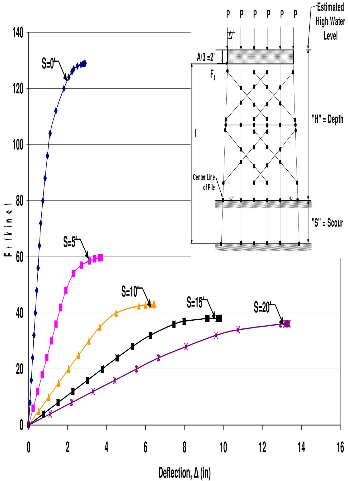
Figure B.106 HP12x53 Two-Story Double X-Braced 6-Pile Bent with  $H=21'$ ,  $P=120$ kips and  $A=6'$  Pushover Analysis Results
