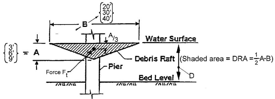
B is determined based on bridge span length, L, as follows:
