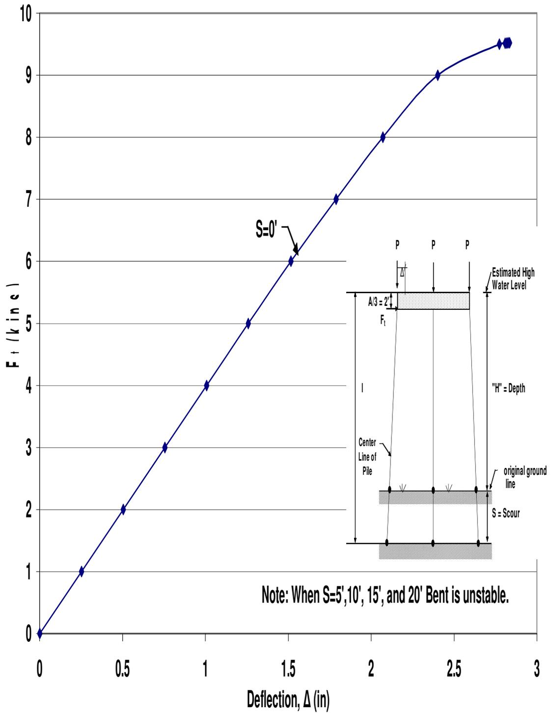
Figure A.8 HP10x42 Unbraced 3-Pile Bent with  $H=13'$ ,  $P=160$  kips and  $A=6'$
