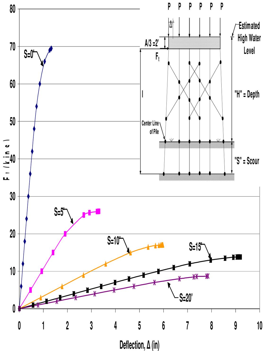
Figure A.95 HP10x42 Double X-Braced 6-Pile Bent with  $H=17'$ ,  $P=140$  kips and  $A=6'$
