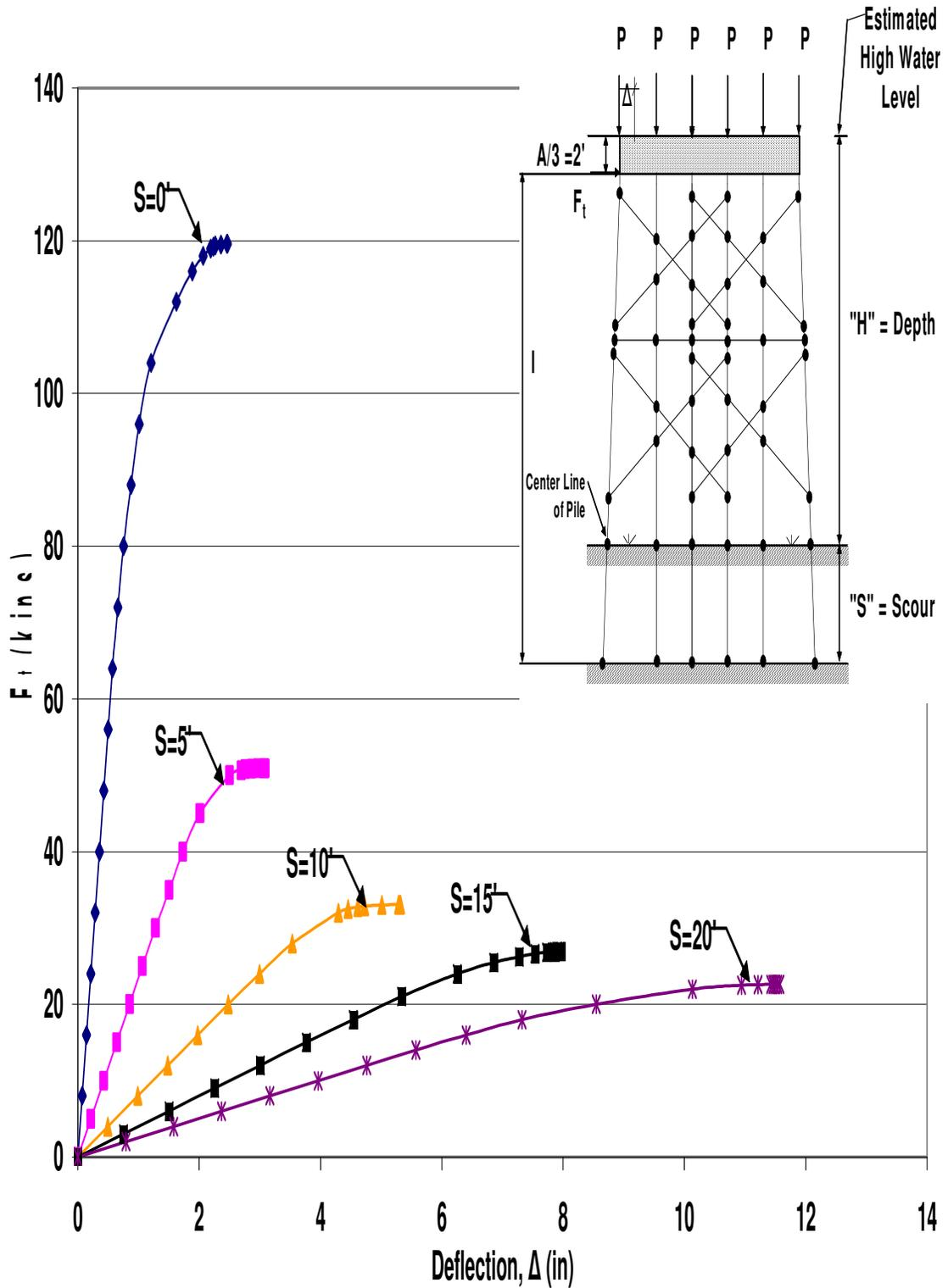
Figure B.108 HP12x53 Two-Story Double X-Braced 6-Pile Bent with  $H=21'$ ,  $P=160$ kips and  $A=6'$  Pushover Analysis Results
