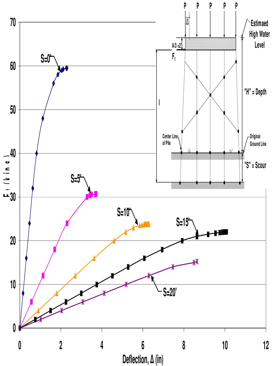
Figure A.58 HP10x42 X-Braced 5-Pile Bent with  $H=13'$ ,  $P=120$ kips and  $A=6'$
