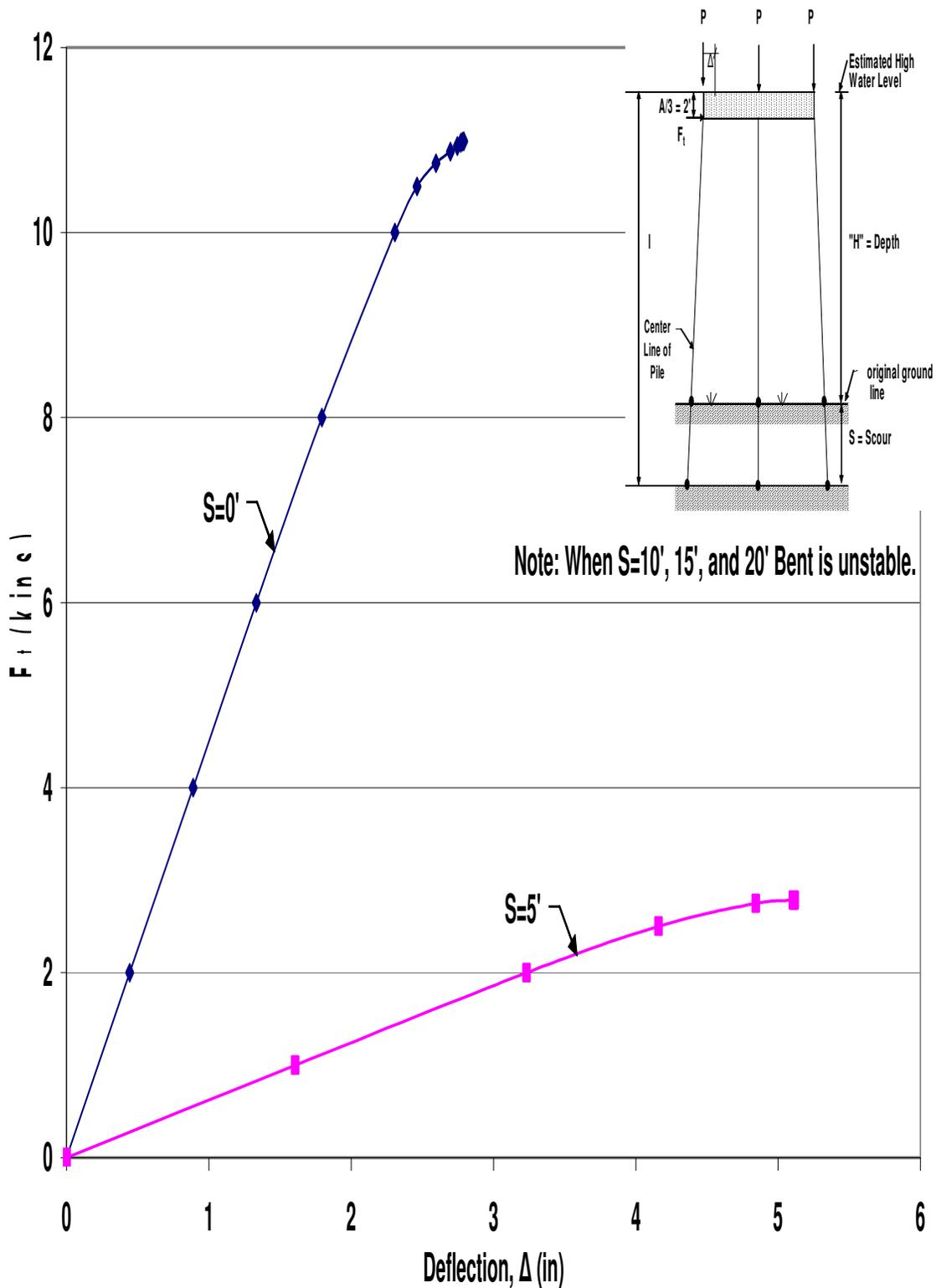
Figure A.7 HP10x42 Unbraced 3-Pile Bent with  $H=13'$ ,  $P=140$ kips and  $A=6'$
