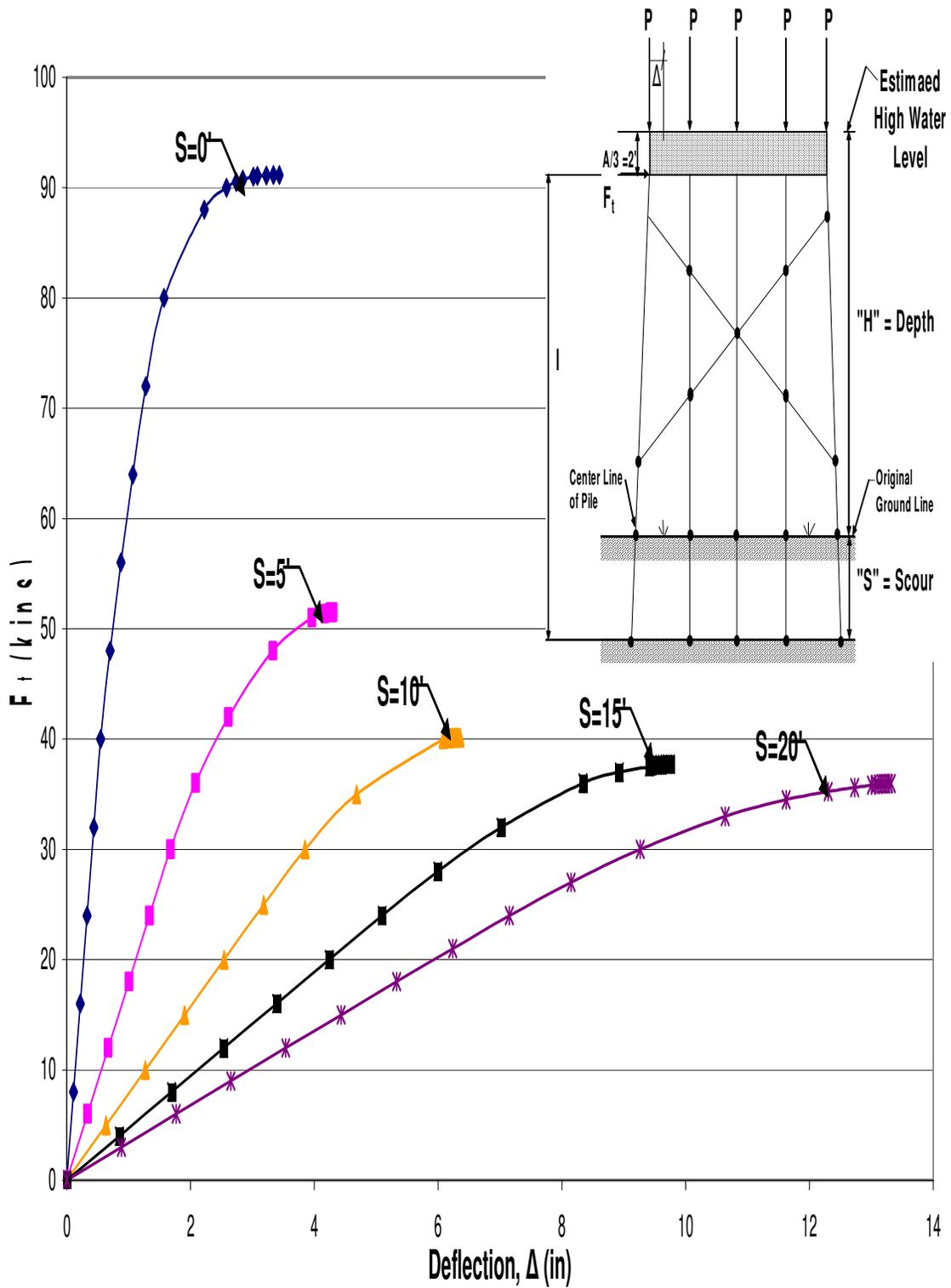
Figure B.58 HP12x53 X-Braced 5-Pile Bent with  $H=13'$ ,  $P=120$ kips and  $A=6'$
