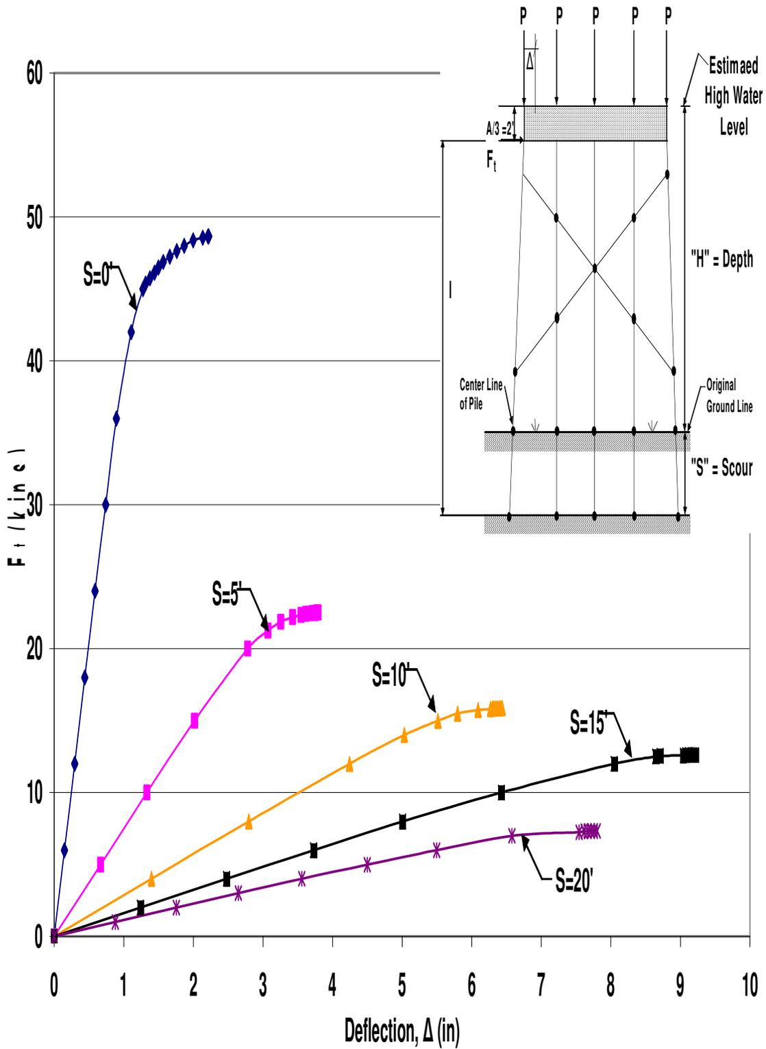
Figure A.63 HP10x42 X-Braced 5-Pile Bent with  $H=17'$ ,  $P=140$ kips and  $A=6'$
