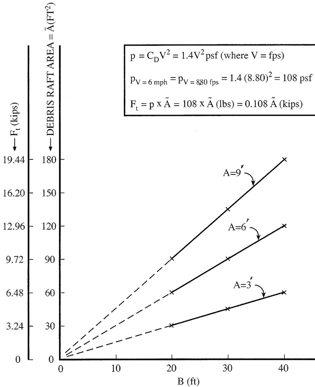
Figure 3.2 Bent  $F_t$  Force for Various Debris Raft Dimensions for  $V_{\text{Design}} = 6\text{mph}$
