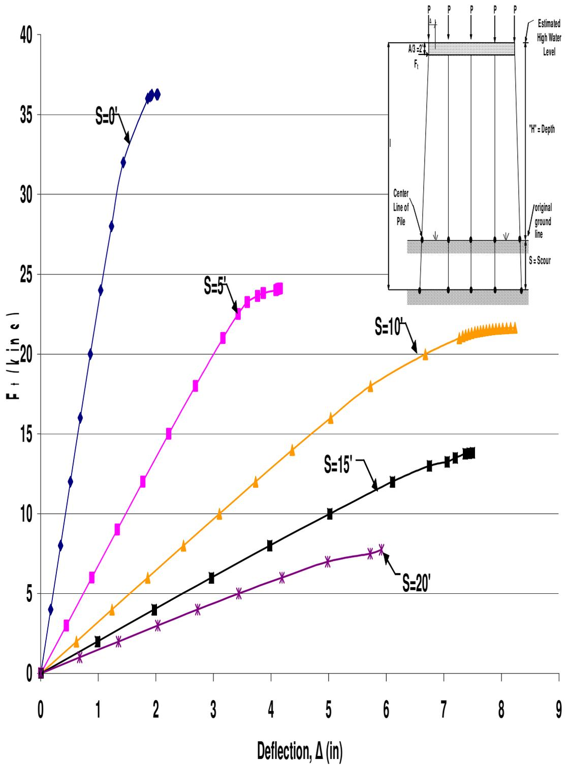
Figure A.52 HP10x42 Unbraced 5-Pile Bent with  $H=10'$ ,  $P=160$ kips and  $A=6'$
