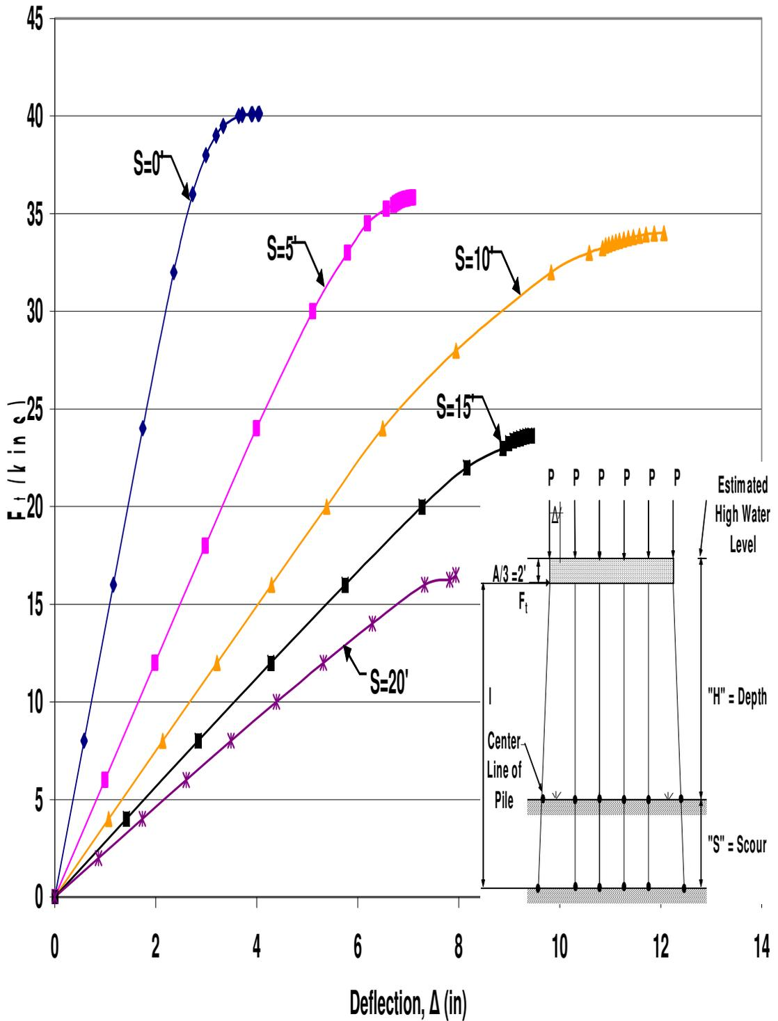
Figure A.77 HP10x42 Unbraced 6-Pile Bent with  $H=13'$ ,  $P=100$  kips and  $A=6'$
