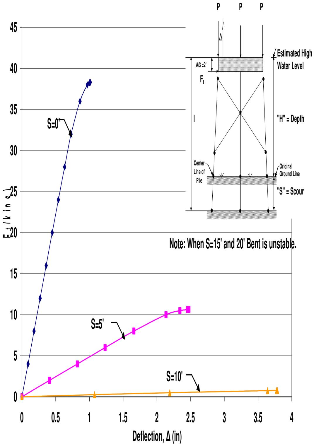
Figure A.15 HP10x42 X-Braced 3-Pile Bent with H=17', P=140kips and A=6'
