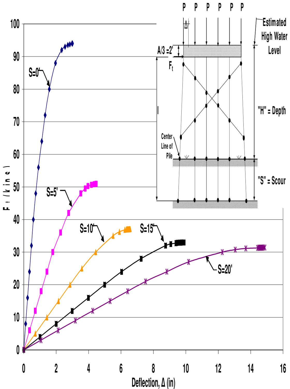
Figure B.83 HP12x53 Single X-Braced 6-Pile Bent with  $H=13'$ ,  $P=140$ kips and  $A=6'$
