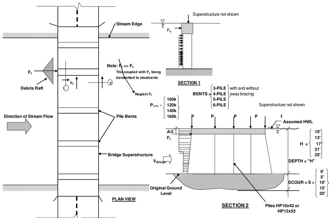
Figure 4.4 Typical Pile Bent Support Bridge Over Stream
