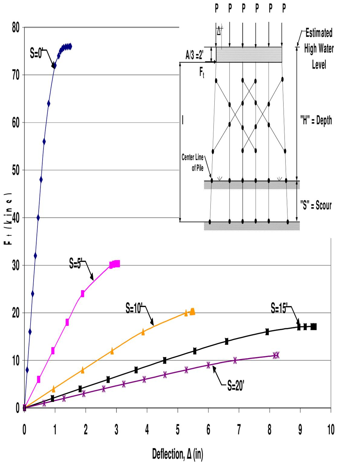
Figure A.91 HP10x42 Double X-Braced 6-Pile Bent with  $H=13'$ ,  $P=140$ kips and  $A=6'$
