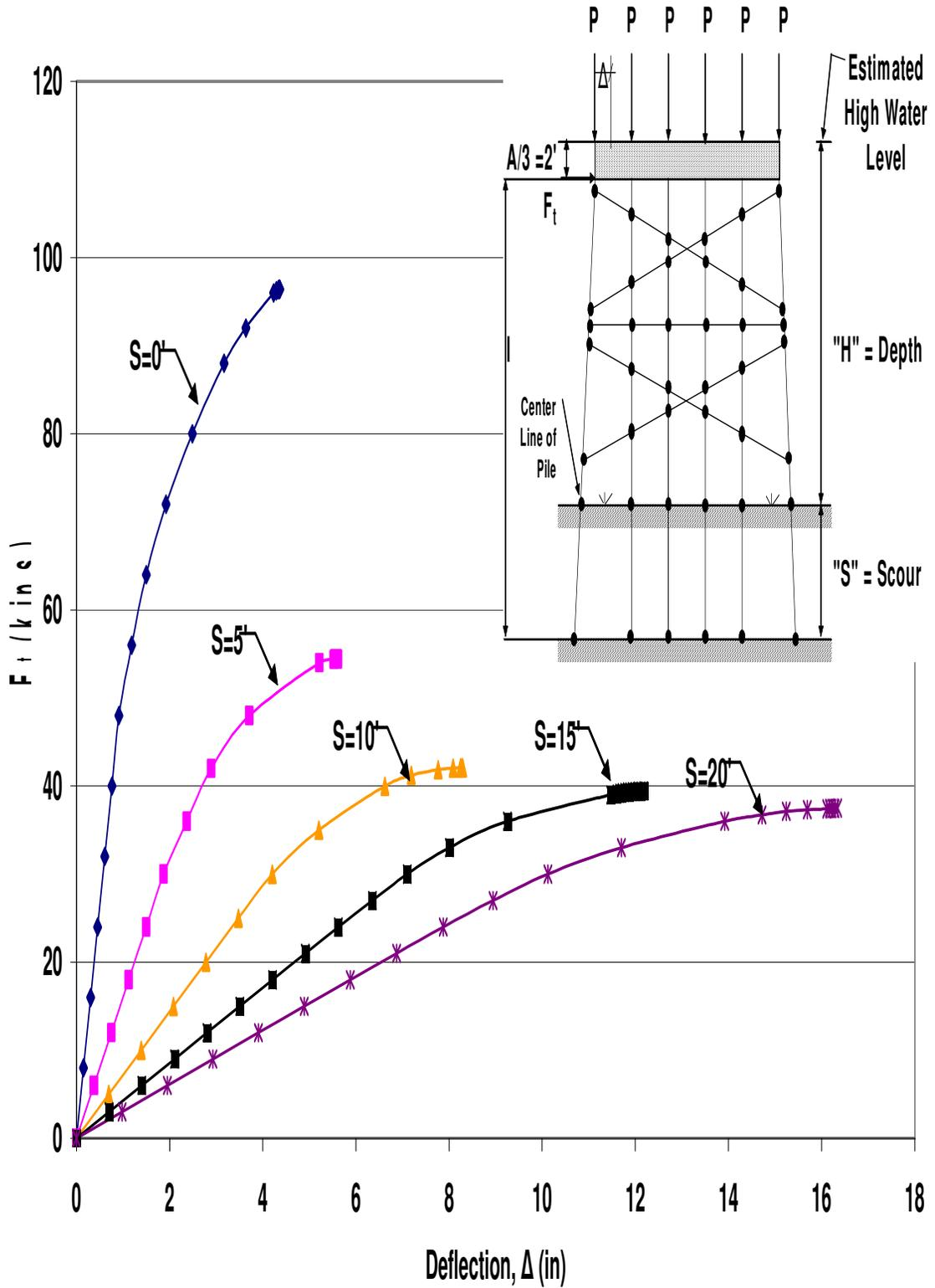
Figure B.101 HP12x53 Two-Story Single X-Braced 6-Pile Bent with  $H=25'$ ,  $P=100$ kips and  $A=6'$  Pushover Analysis Results
