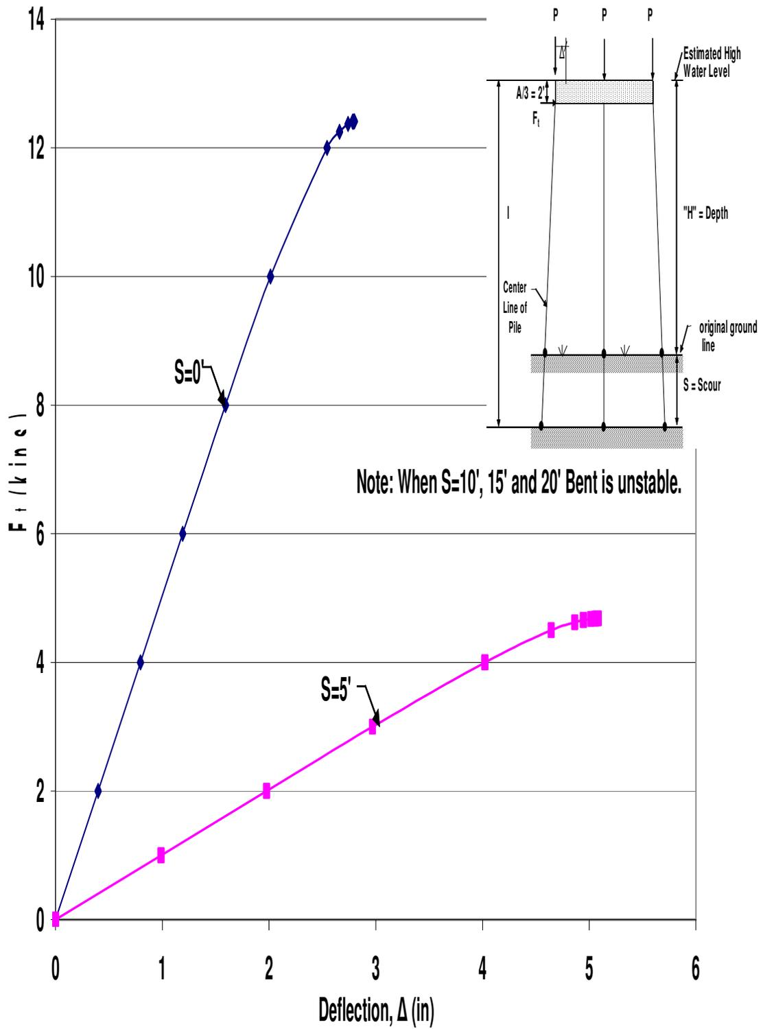
Figure A.6 HP10x42 Unbraced 3-Pile Bent with H=13', P=120kips, and A=6'
