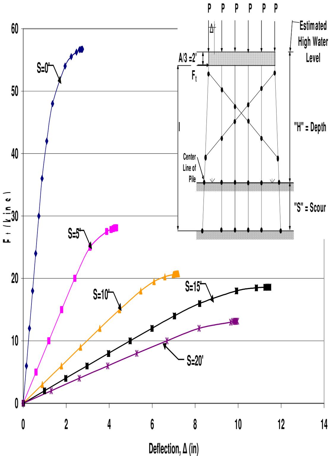
Figure A.86 HP10x42 Single X-Braced 6-Pile Bent with  $H=17'$ ,  $P=120$ kips and  $A=6'$
