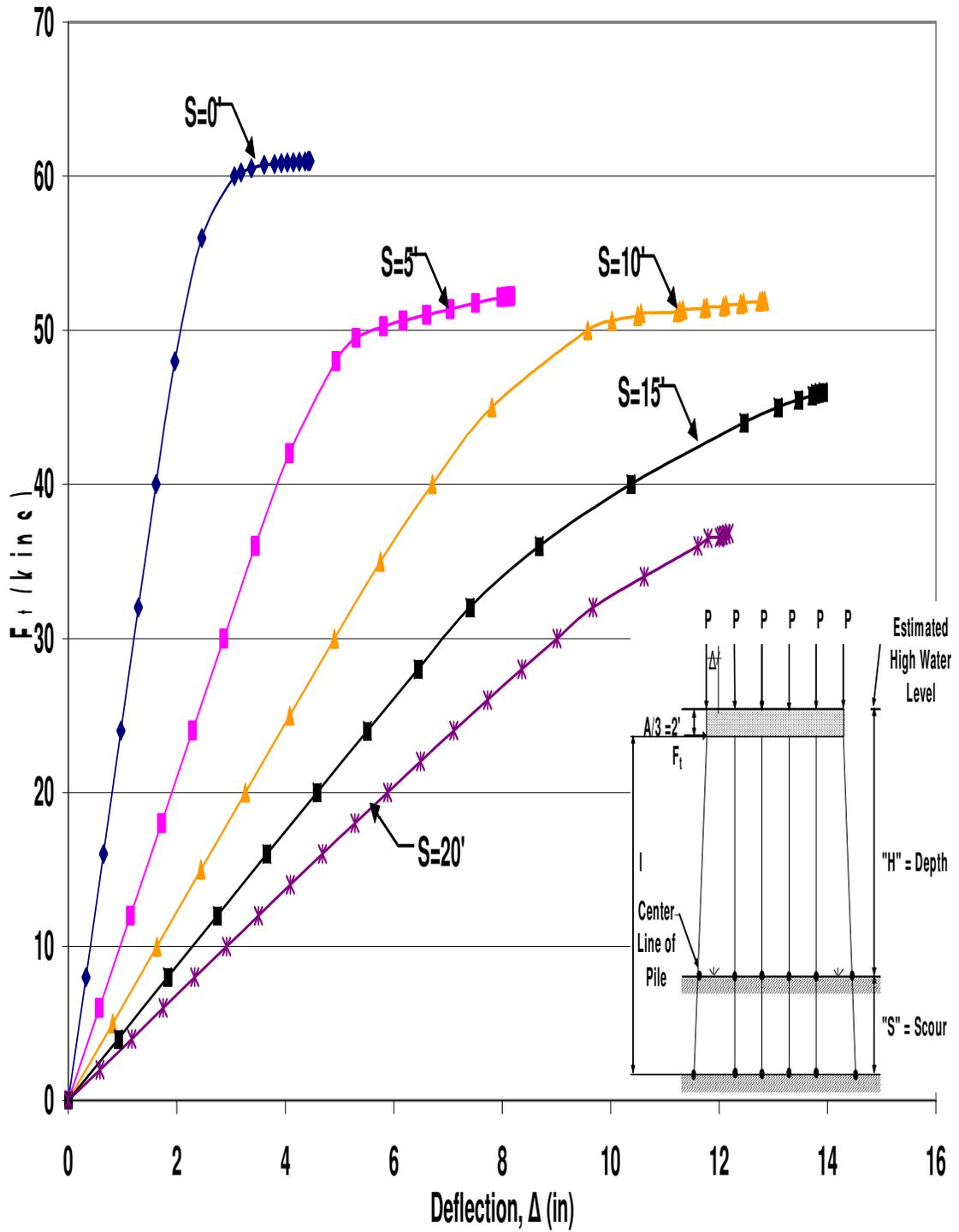
Figure B.77 HP12x53 Unbraced 6-Pile Bent with  $H=13'$ ,  $P=100$ kips and  $A=6'$
