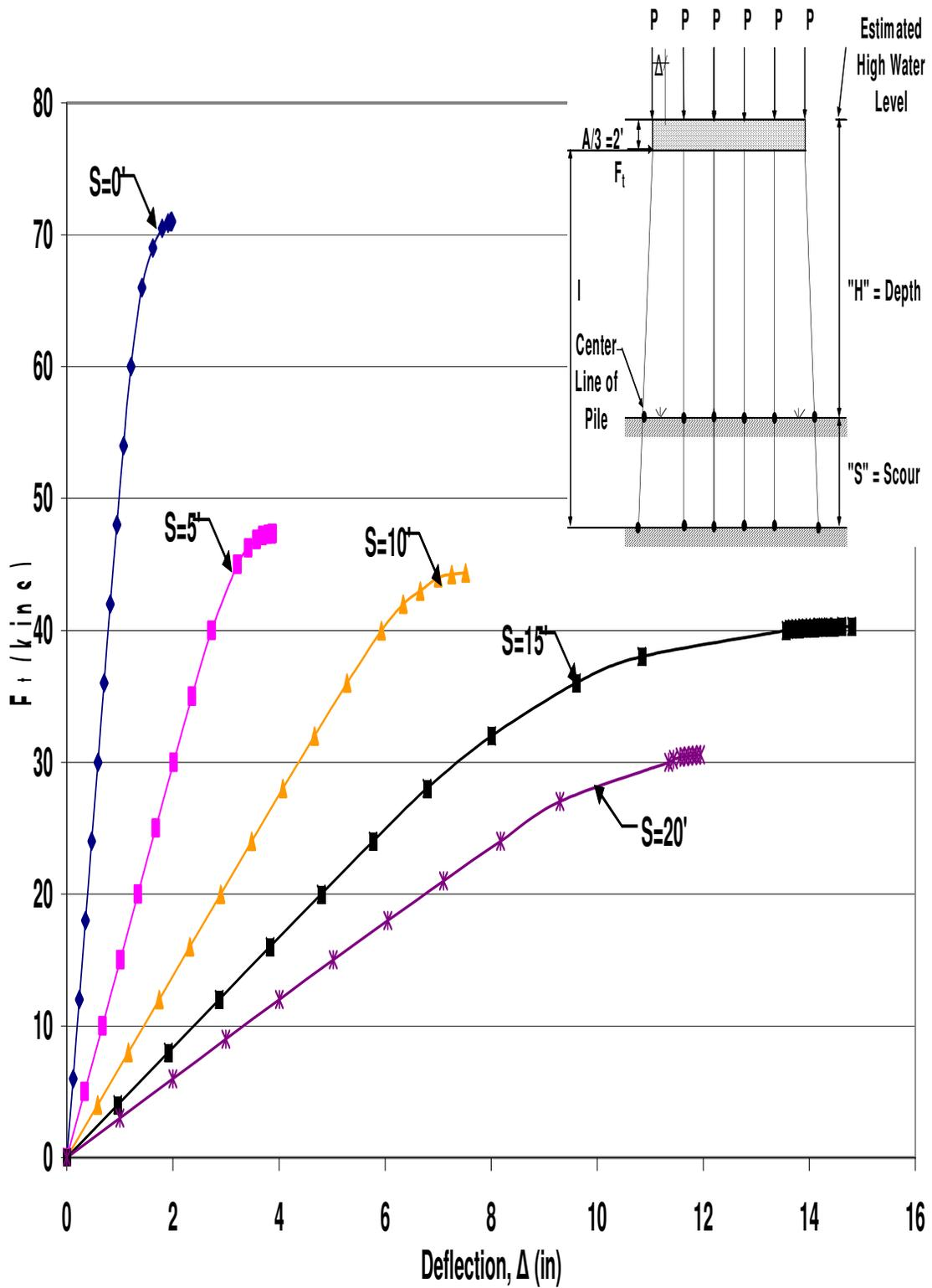
Figure B.75 HP12x53 Unbraced 6-Pile Bent with  $H=10'$ ,  $P=140$ kips and  $A=6'$
