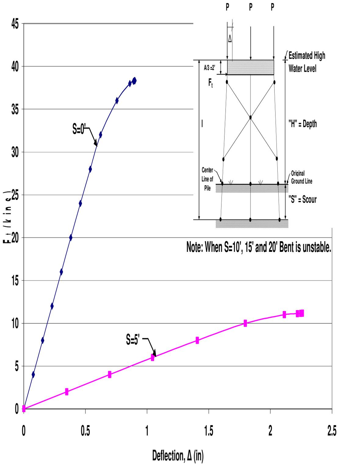
Figure A.12 HP10x42 X-Braced 3-Pile Bent with H=13', P=160kips and A=6'
