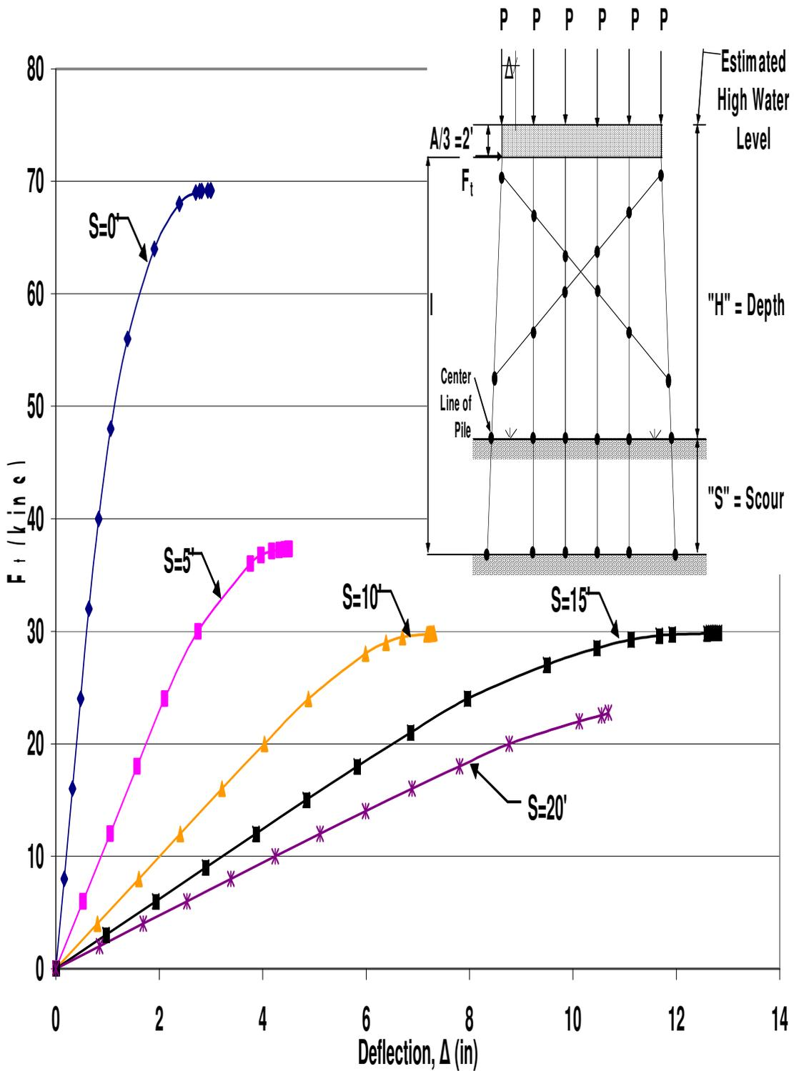
Figure A.81 HP10x42 Single X-Braced 6-Pile Bent with  $H=13'$ ,  $P=100$  kips and  $A=6'$
