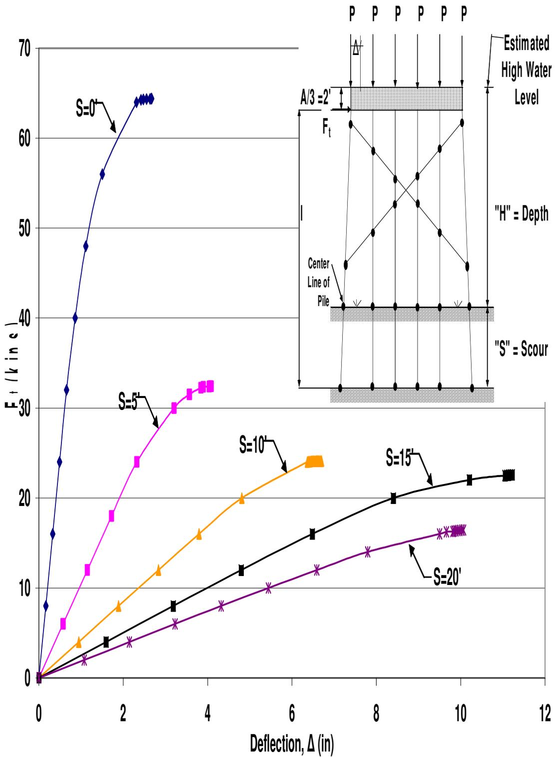
Figure A.82 HP10x42 Single X-Braced 6-Pile Bent with  $H=13'$ ,  $P=120$ kips and  $A=6'$
