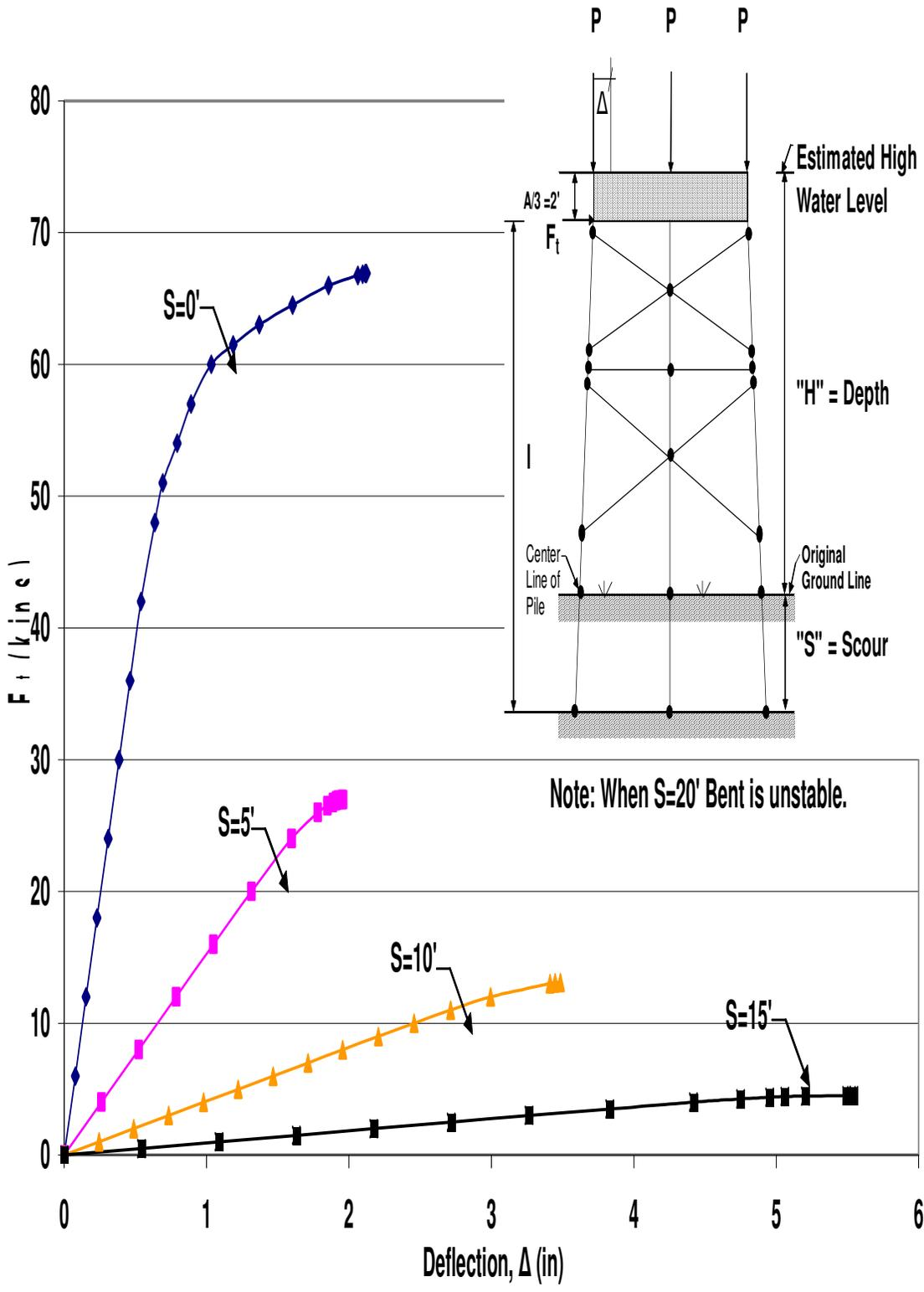
Figure B.19 HP12x53 Two-Story X-Braced 3-Pile Bent with H=21', P=140kips and A=6'
