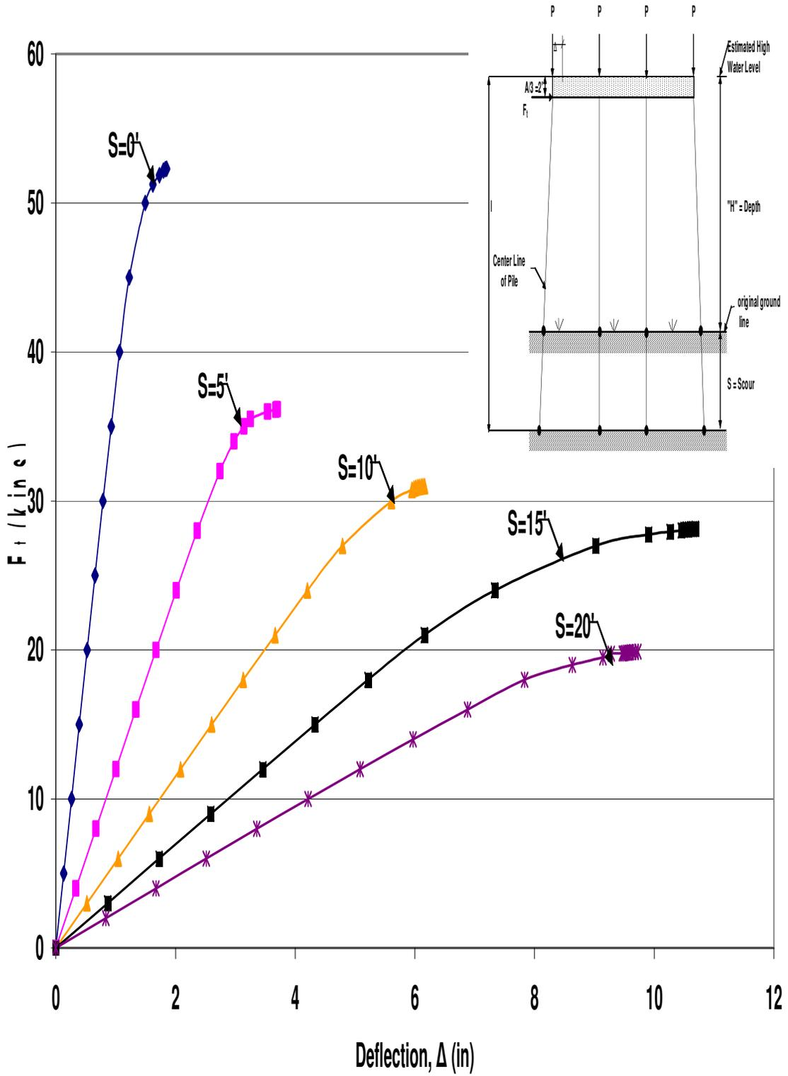
Figure B.27 HP12x53 Unbraced 4-Pile Bent with  $H=10'$ ,  $P=140$ kips and  $A=6'$
