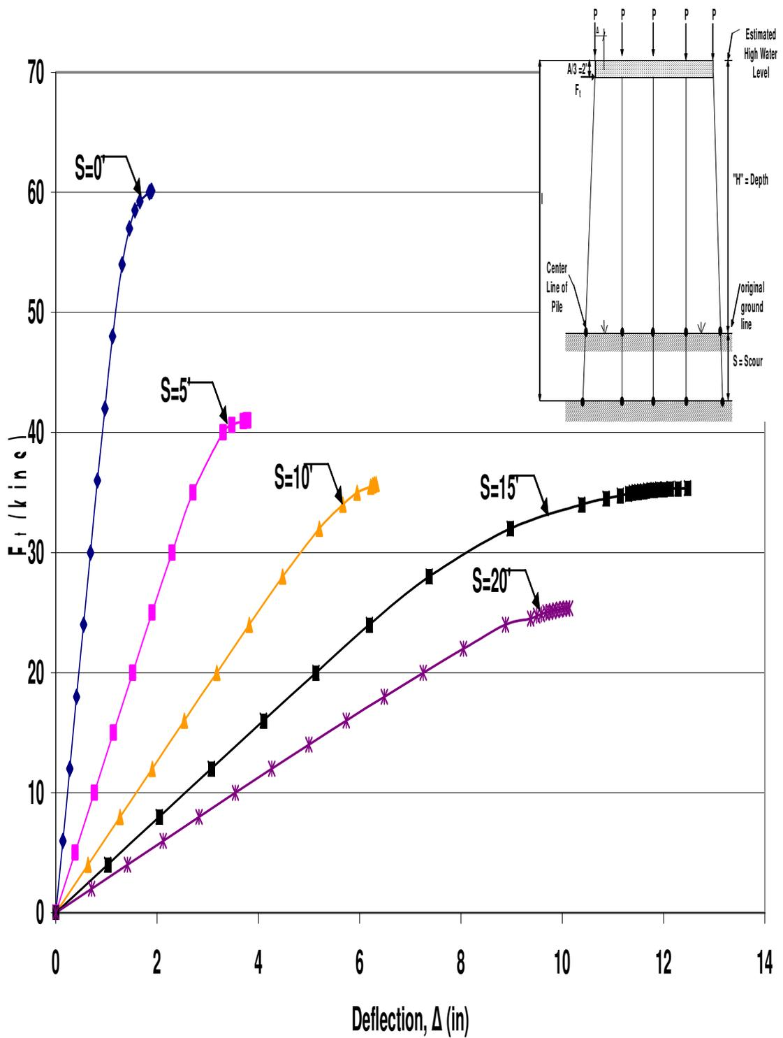
Figure B.52 HP12x53 Unbraced 5-Pile Bent with  $H=10'$ ,  $P=160$ kips and  $A=6'$
