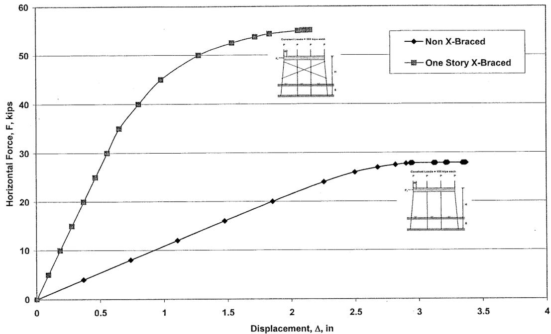
Figure 4.7 GTSTRUDL Pushover Analysis Results for HP10x42 4 Pile Bents, Bents Pinned at Ground, H=13ft, S=0ft
