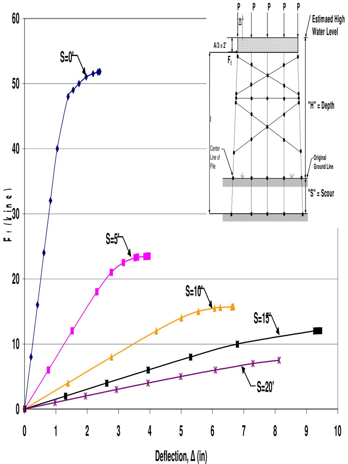
Figure A.70 HP10x42 Two-Story X-Braced 5-Pile Bent with  $H=25'$ ,  $P=120$ kips and  $A=6'$
