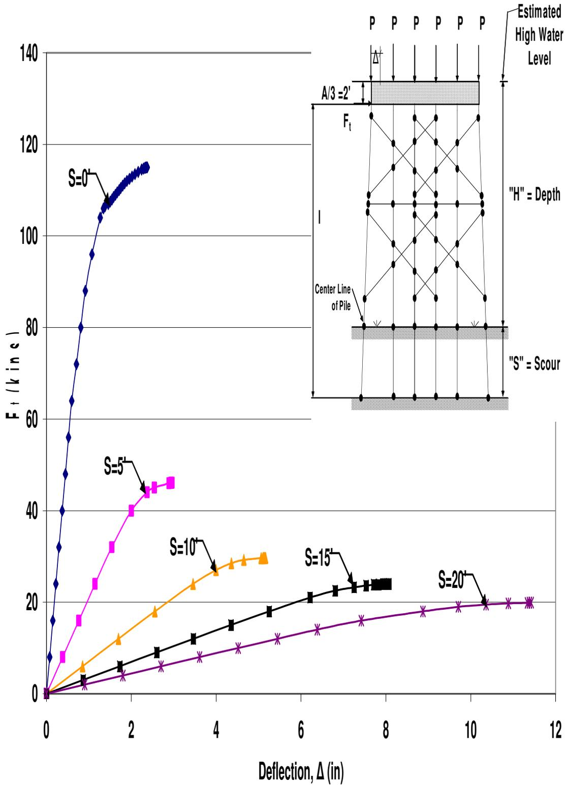
Figure B.112 HP12x53 Two-Story Double X-Braced 6-Pile Bent with  $H=25'$ ,  $P=160$ kips and  $A=6'$  Pushover Analysis Results
