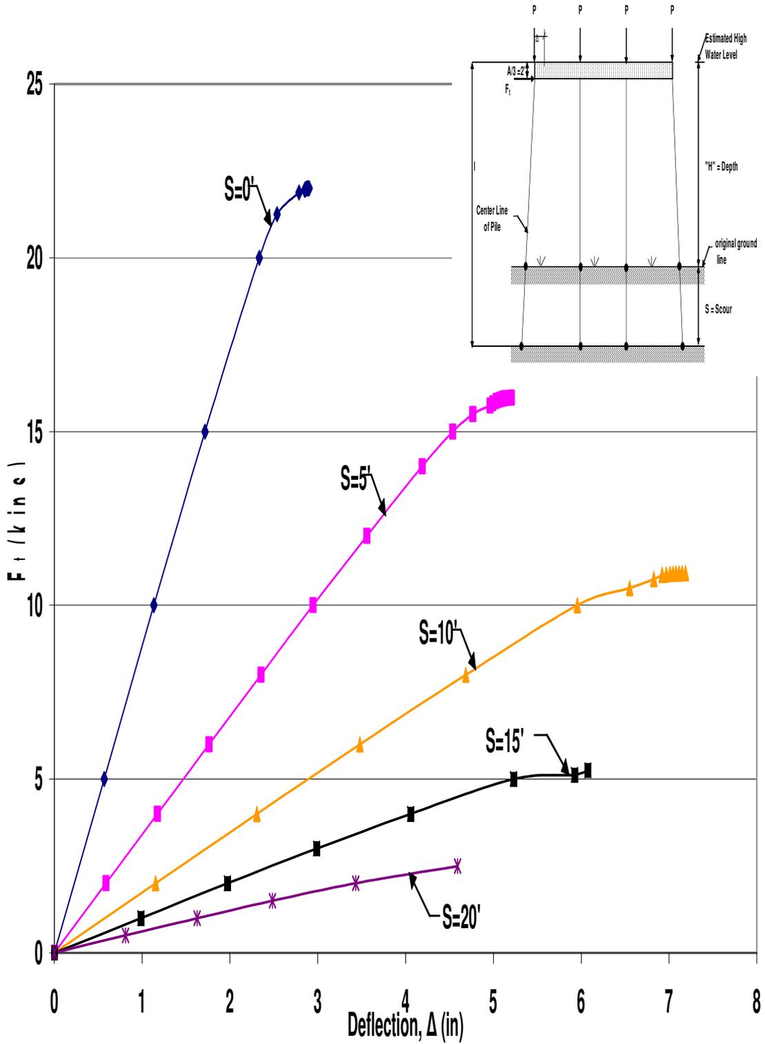
Figure A.32 Unbraced 4-Pile Bent with H=13', P=160kips and A=6'
