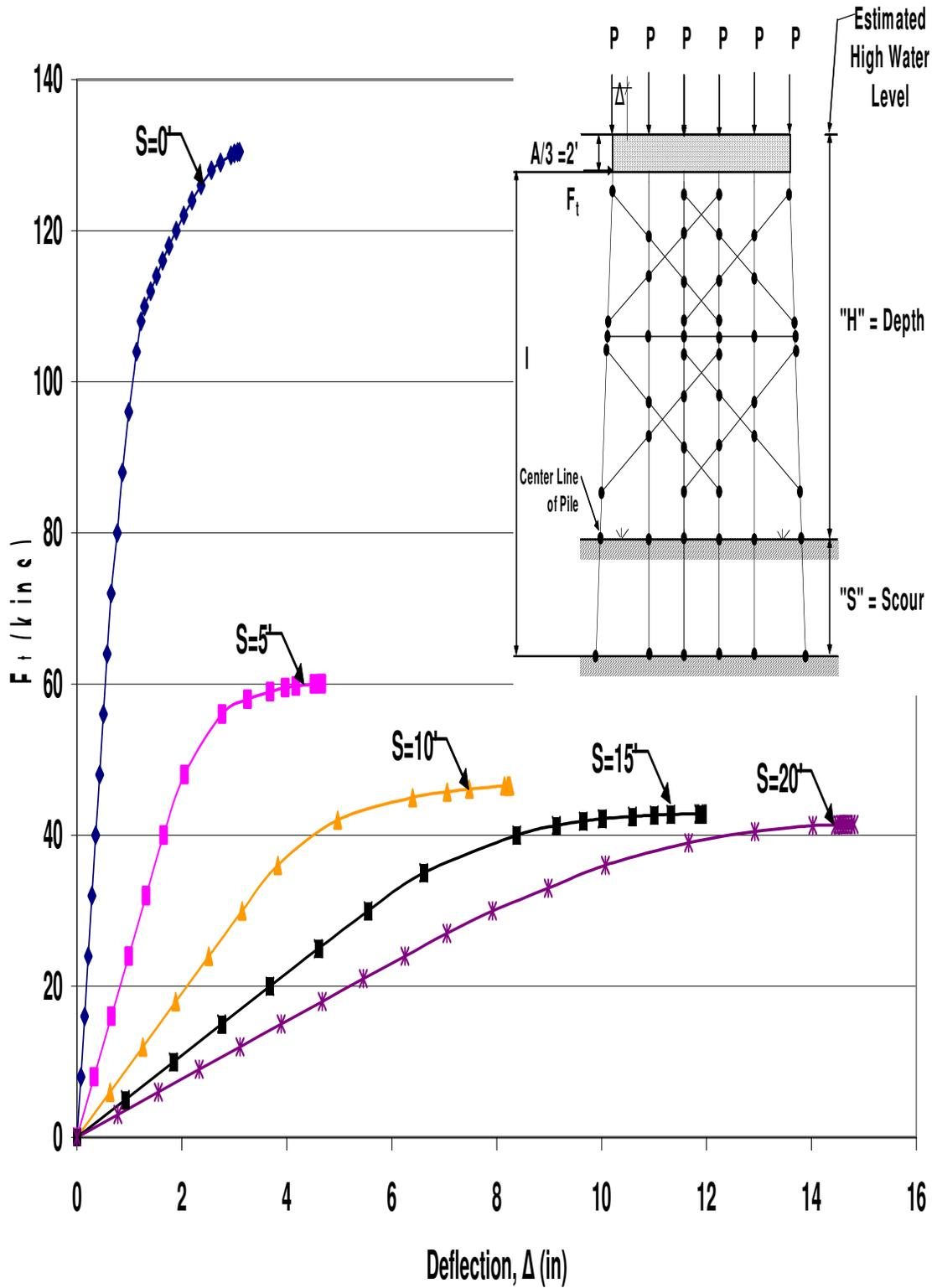
Figure B.109 HP12x53 Two-Story Double X-Braced 6-Pile Bent with  $H=25'$ ,  $P=100$ kips and  $A=6'$  Pushover Analysis Results
