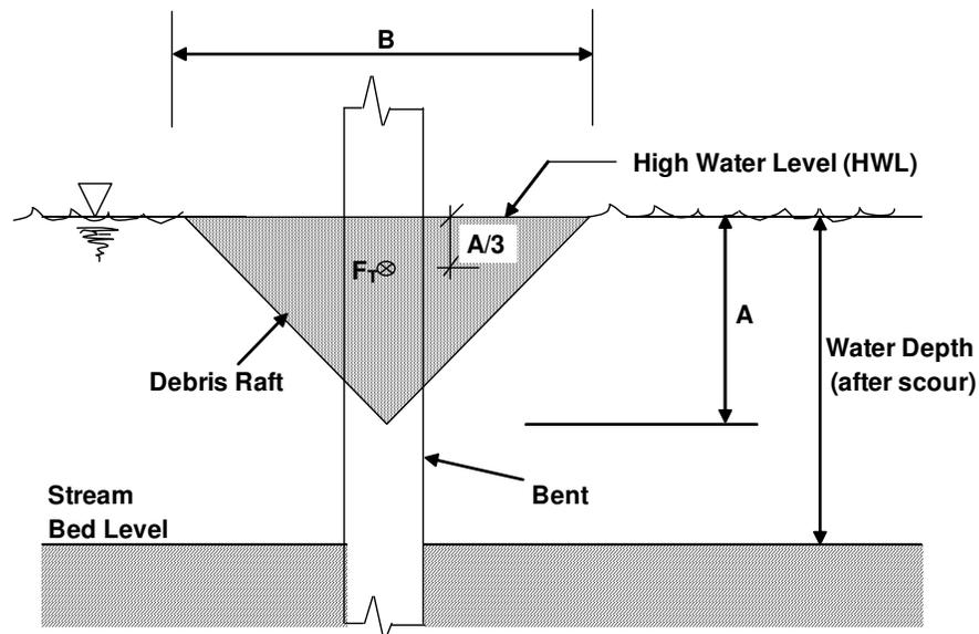
Figure 3.1 Debris Raft for Pier Design (AASHTO 1997)
