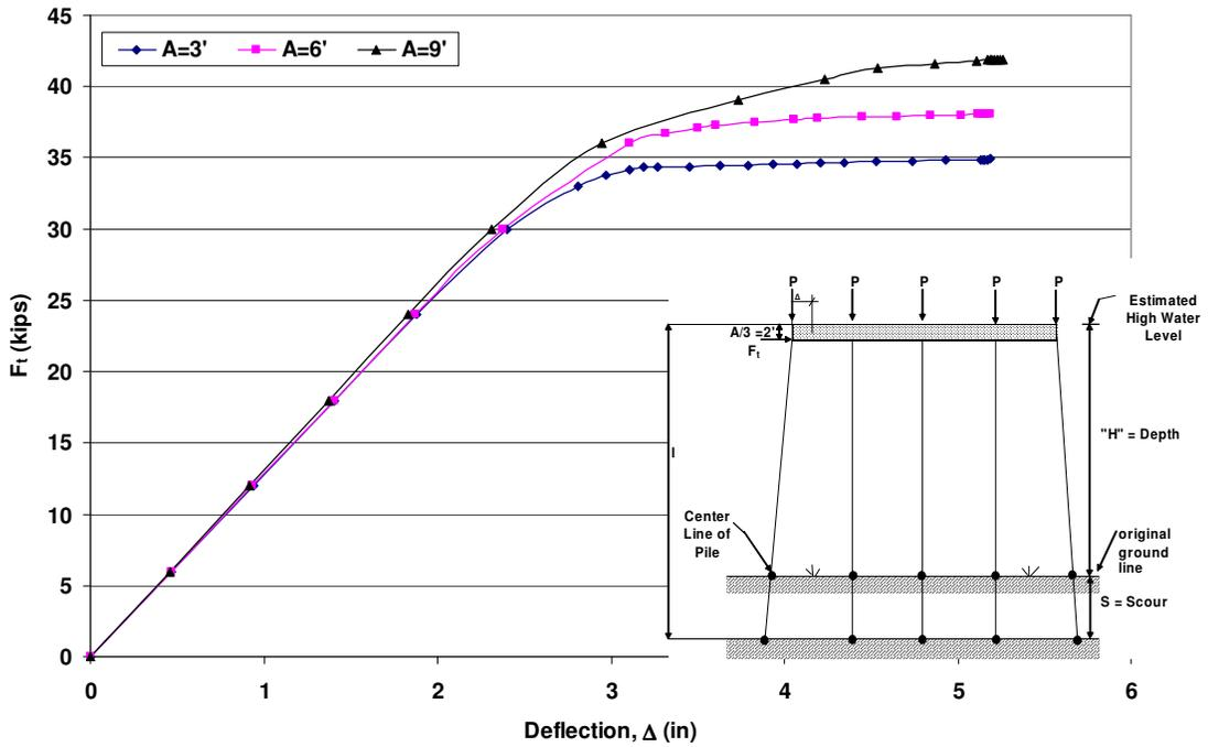
Figure 3.3 HP10x42 Unbraced 5-Pile Bent with  $H=13'$ ,  $S=0'$ , and  $P=100$ kips Pushover Analysis Results
