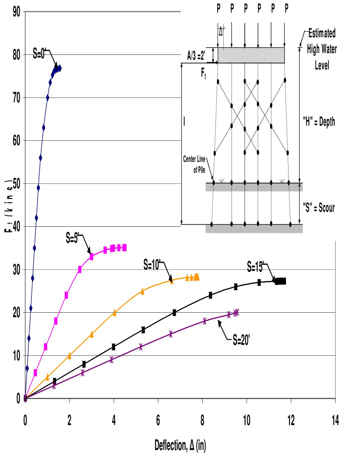
Figure A.93 HP10x42 Double X-Braced 6-Pile Bent with  $H=17'$ ,  $P=100$ kips and  $A=6'$
