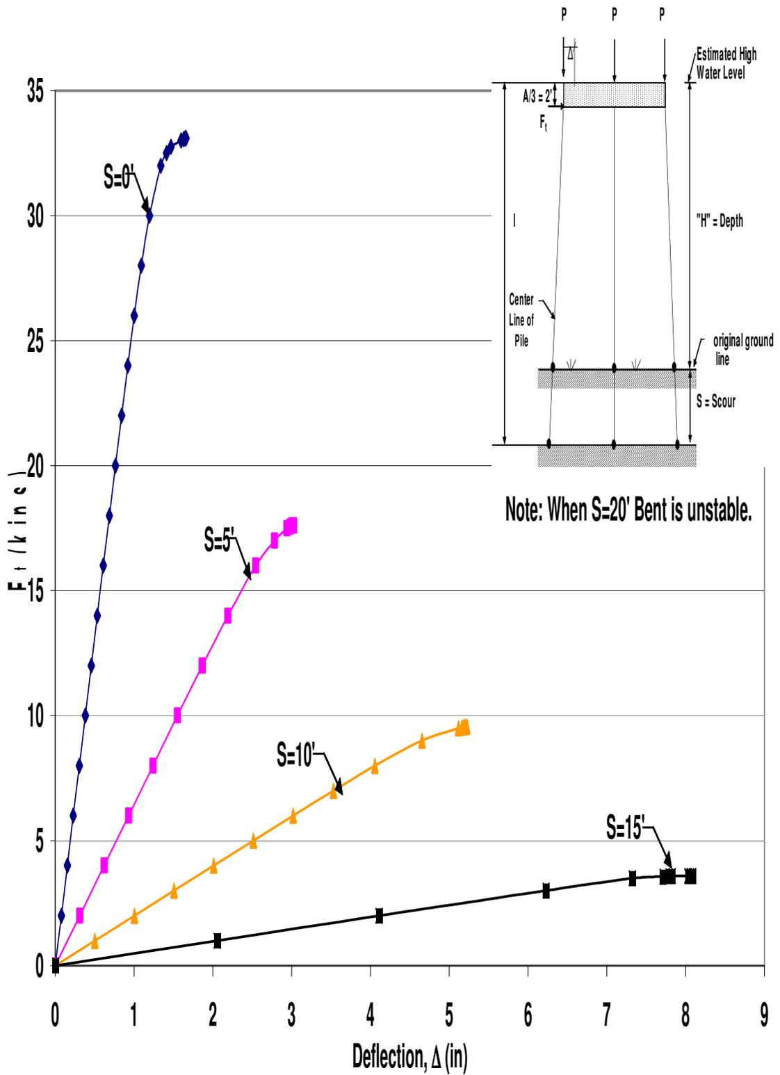
Figure B.3 HP12x53 Unbraced 3-Pile Bent with  $H=10'$ ,  $P=140$ kips and  $A=6'$
