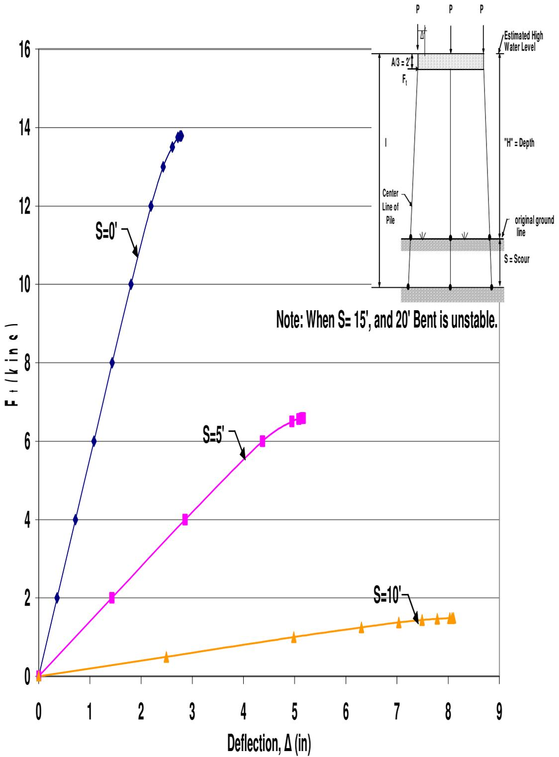
Figure A.5 HP10x42 Unbraced 3-Pile Bent with  $H=13'$ ,  $P=100$ kips, and  $A=6'$
