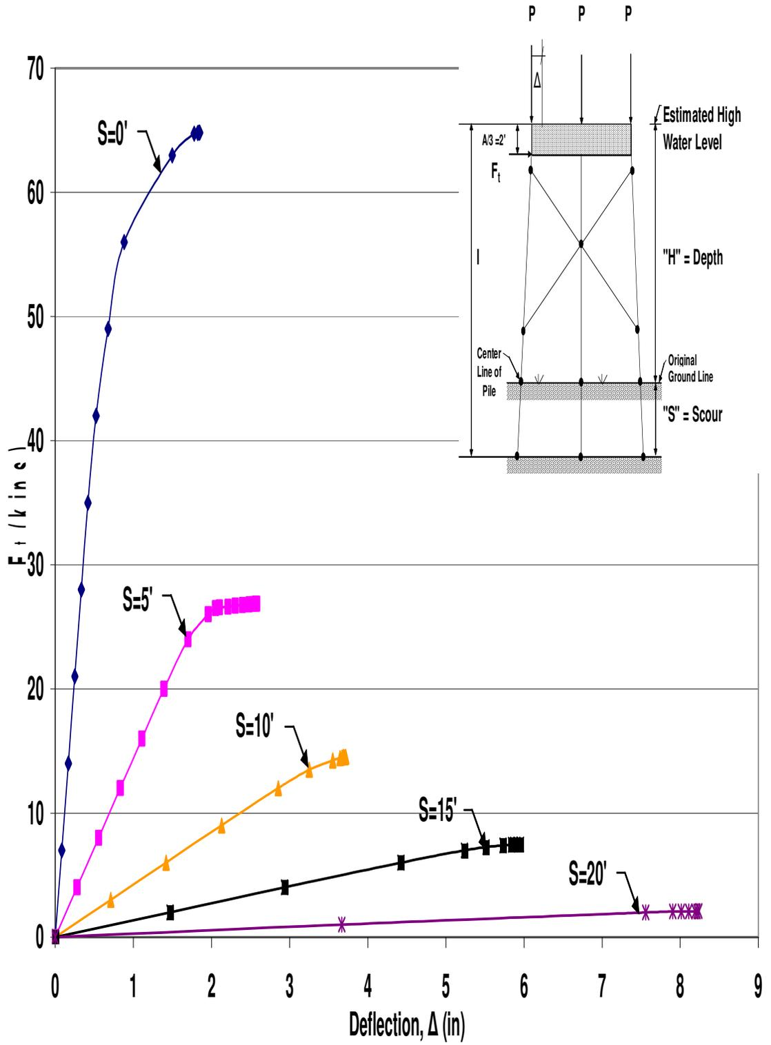
Figure B.10 HP12x53 X-Braced 3-Pile Bent with  $H=13'$ ,  $P=120$ kips and  $A=6'$
