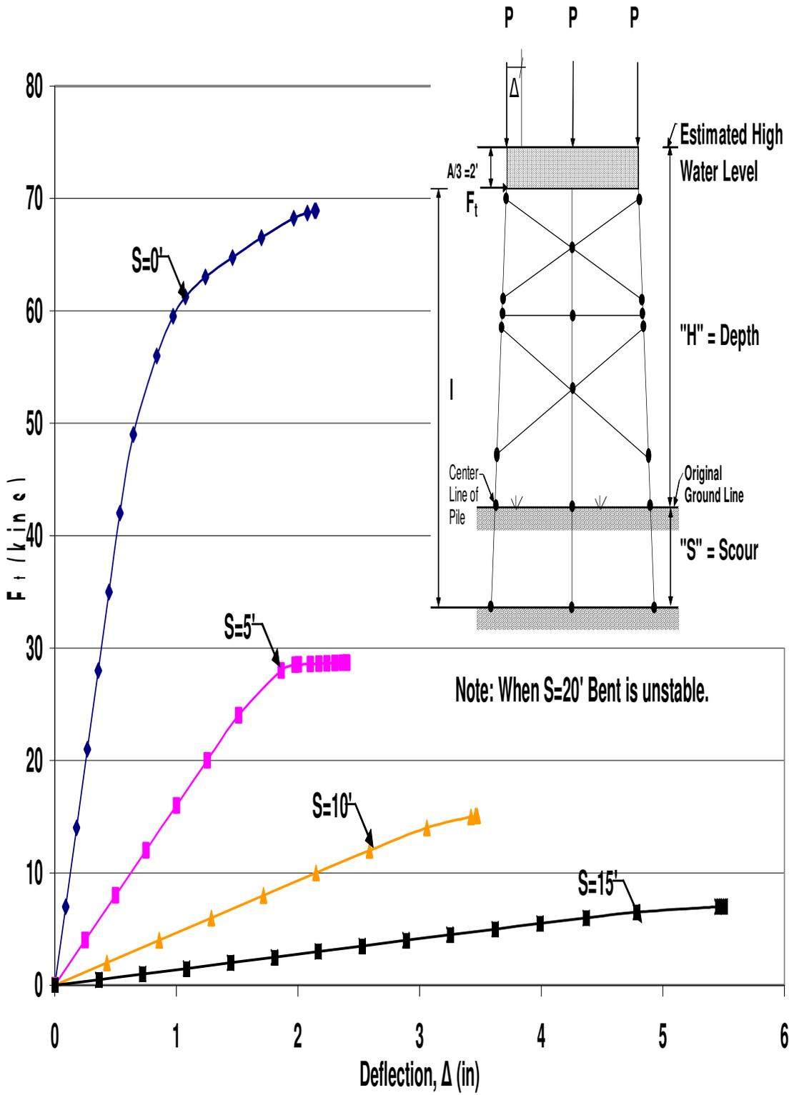
Figure B.18 HP12x53 Two-Story X-Braced 3-Pile Bent with  $H=21'$ ,  $P=120$ kips and  $A=6'$
