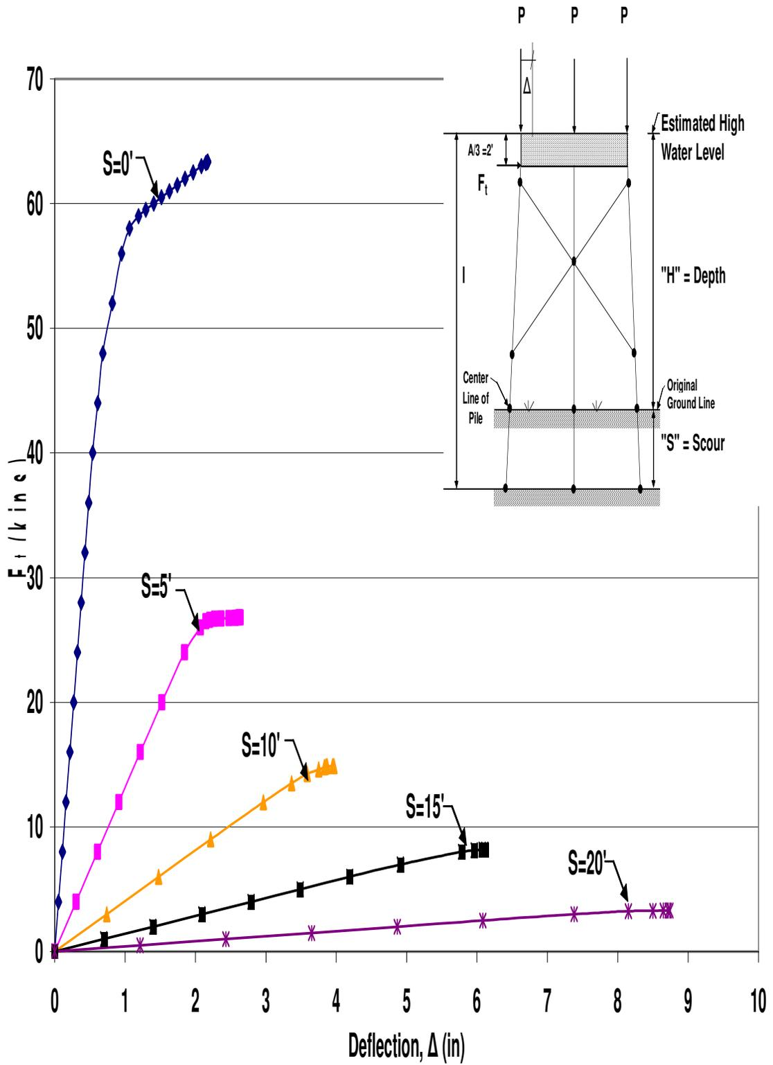
Figure B.13 HP12x53 X-Braced 3-Pile Bent with  $H=17'$ ,  $P=100$  kips and  $A=6'$
