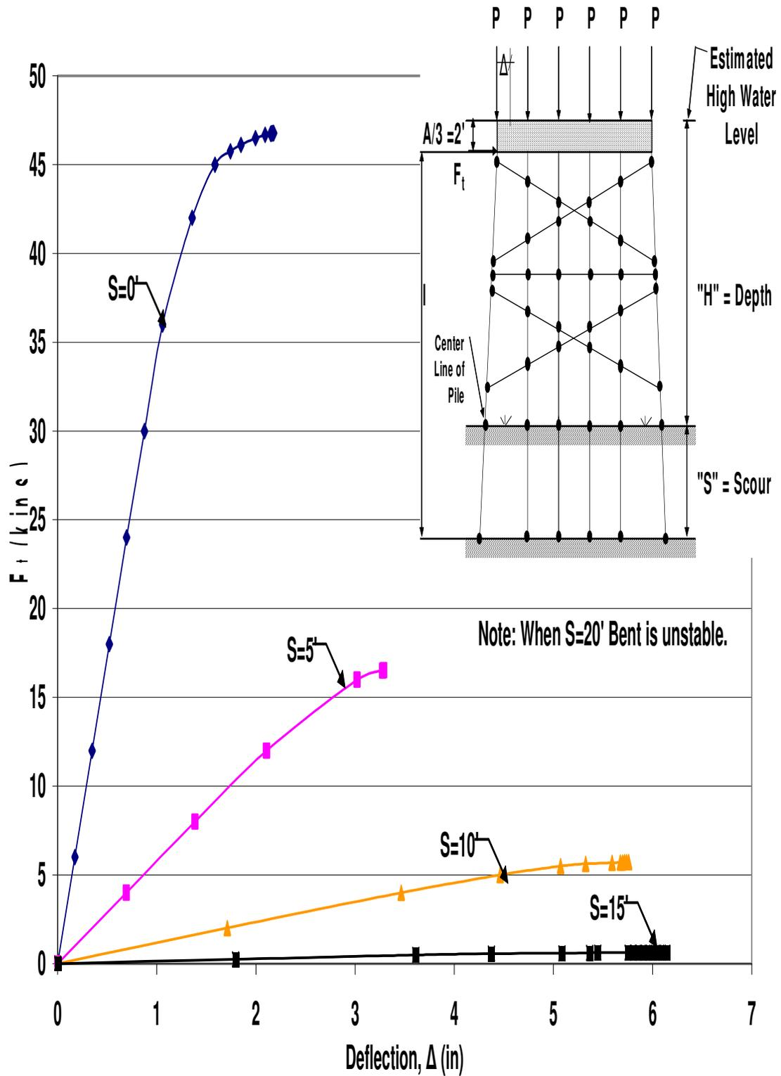
Figure A.104 HP10x42 Two-Story Single X-Braced 6-Pile Bent with  $H=25'$ ,  $P=160$ kips and  $A=6'$  Pushover Analysis Results
