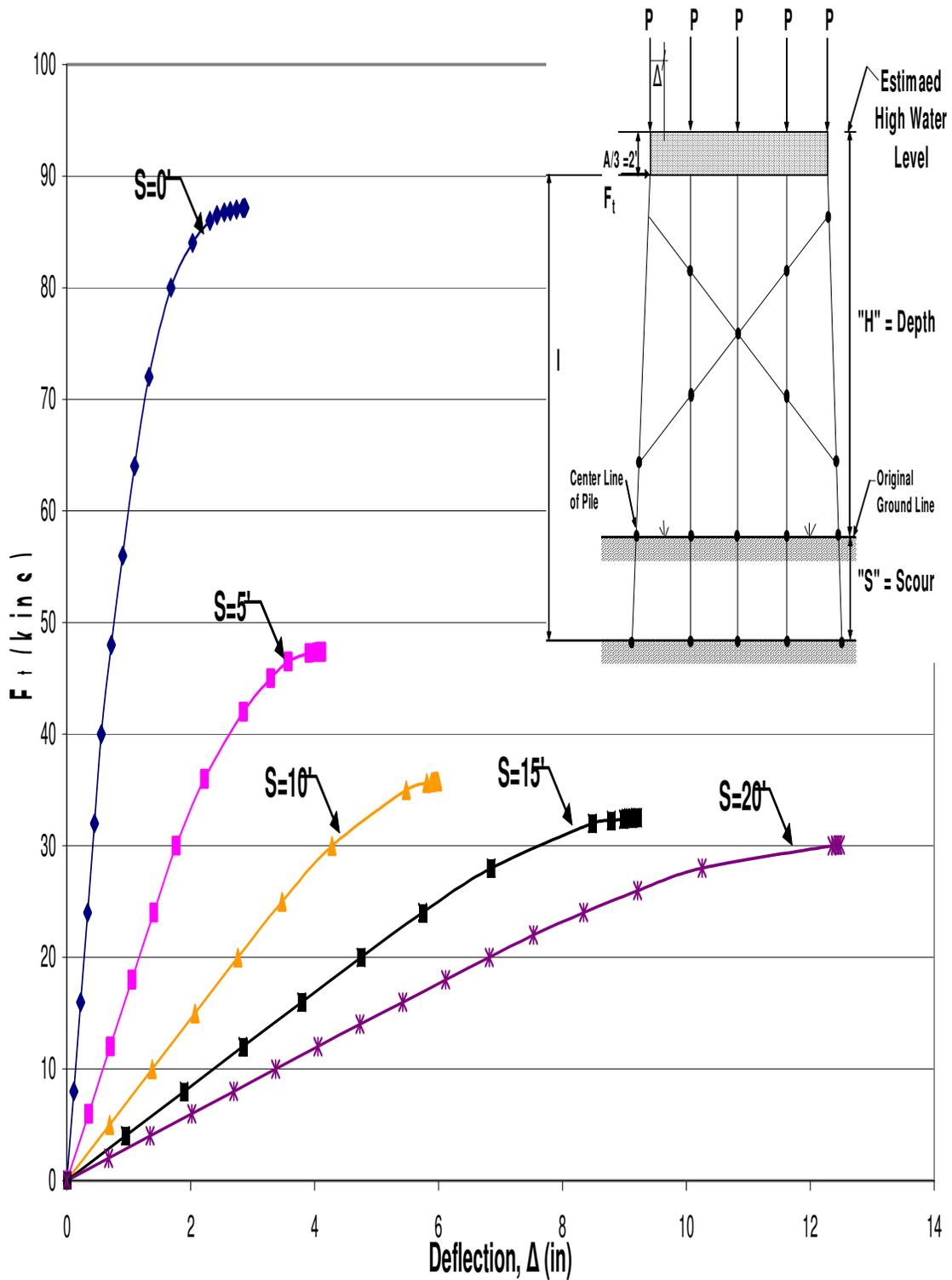
Figure B.59 HP12x53 X-Braced 5-Pile Bent with  $H=13'$ ,  $P=140$ kips and  $A=6'$
