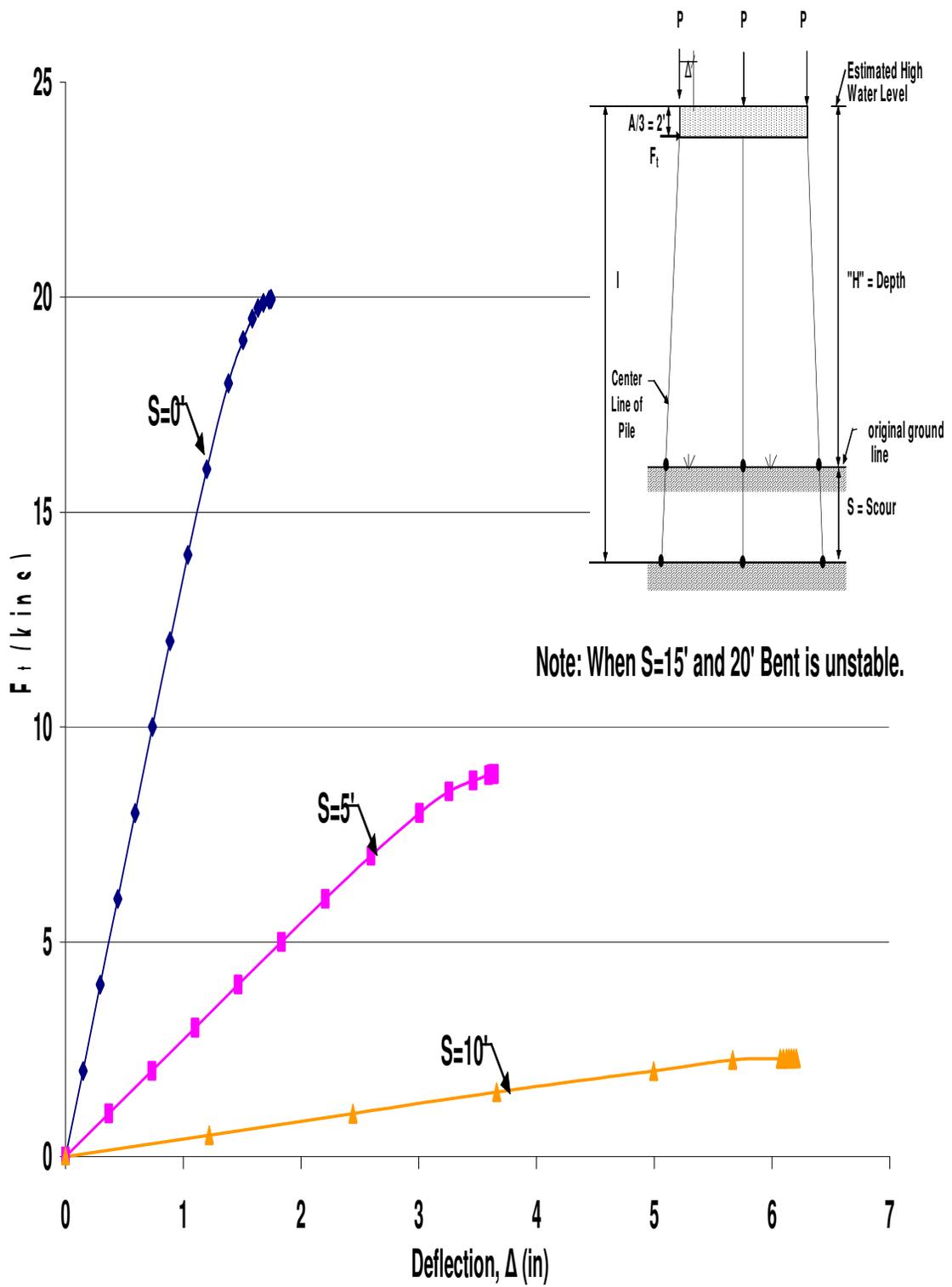
Figure A.2 HP10x42 Unbraced 3-Pile Bent with H=10', P=120kips, and A=6'
