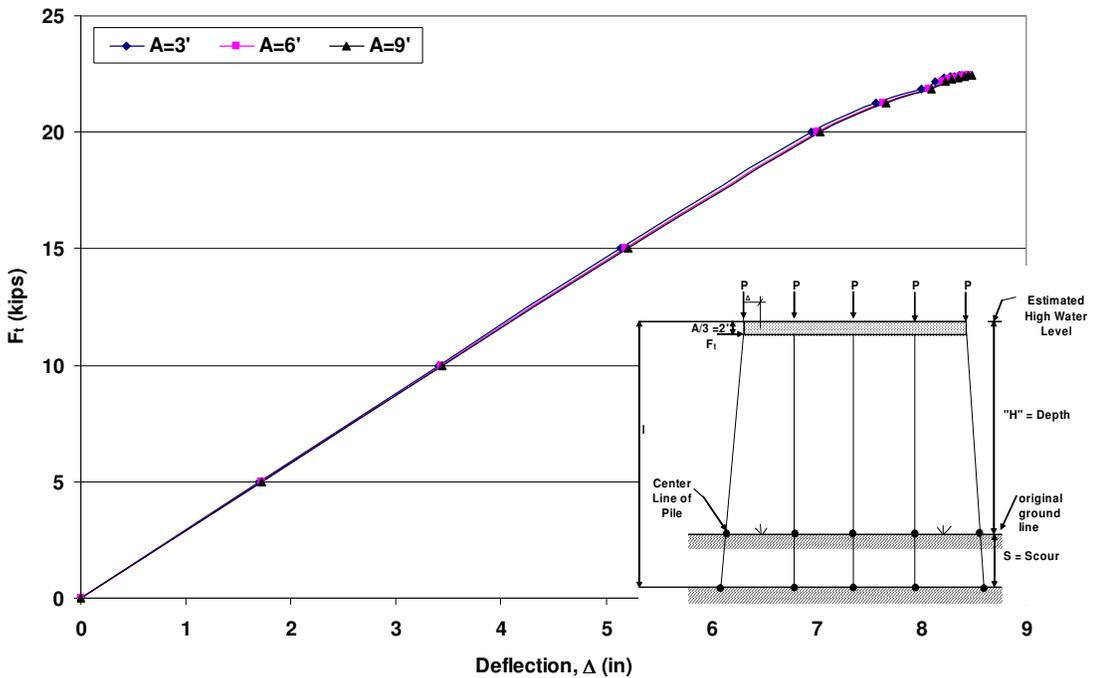
Figure 3.4 HP10x42 Unbraced 5-Pile Bent with  $H=13'$ ,  $S=15'$ , and  $P=100$ kips Pushover Analysis Results
