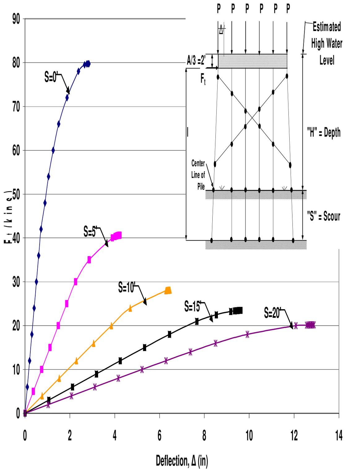
Figure B.88 HP12x53 Single X-Braced 6-Pile Bent with  $H=17'$ ,  $P=160$ kips and  $A=6'$
