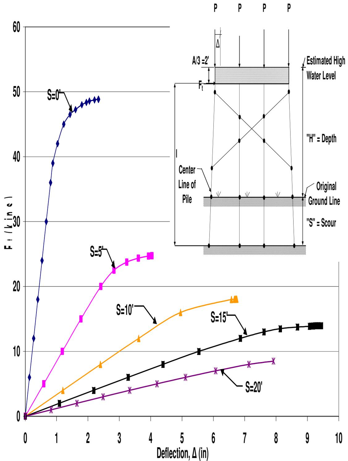
Figure A.37 HP10x42 X-Braced 4-Pile Bent with  $H=17'$ ,  $P=100$ kips and  $A=6'$
