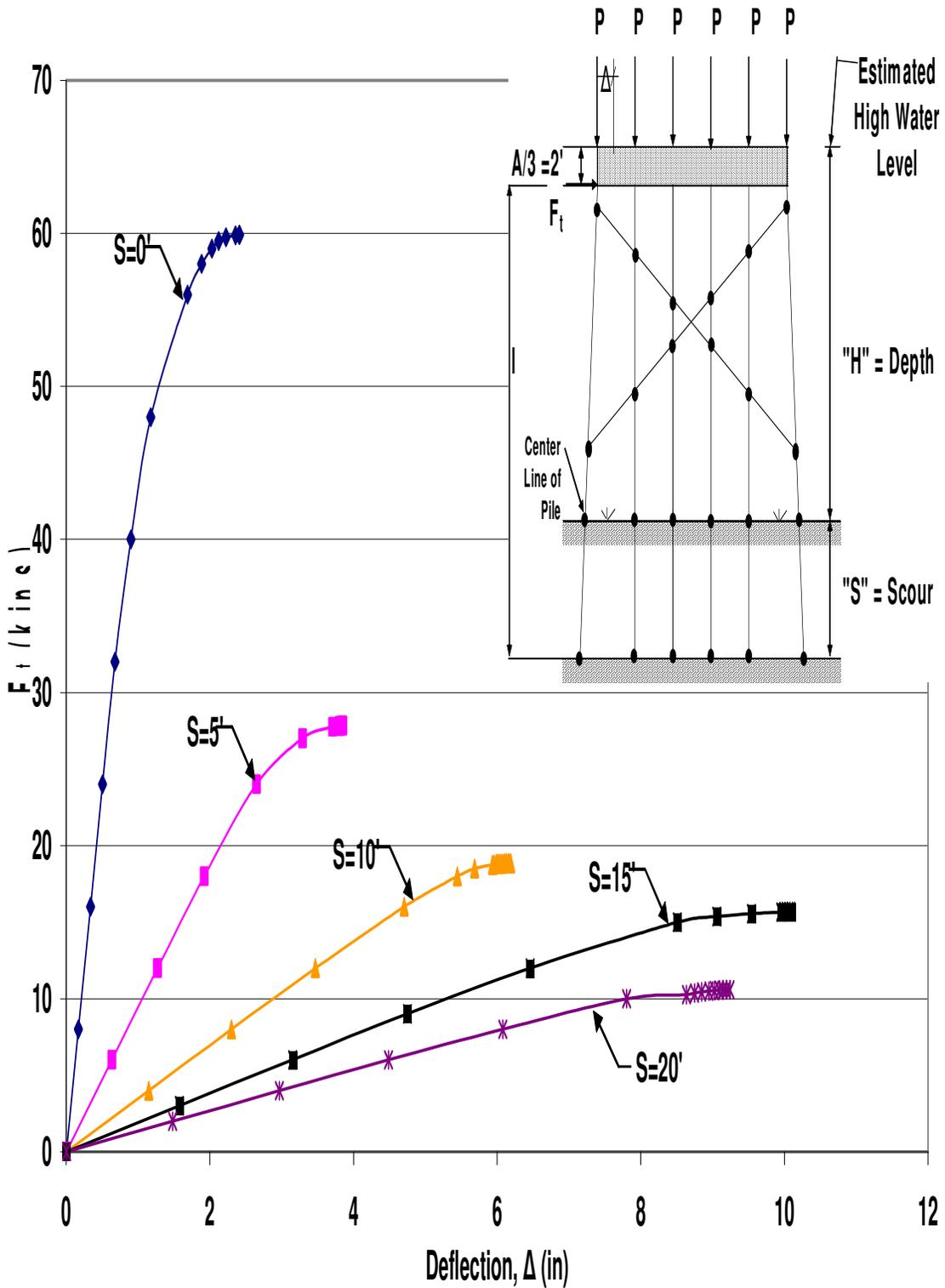
Figure A.83 HP10x42 Single X-Braced 6-Pile Bent with  $H=13'$ ,  $P=140$  kips and  $A=6'$
