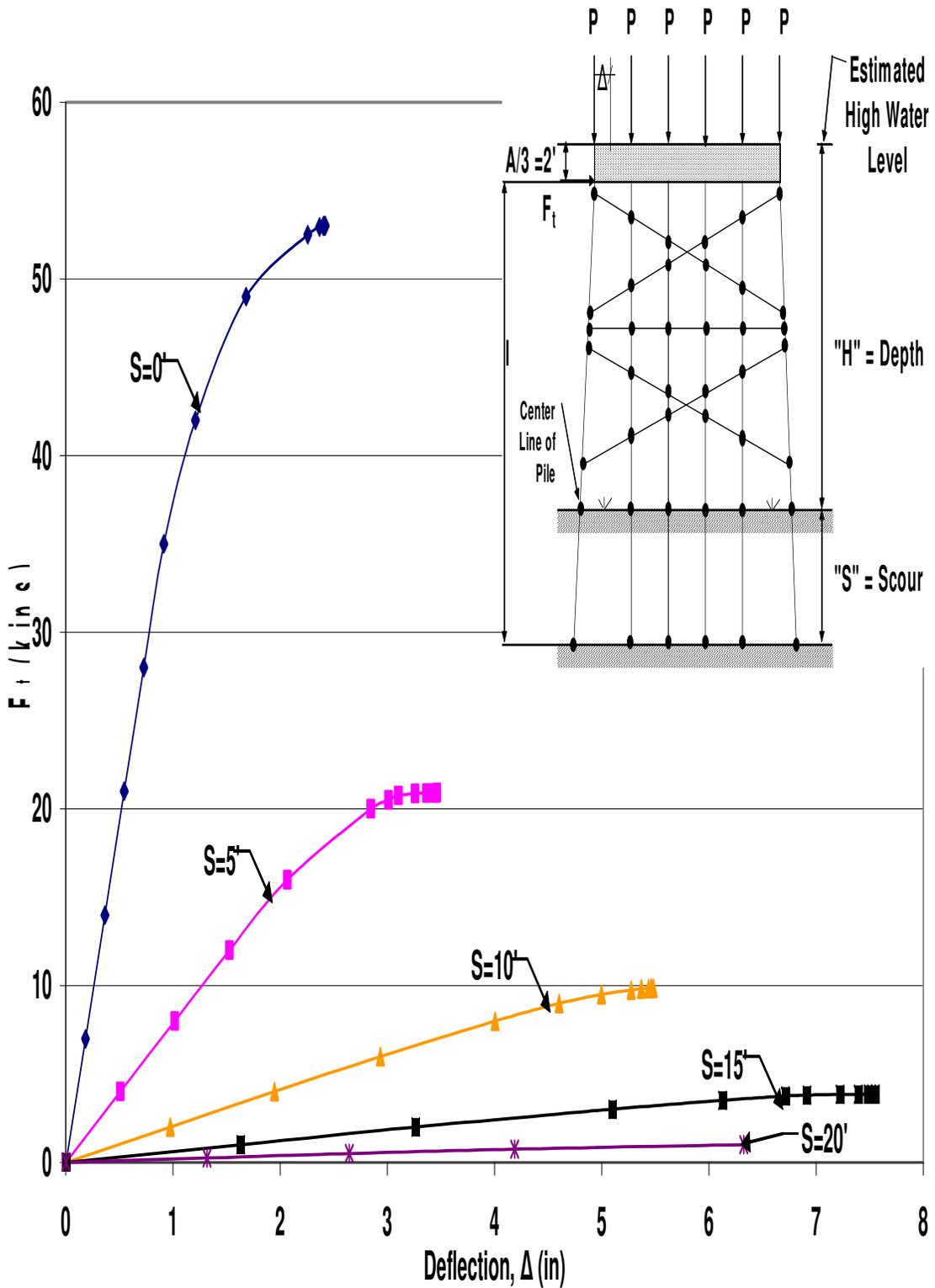
Figure A.100 HP10x42 Two-Story Single X-Braced 6-Pile Bent with  $H=21'$ ,  $P=160$ kips and  $A=6'$  Pushover Analysis Results
