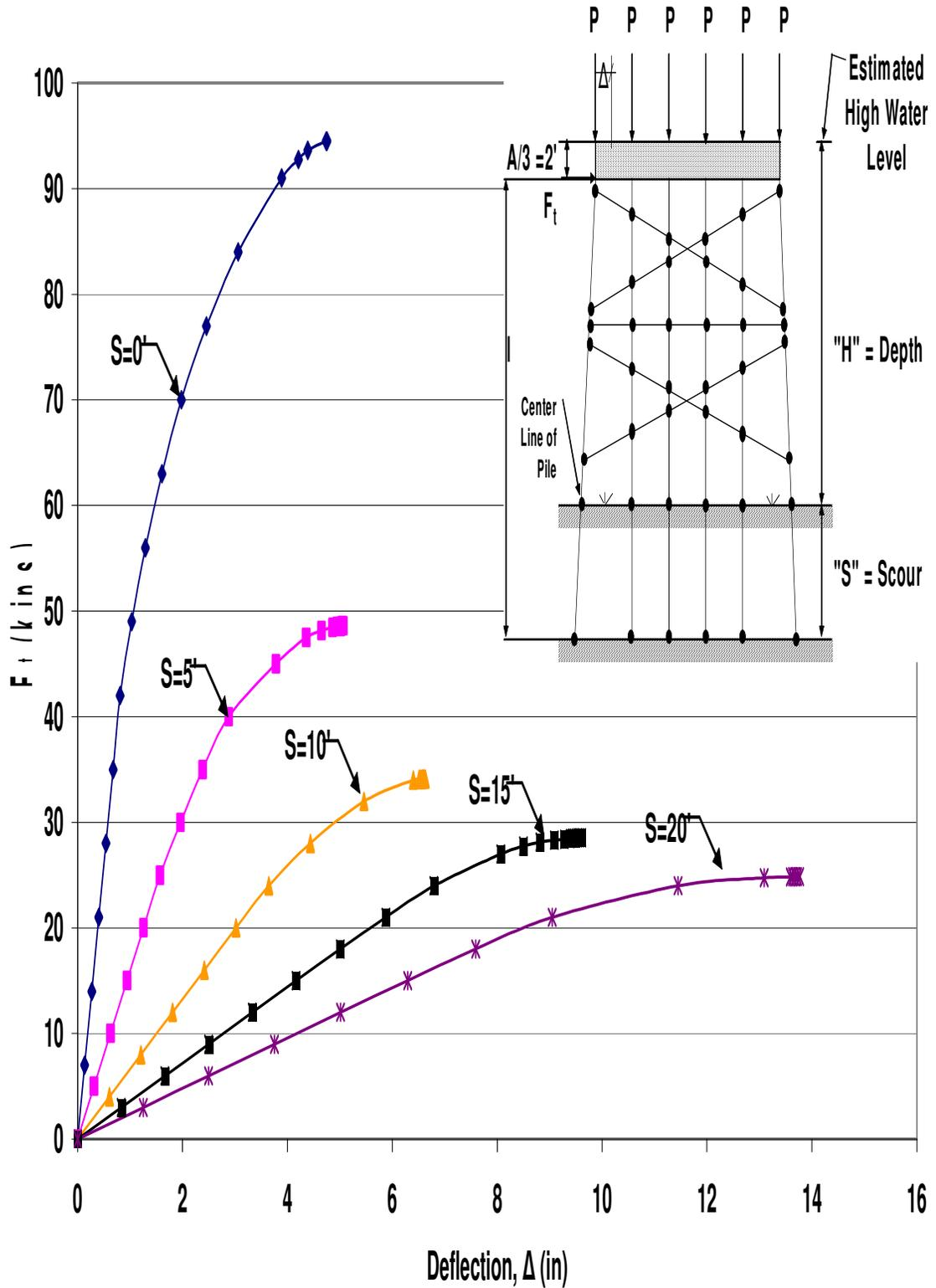
Figure B.99 HP12x53 Two-Story Single X-Braced 6-Pile Bent with  $H=21'$ ,  $P=140$ kips and  $A=6'$  Pushover Analysis Results
