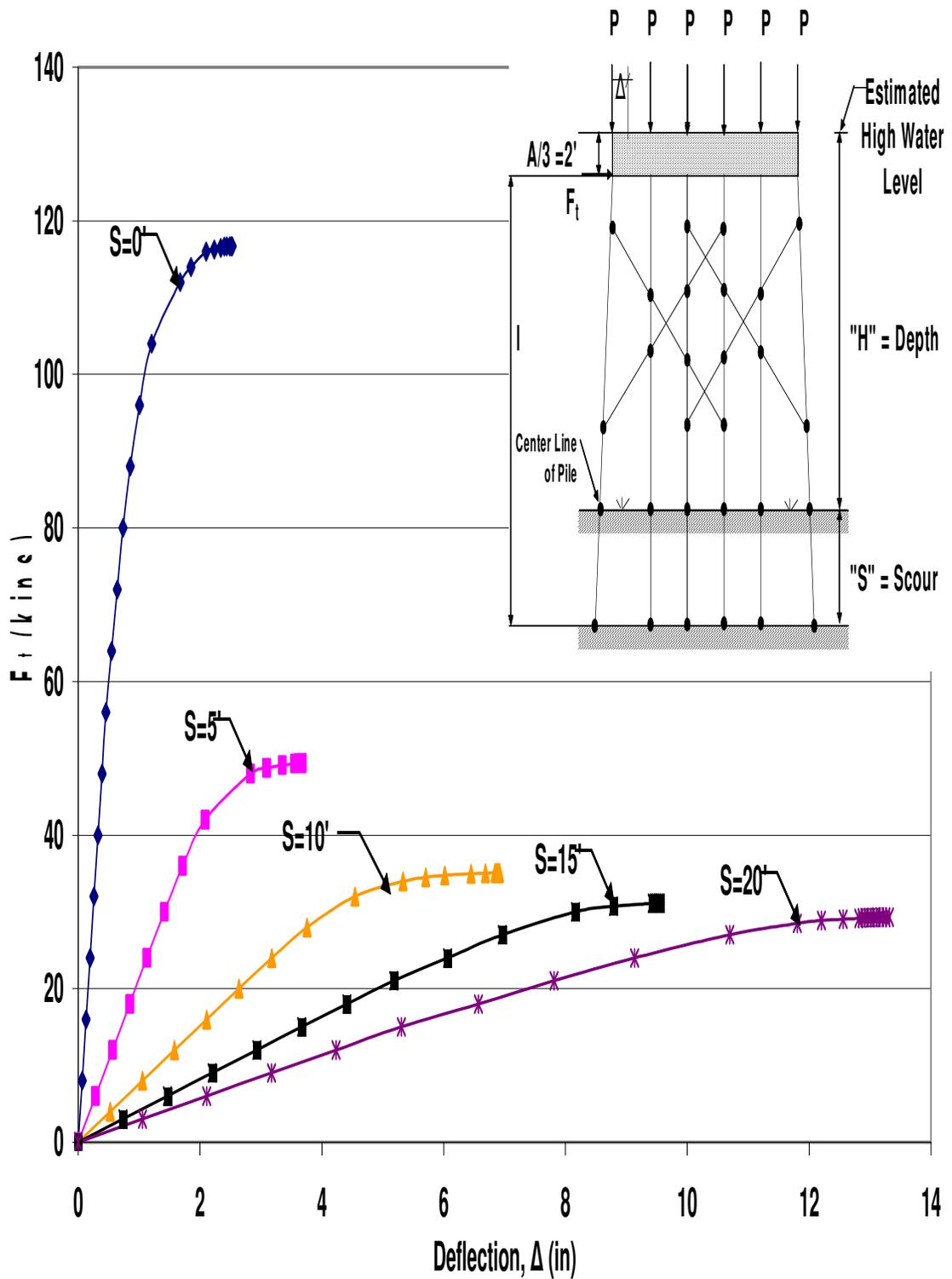
Figure B.95 HP12x53 Double X-Braced 6-Pile Bent with  $H=17'$ ,  $P=140$ kips and  $A=6'$
