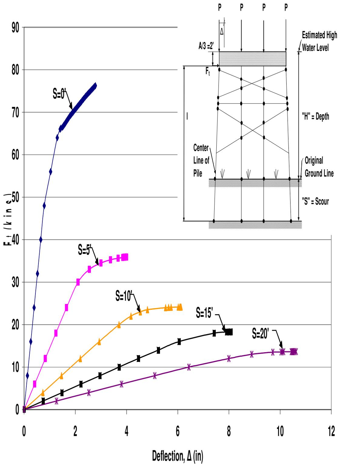
Figure B.46 HP12x53 Two-Story X-Braced 4-Pile Bent with  $H=25'$ ,  $P=120$ kips and  $A=6'$
