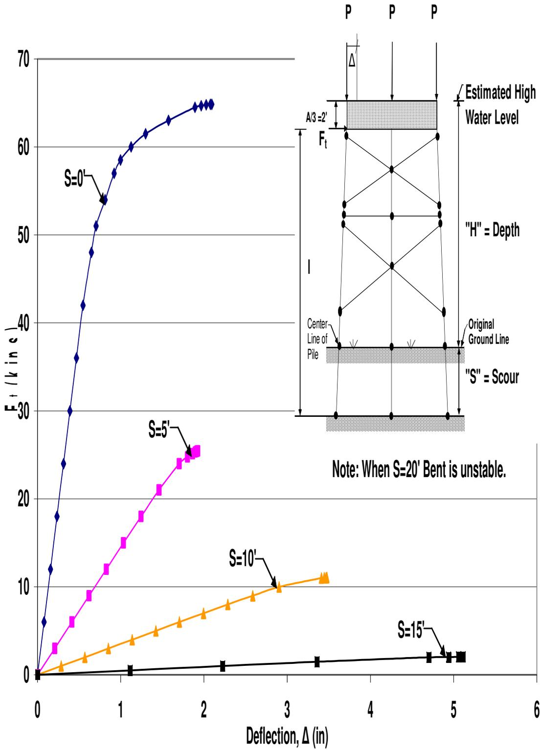
Figure B.20 HP12x53 Two-Story X-Braced 3-Pile Bent with  $H=21'$ ,  $P=160$ kips and  $A=6'$
