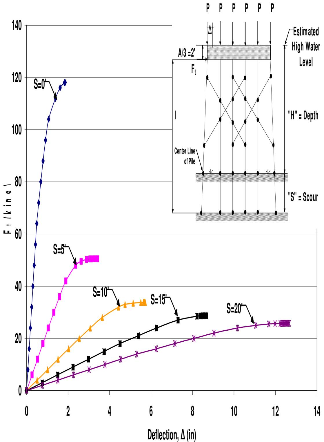
Figure B.92 HP12x53 Double X-Braced 6-Pile Bent with  $H=13'$ ,  $P=160$  kips and  $A=6'$
