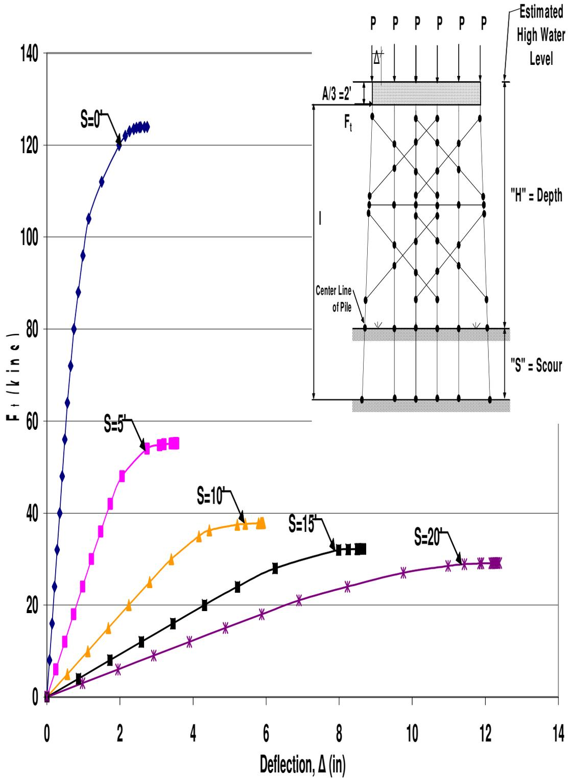
Figure B.107 HP12x53 Two-Story Double X-Braced 6-Pile Bent with  $H=21'$ ,  $P=140$ kips and  $A=6'$  Pushover Analysis Results
