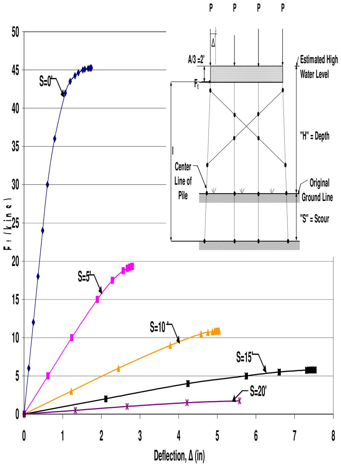
Figure A.36 HP10x42 X-Braced 4-Pile Bent with H=13', P=160 kips and A=6'
