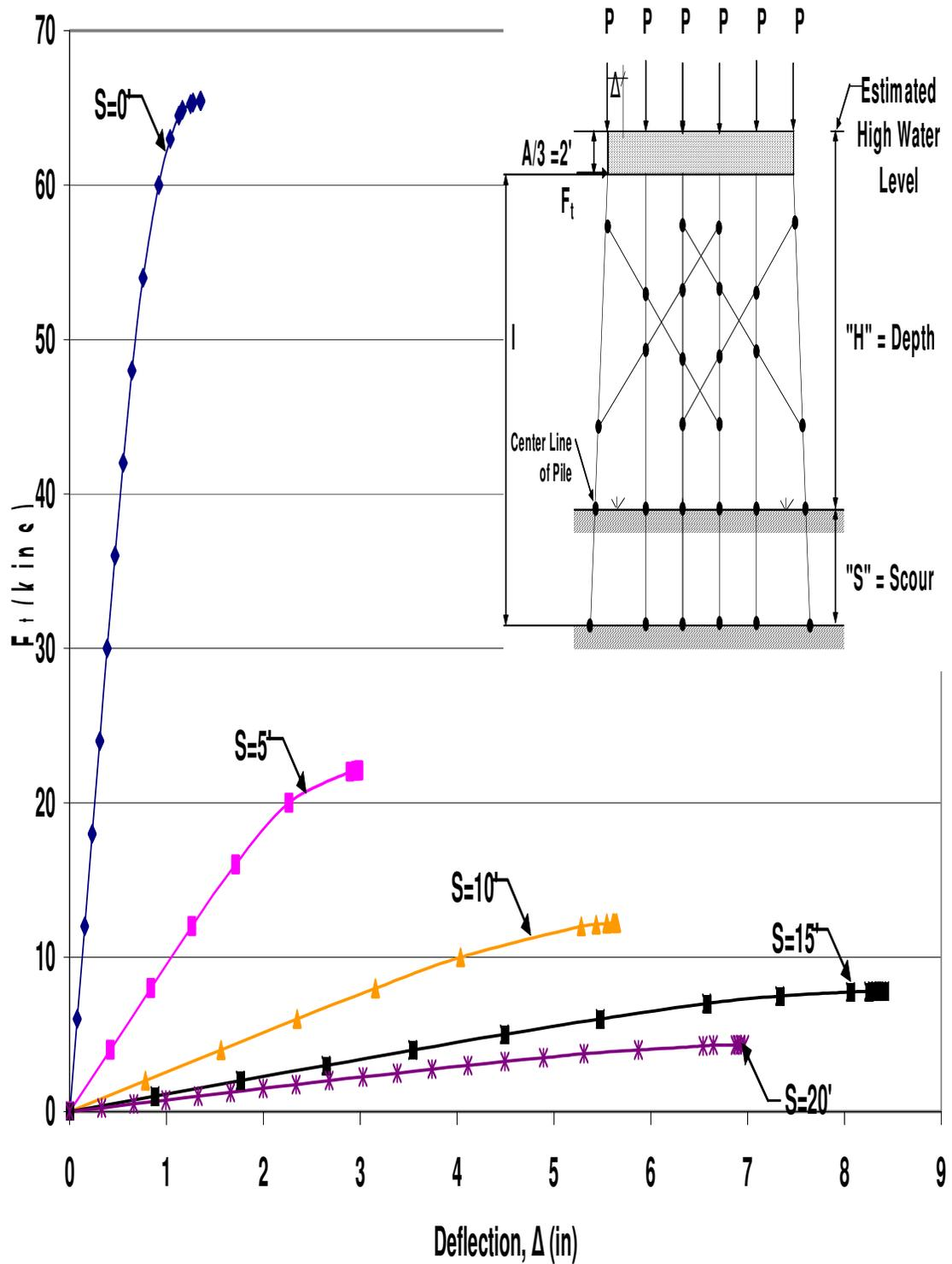
Figure A.96 HP10x42 Double X-Braced 6-Pile Bent with  $H=17'$ ,  $P=160$  kips and  $A=6'$
