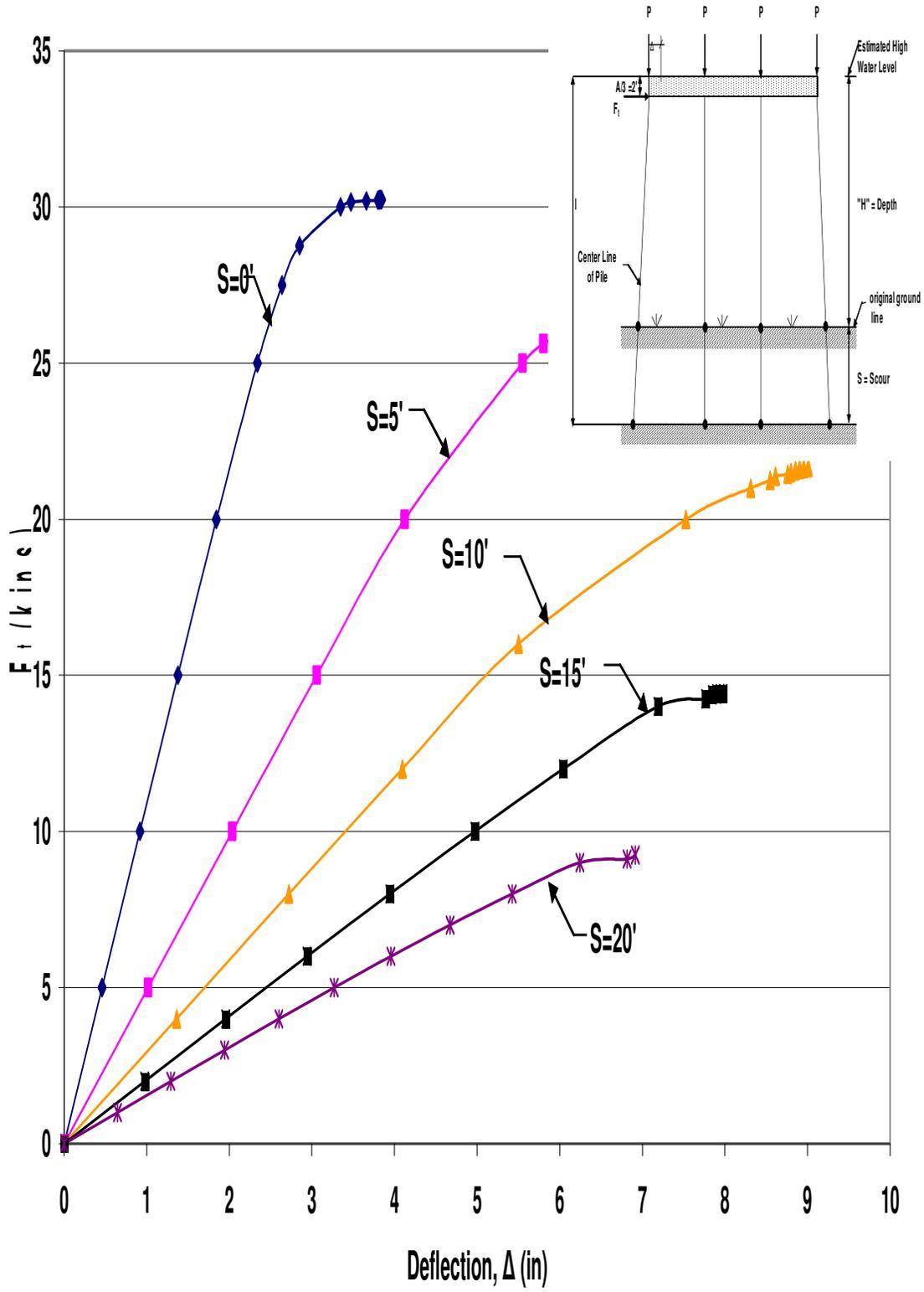
Figure A.29 HP10x42 Unbraced 4-Pile Bent with  $H=13'$ ,  $P=100$ kips and  $A=6'$
