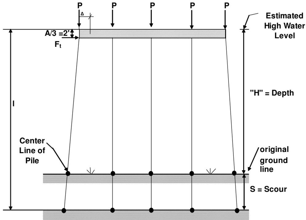
Figure 3.5 Typical Unbraced Bent and Typical Loading Conditions
