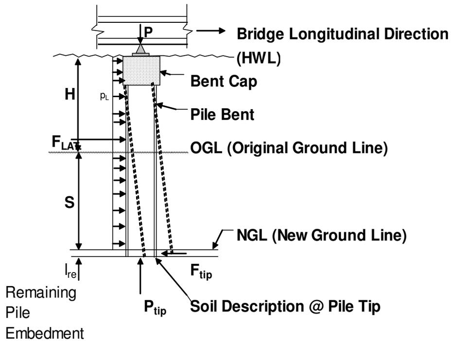
Figure 4.3 Evaluation of Bent Pile “Kick-Out” Load from Extreme Flood/Scour Event
