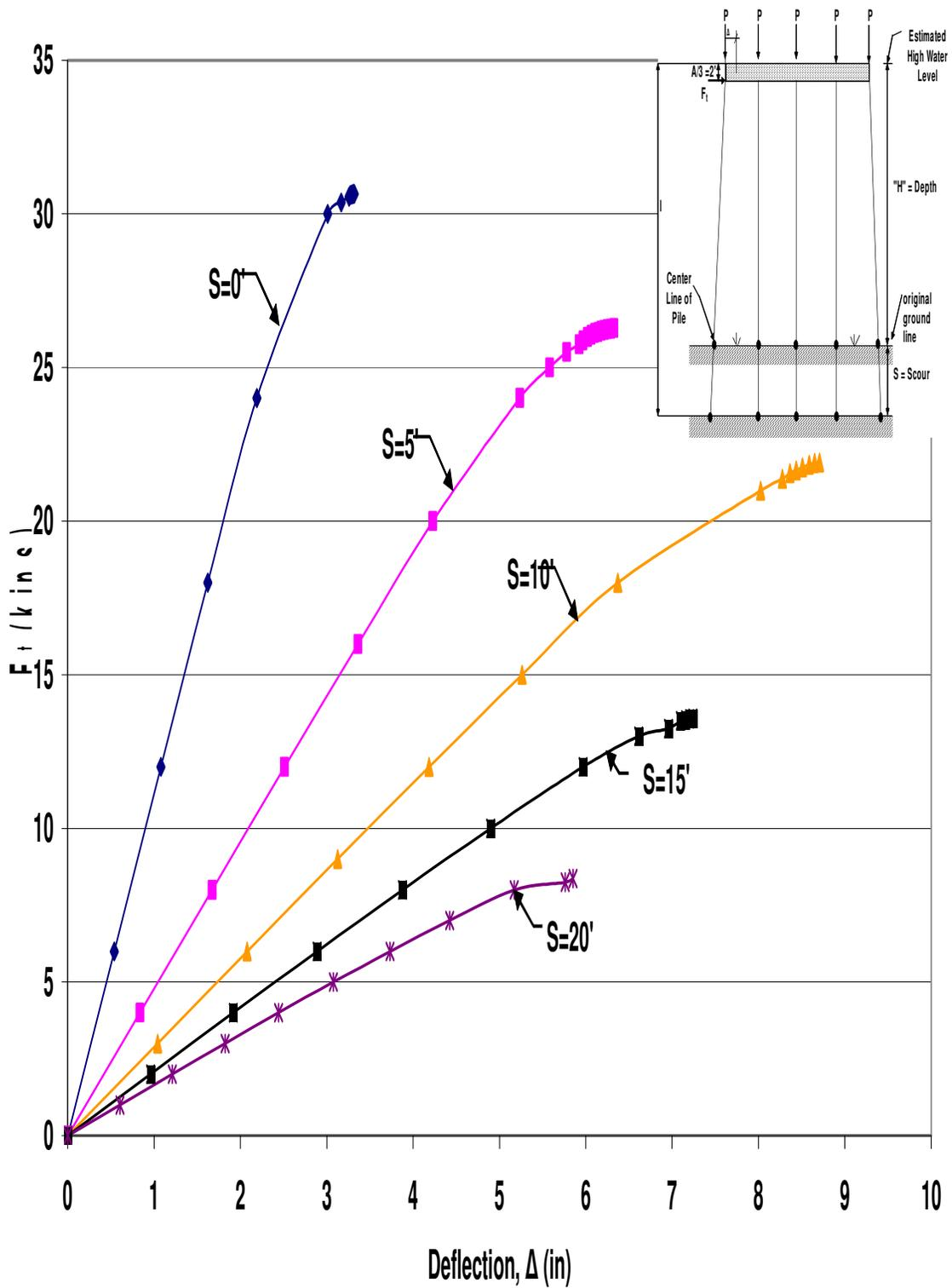
Figure A.55 HP10x42 Unbraced 5-Pile Bent with  $H=13'$ ,  $P=140$ kips and  $A=6'$
