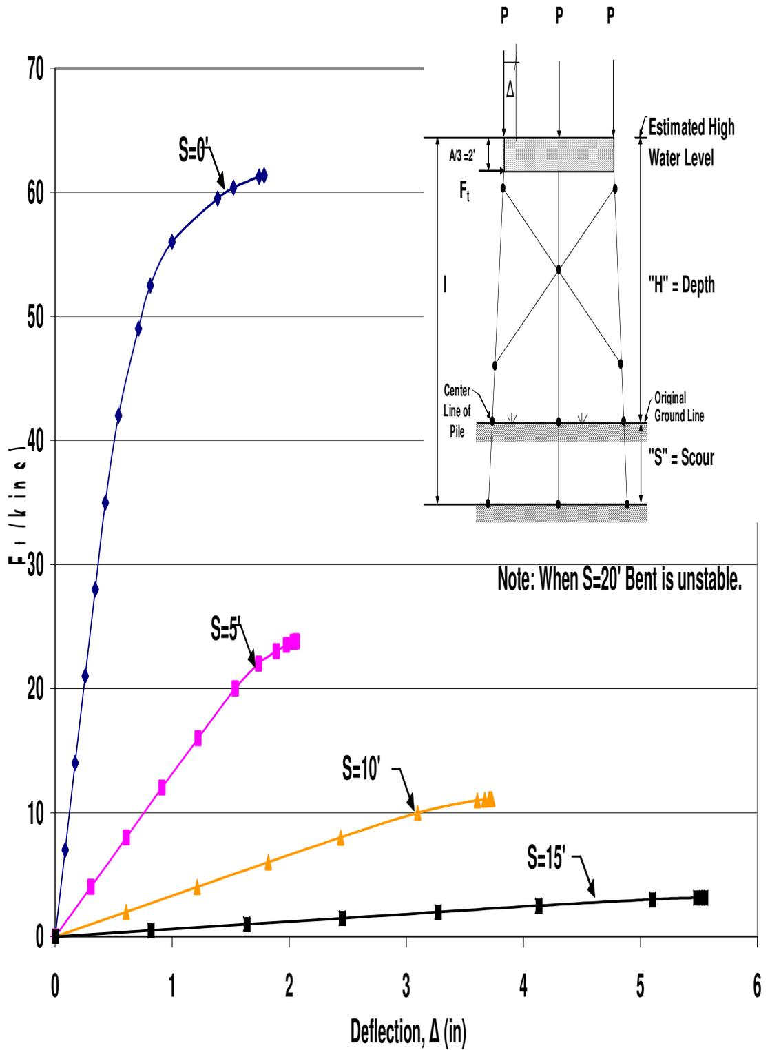
Figure B.12 HP12x53 X-Braced 3-Pile Bent with  $H=13'$ ,  $P=160$ kips and  $A=6'$
