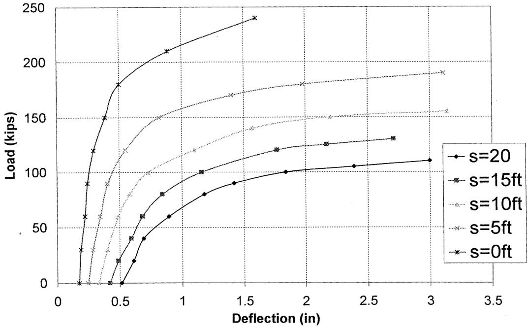
Figure 2.16  $P-\Delta_{top}$  Curves in Transverse Direction for Pile Bent in Figure 2.14 for Batter = 0.083 (Brown and Ramey 2003)
