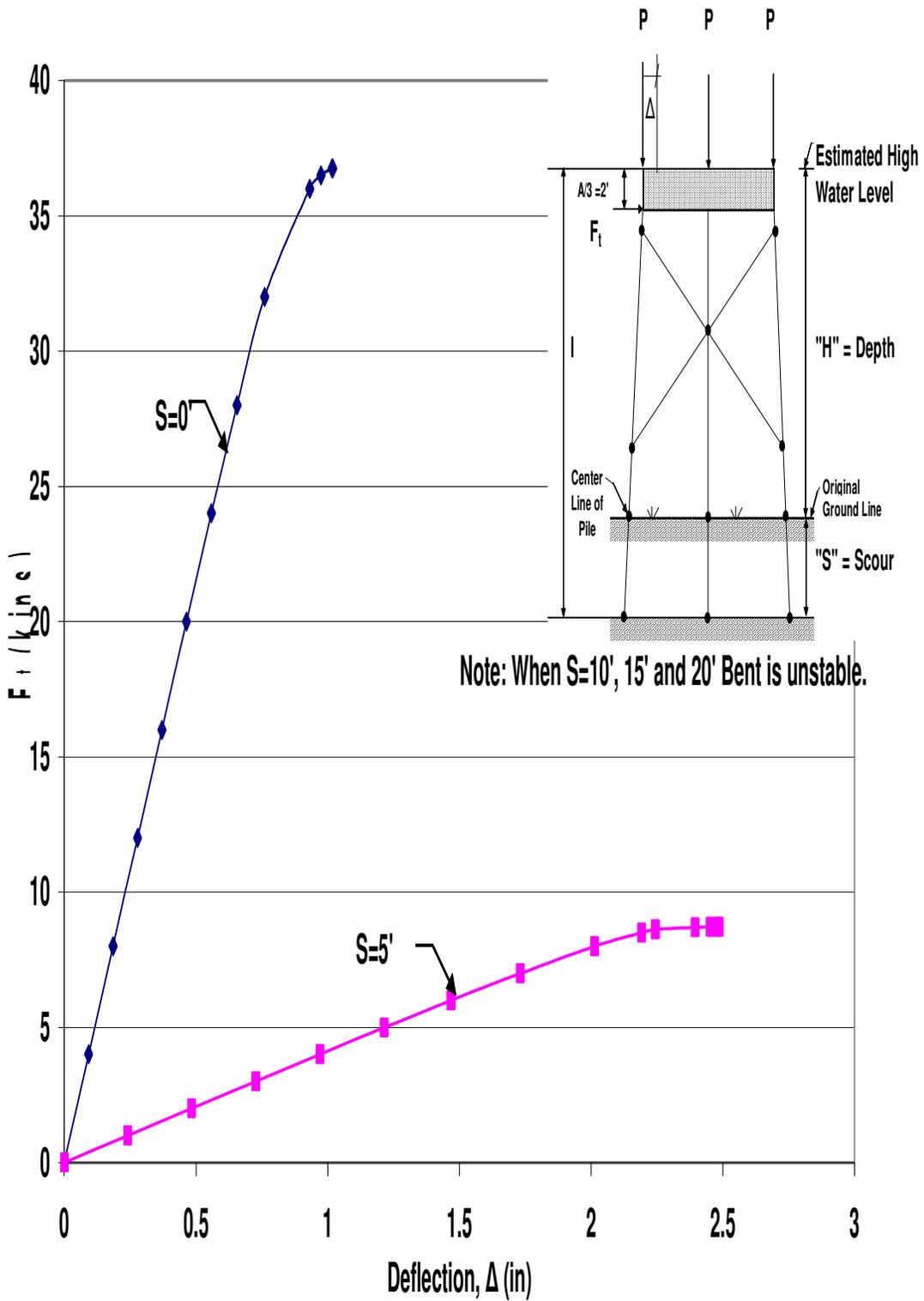
Figure A.16 HP10x42 X-Braced 3-Pile Bent with  $H=17'$ ,  $P=160$ kips and  $A=6'$
