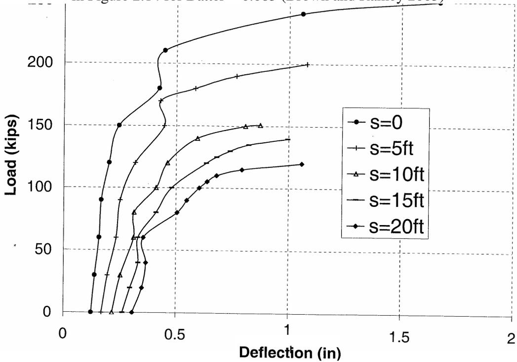
Figure 2.17  $P-\Delta_{top}$  Curves in Transverse Direction for Pile Bent in Figure 2.14 for Batter = 0.125 (Brown and Ramey 2003)
