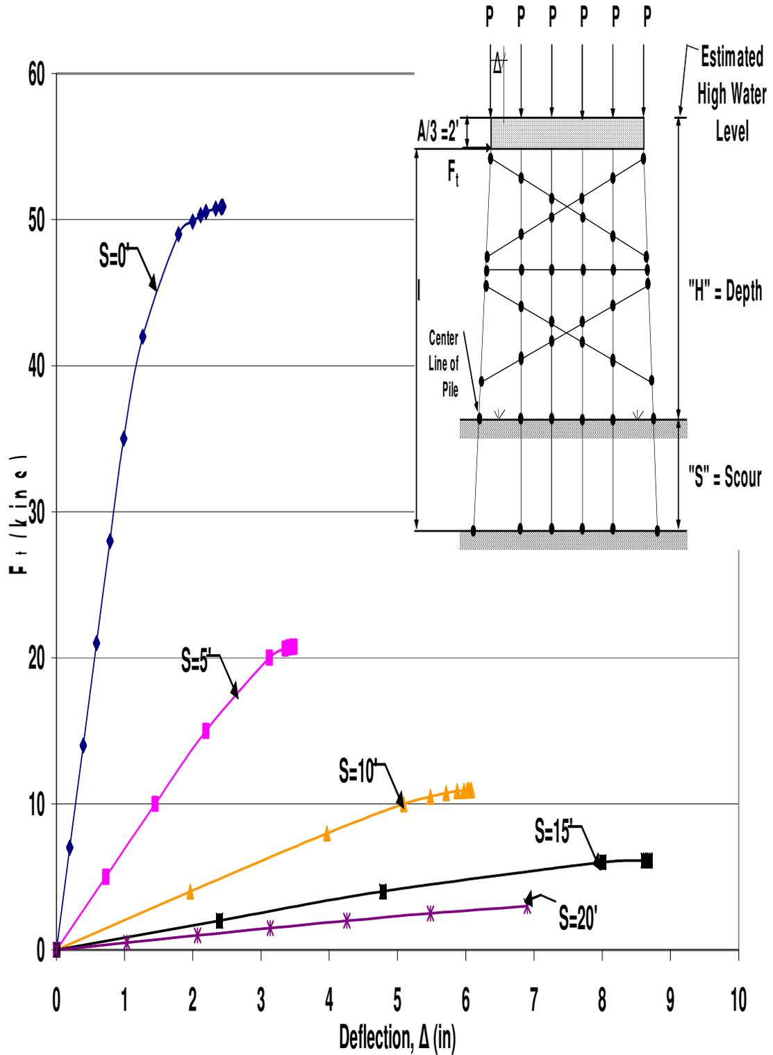
Figure A.103 HP10x42 Two-Story Single X-Braced 6-Pile Bent with H=25', P=140kips and A=6' Pushover Analysis Results
