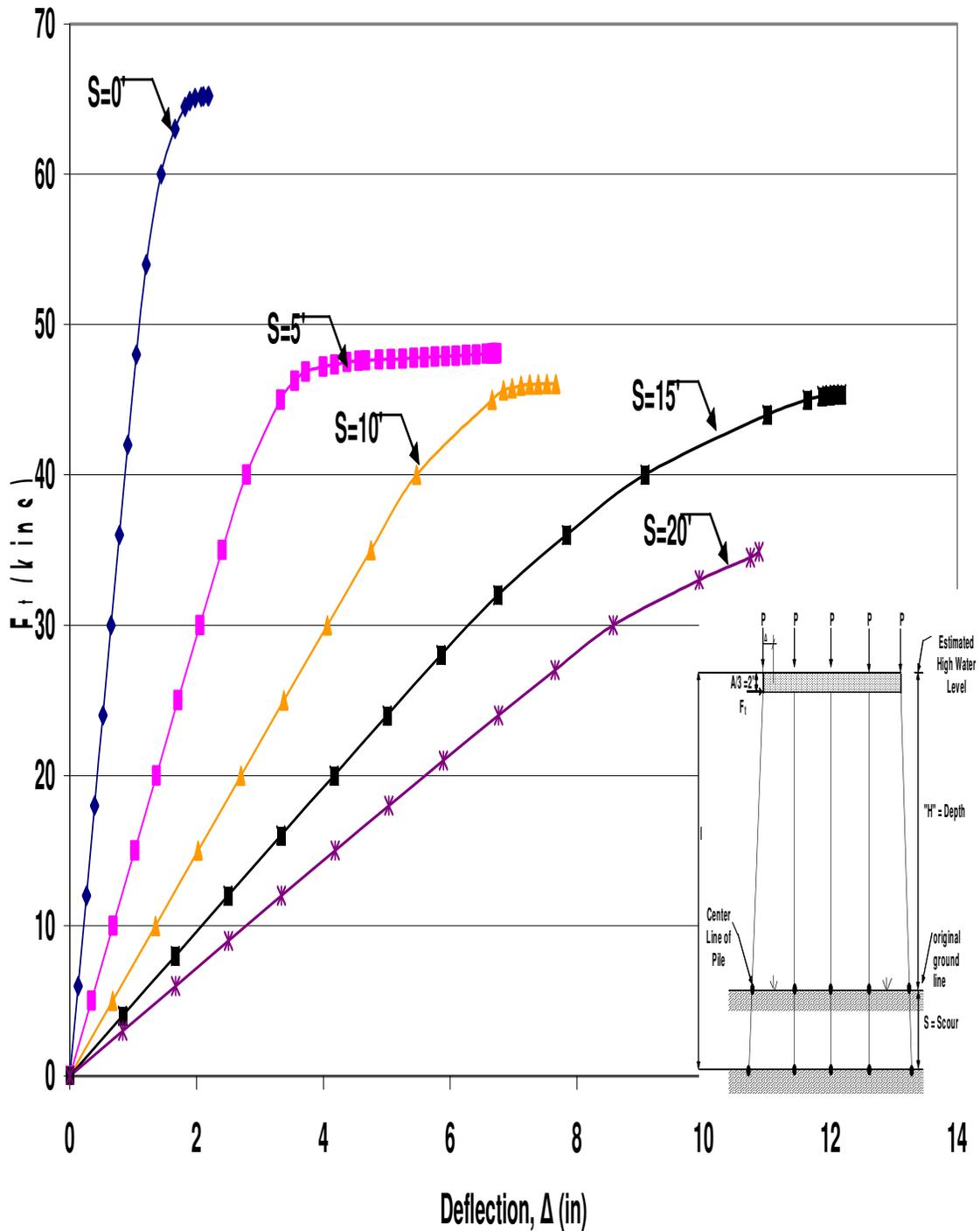
Figure B.50 HP12x53 Unbraced 5-Pile Bent with H=10', P=120kips and A=6'
