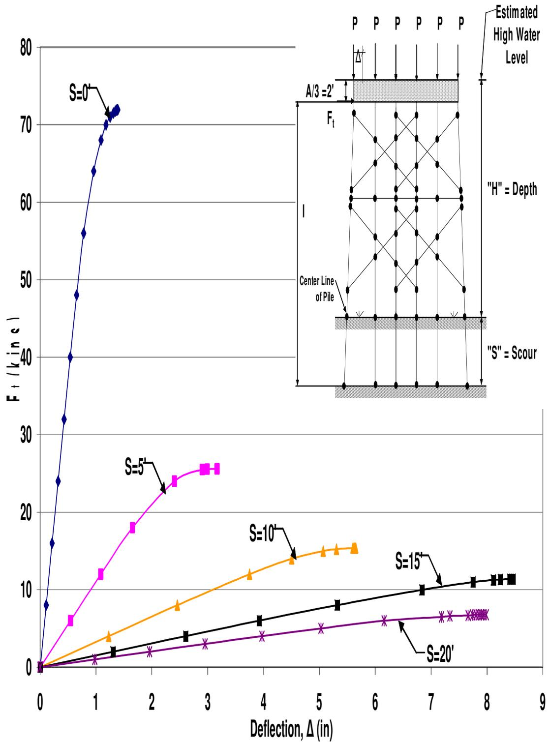
Figure A.111 HP10x42 Two-Story Double X-Braced 6-Pile Bent with  $H=25'$ ,  $P=140$ kips and  $A=6'$  Pushover Analysis Results
