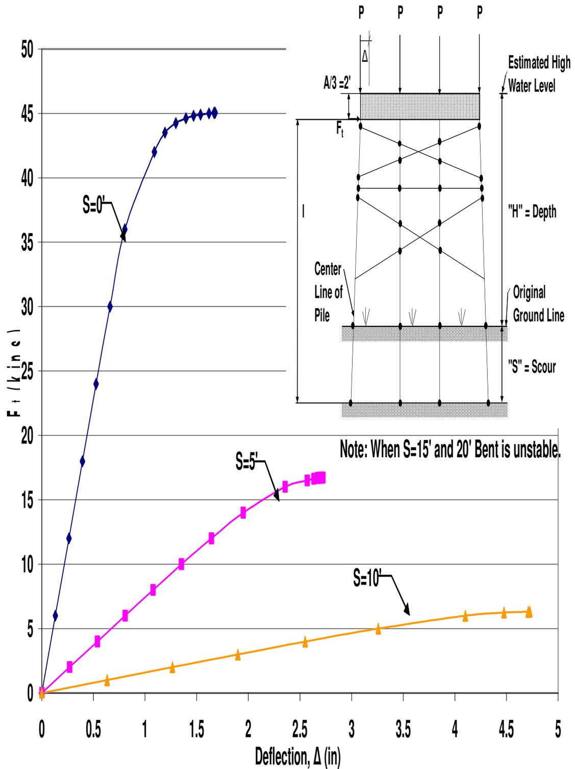
Figure A.44 HP10x42 Two-Story X-Braced 4-Pile Bent with  $H=21'$ ,  $P=160$ kips, and  $A=6'$
