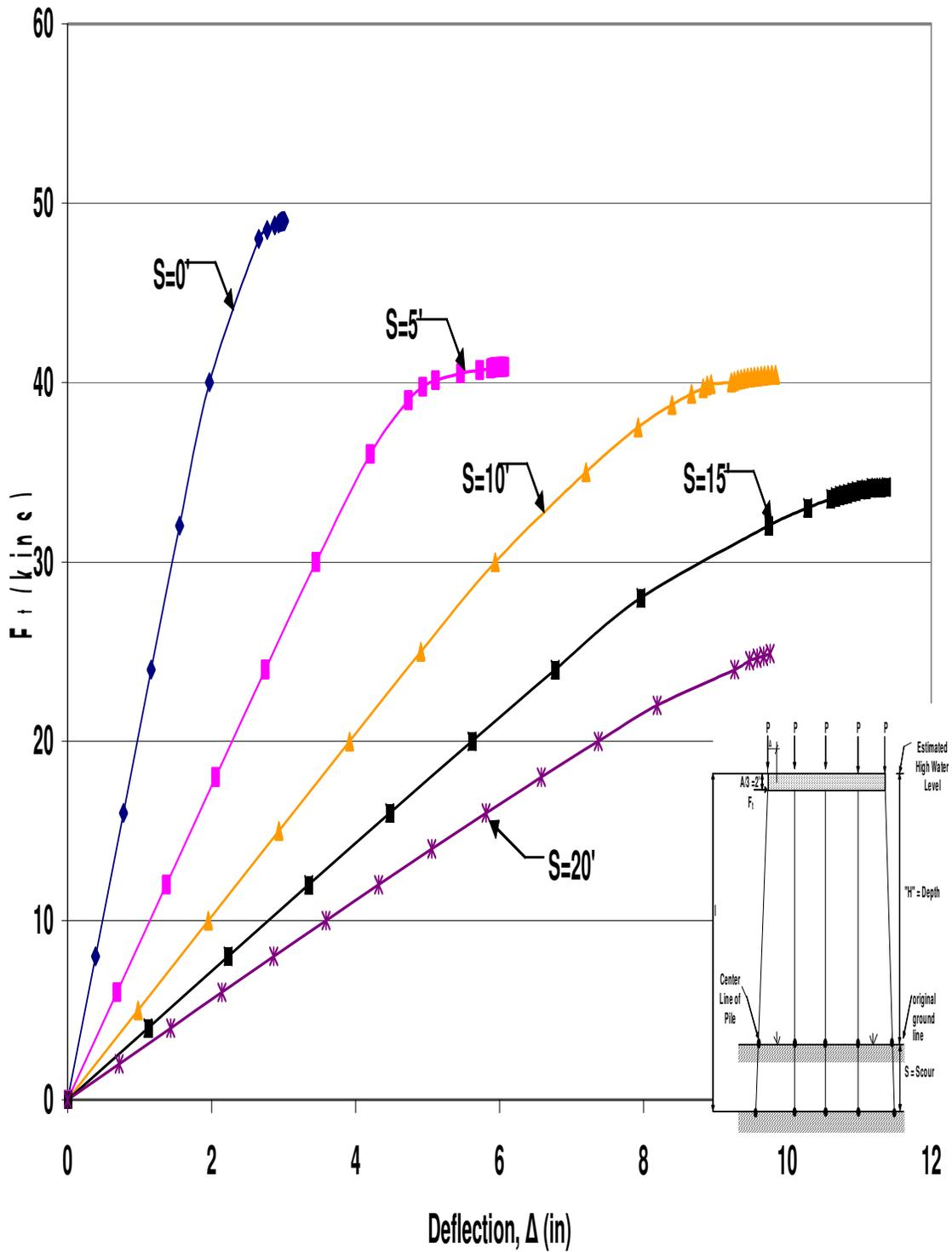
Figure B.55 HP12x53 Unbraced 5-Pile Bent with H=13', P=140kips and A=6'
