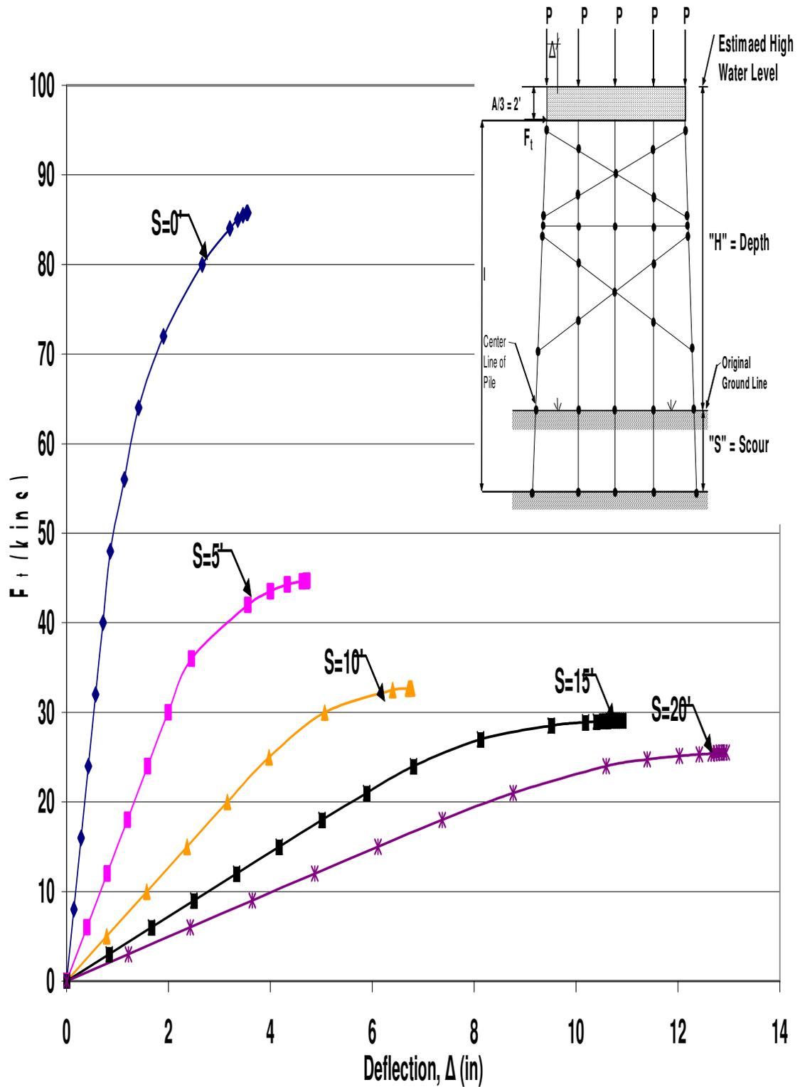
Figure B.70 HP12x53 Two-Story X-Braced 5-Pile Bent with  $H=25'$ ,  $P=120$ kips and  $A=6'$
