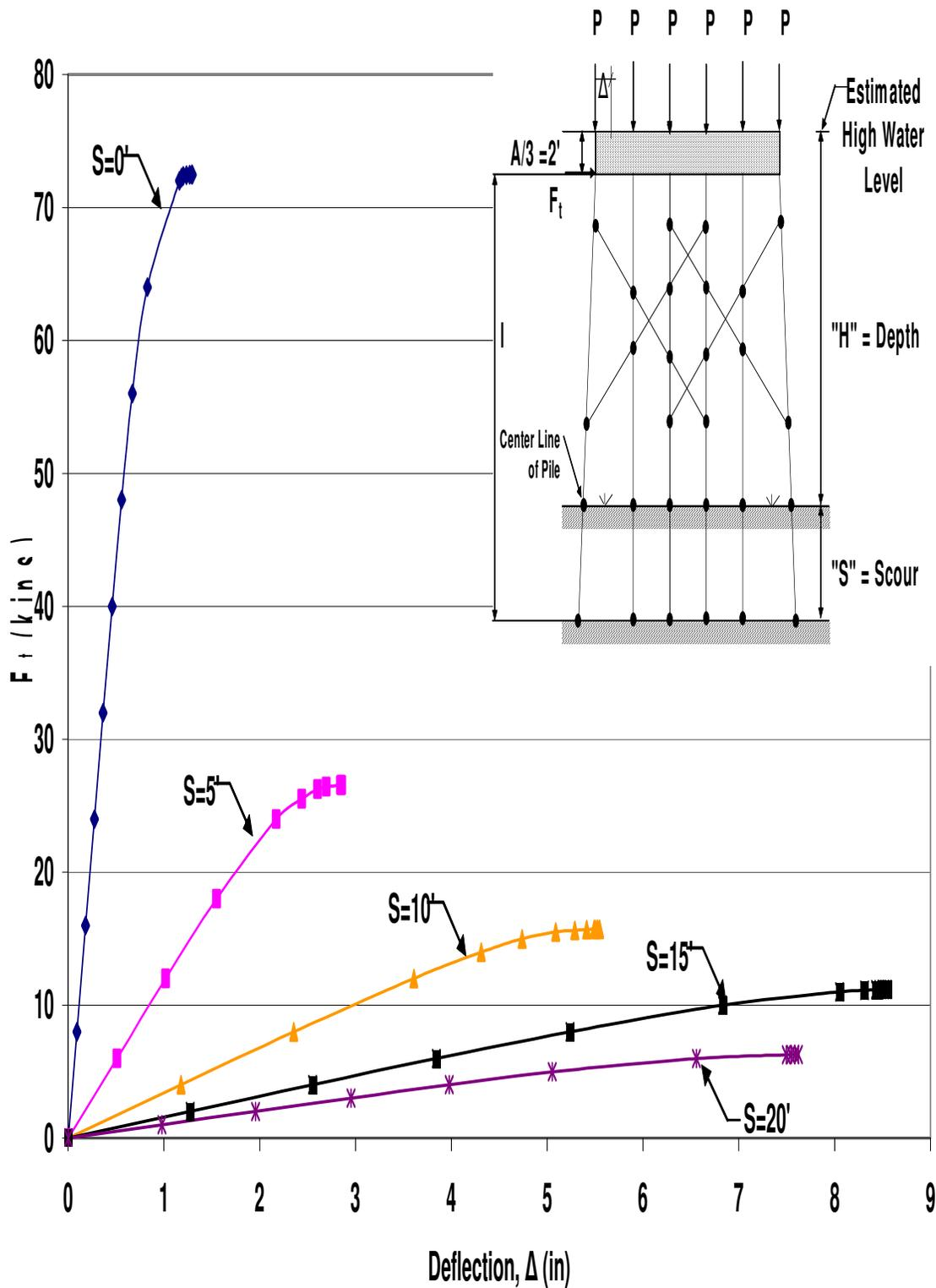
Figure A.92 HP10x42 Double X-Braced 6-Pile Bent with  $H=13'$ ,  $P=160$ kips and  $A=6'$
