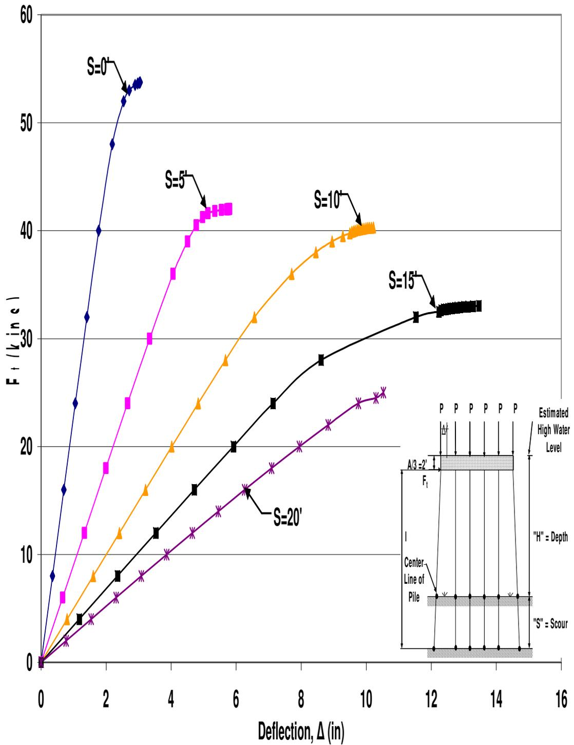
Figure B.79 HP12x53 Unbraced 6-Pile Bent with  $H=13'$ ,  $P=140$ kips and  $A=6'$
