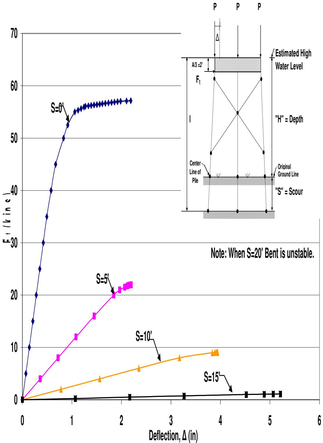
Figure B.16 HP12x53 X-Braced 3-Pile Bent with H=17', P=160 kips and A=6'
