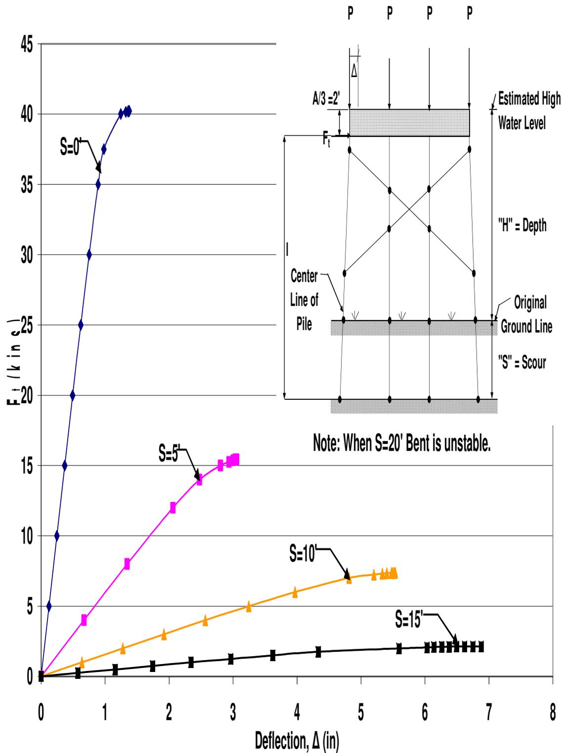
Figure A.40 HP10x42 X-Braced 4-Pile Bent with H=17', P=160kips, and A=6'
