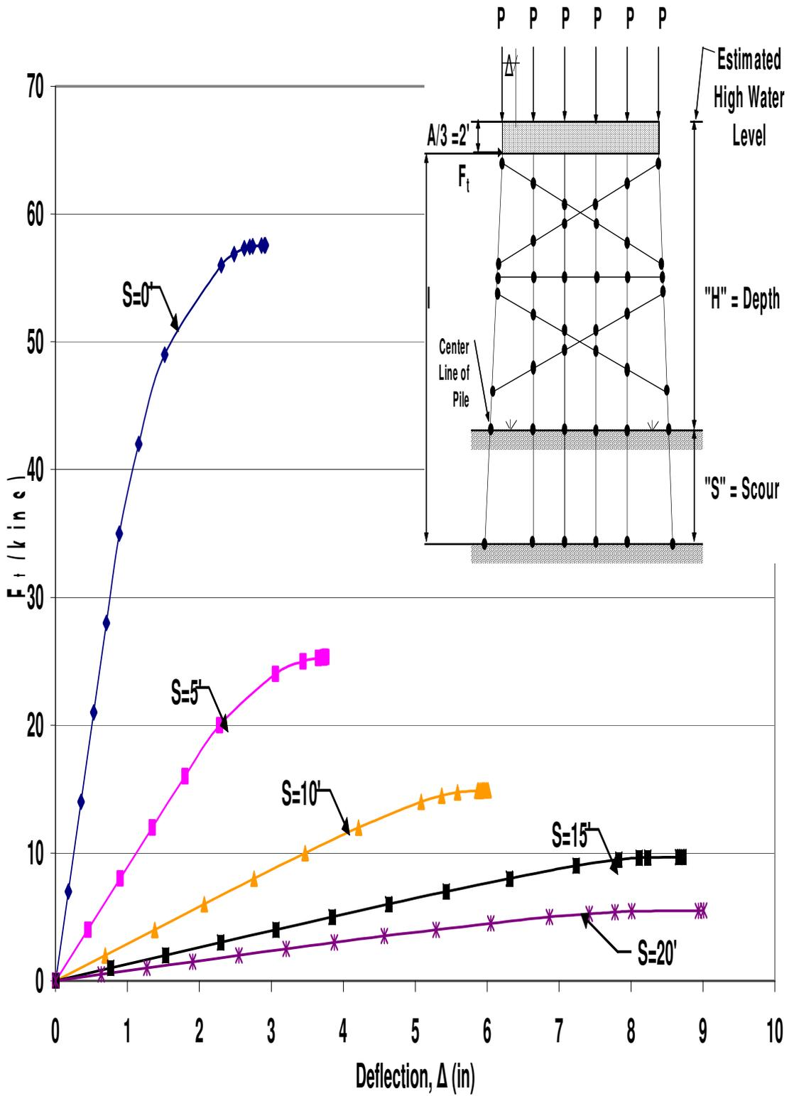
Figure A.99 HP10x42 Two-Story Single X-Braced 6-Pile Bent with  $H=21'$ ,  $P=140$  kips and  $A=6'$  Pushover Analysis Results
