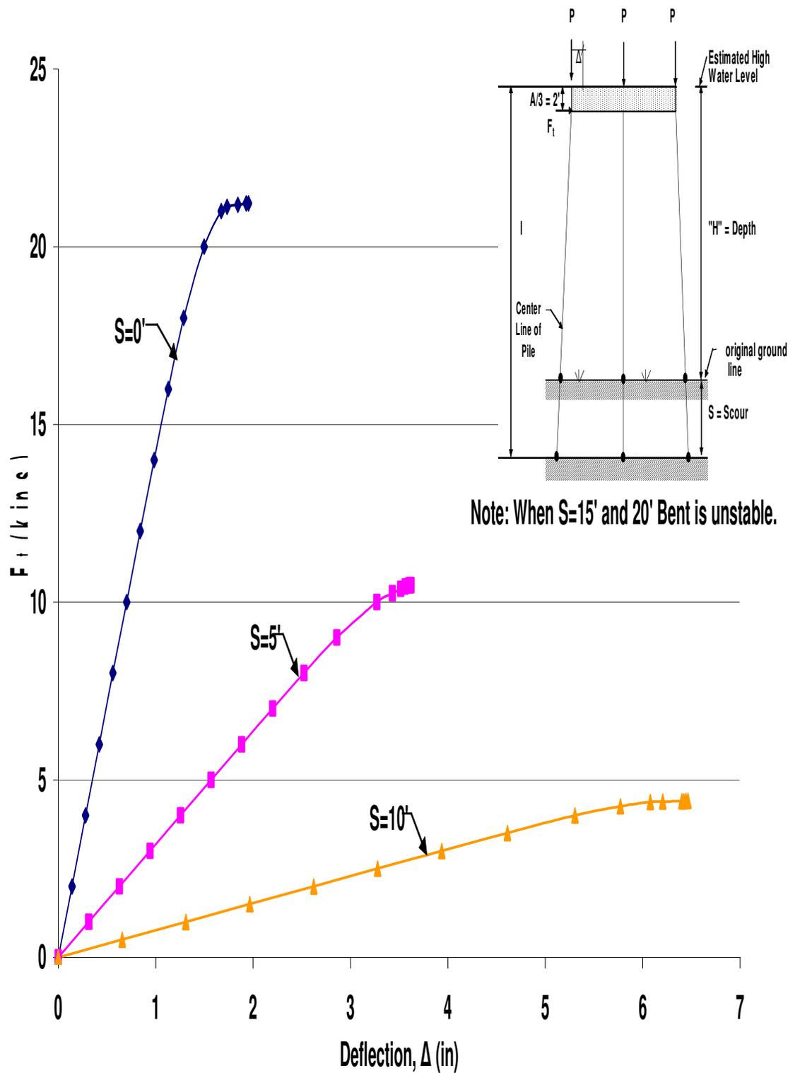
Figure A.1 HP10x42 Unbraced 3-Pile Bent with  $H=10'$ ,  $P=100$ kips, and  $A=6'$
