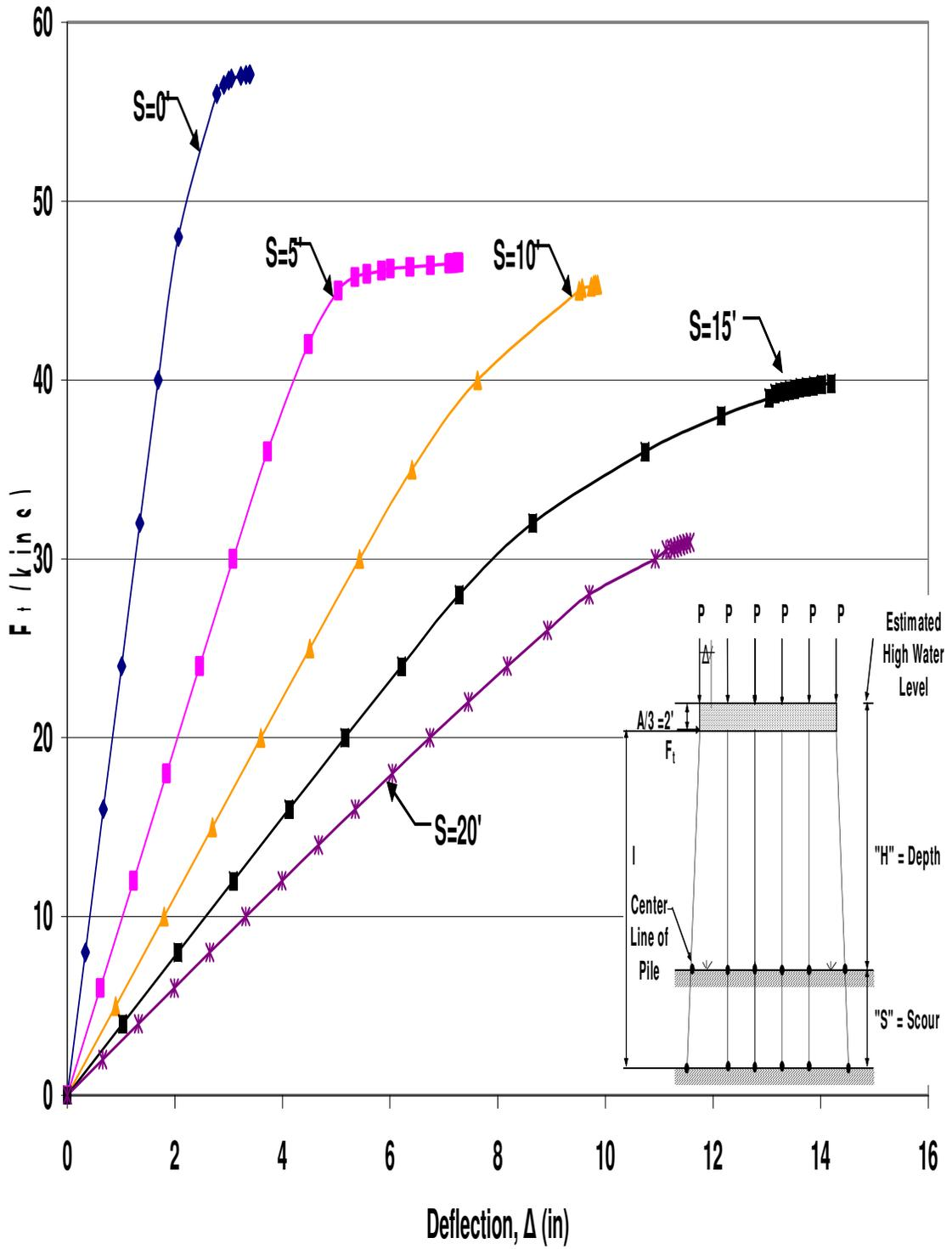
Figure B.78 HP12x53 Unbraced 6-Pile Bent with  $H=13'$ ,  $P=120$ kips and  $A=6'$
