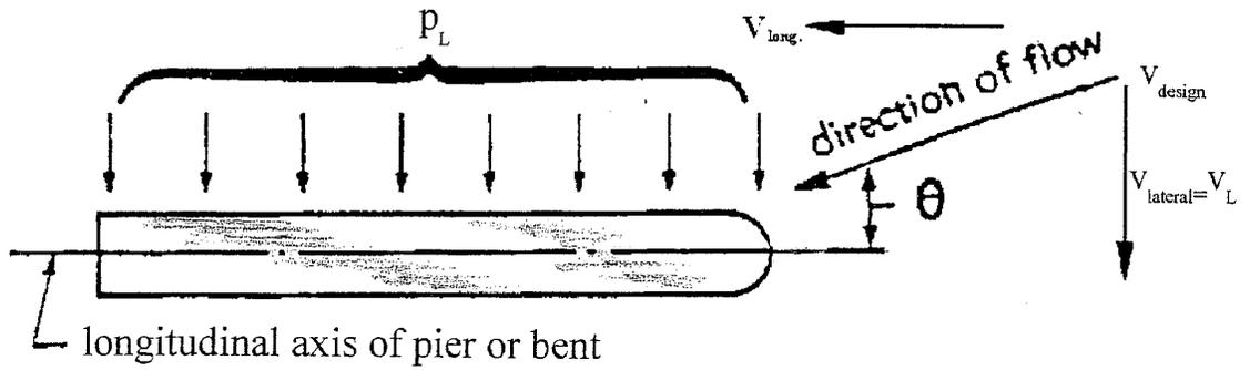
Figure 4.8 Plan View of Pier Showing Stream Flow and Lateral Pressure (AASHTO 1997)
