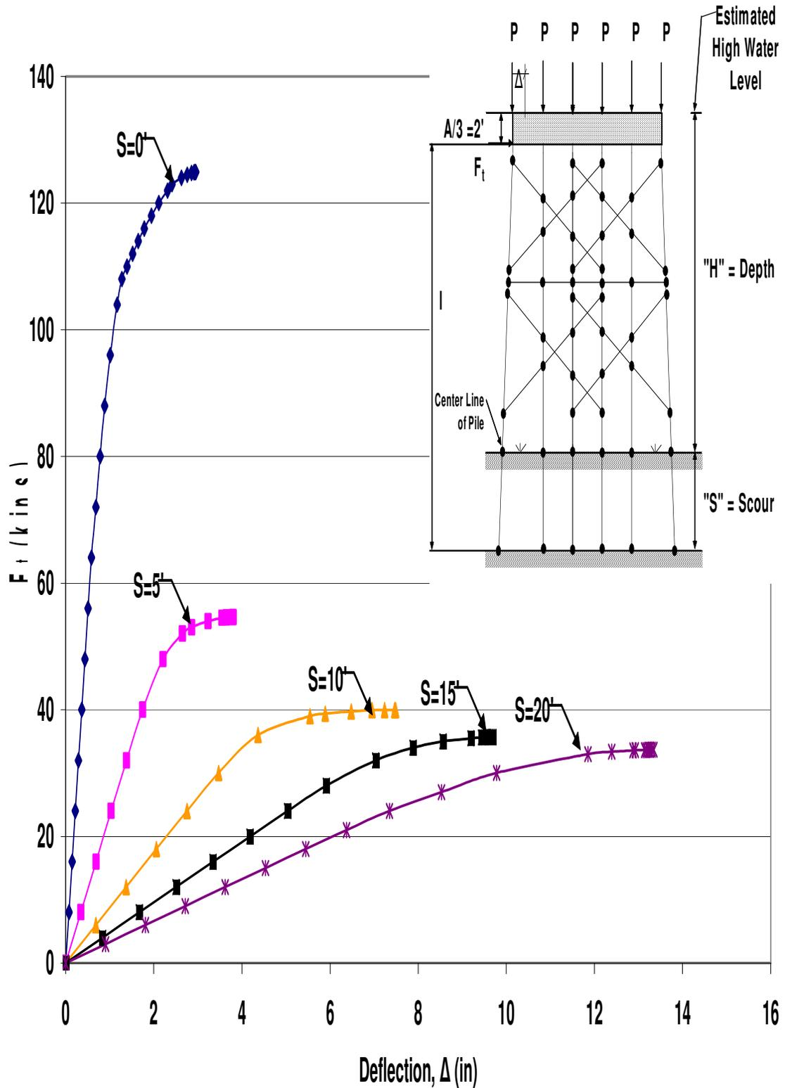
Figure B.110 HP12x53 Two-Story Double X-Braced 6-Pile Bent with  $H=25'$ ,  $P=120$ kips and  $A=6'$  Pushover Analysis Results
