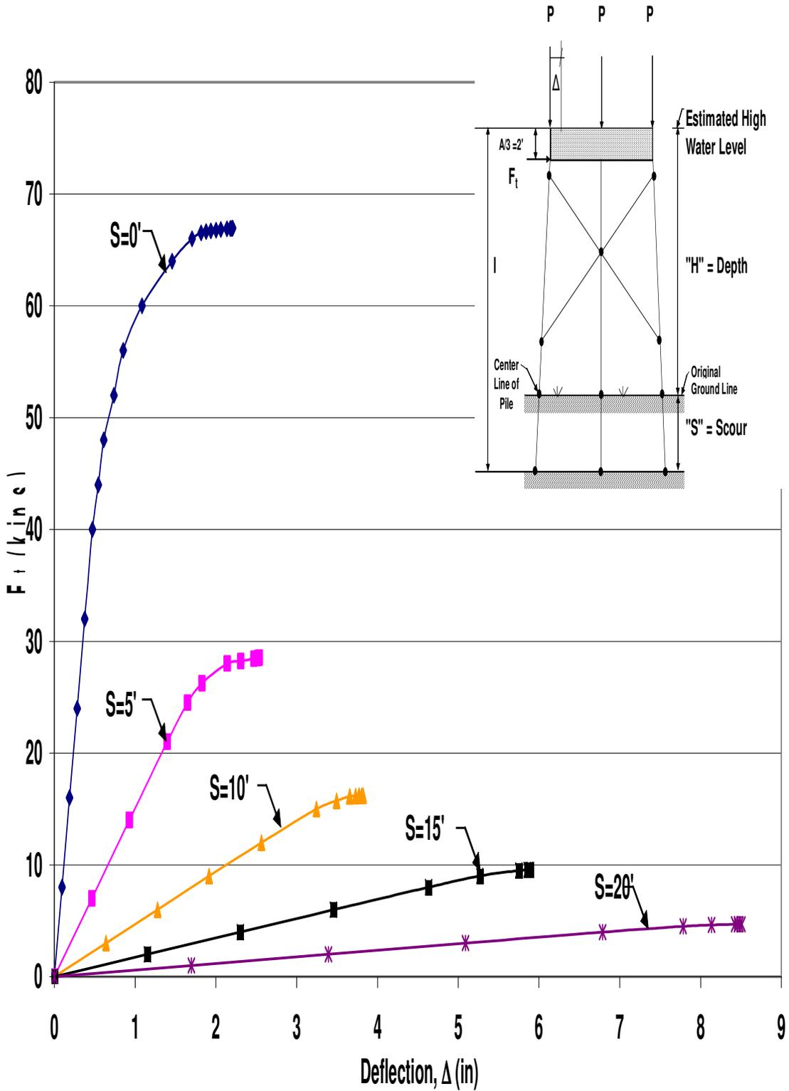
Figure B.9 HP12x53 X-Braced 3-Pile Bent with  $H=13'$ ,  $P=100$ kips and  $A=6'$
