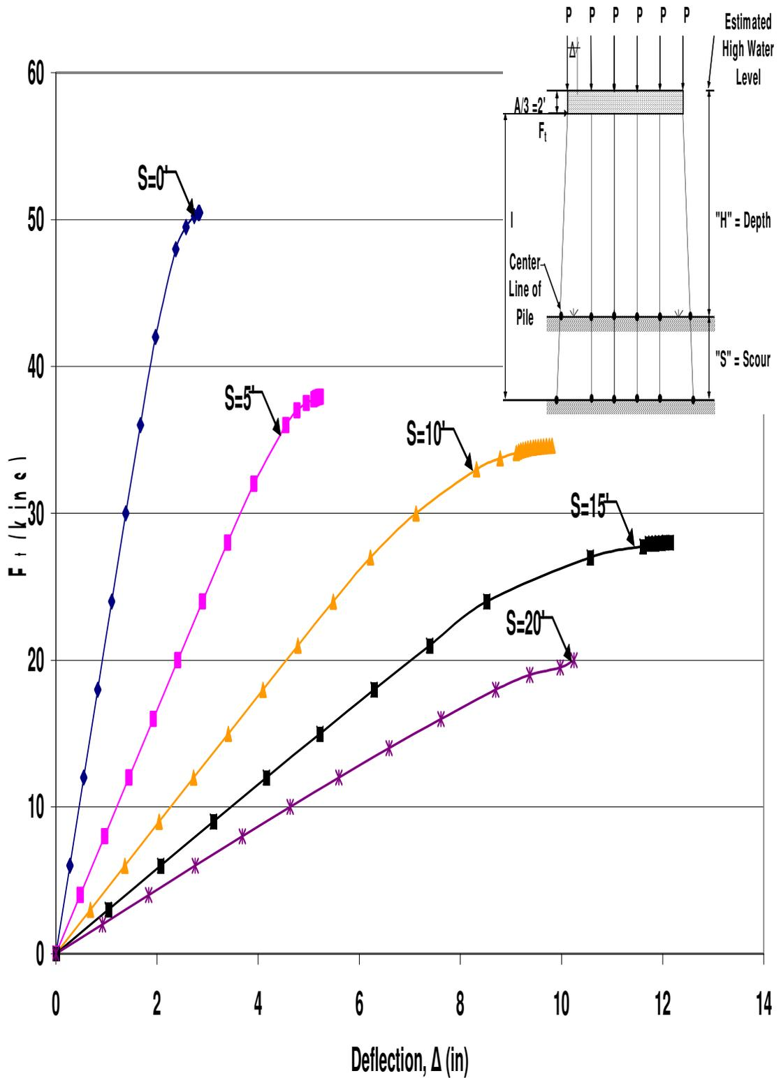
Figure B.80 HP12x53 Unbraced 6-Pile Bent with  $H=13'$ ,  $P=160$ kips and  $A=6'$
