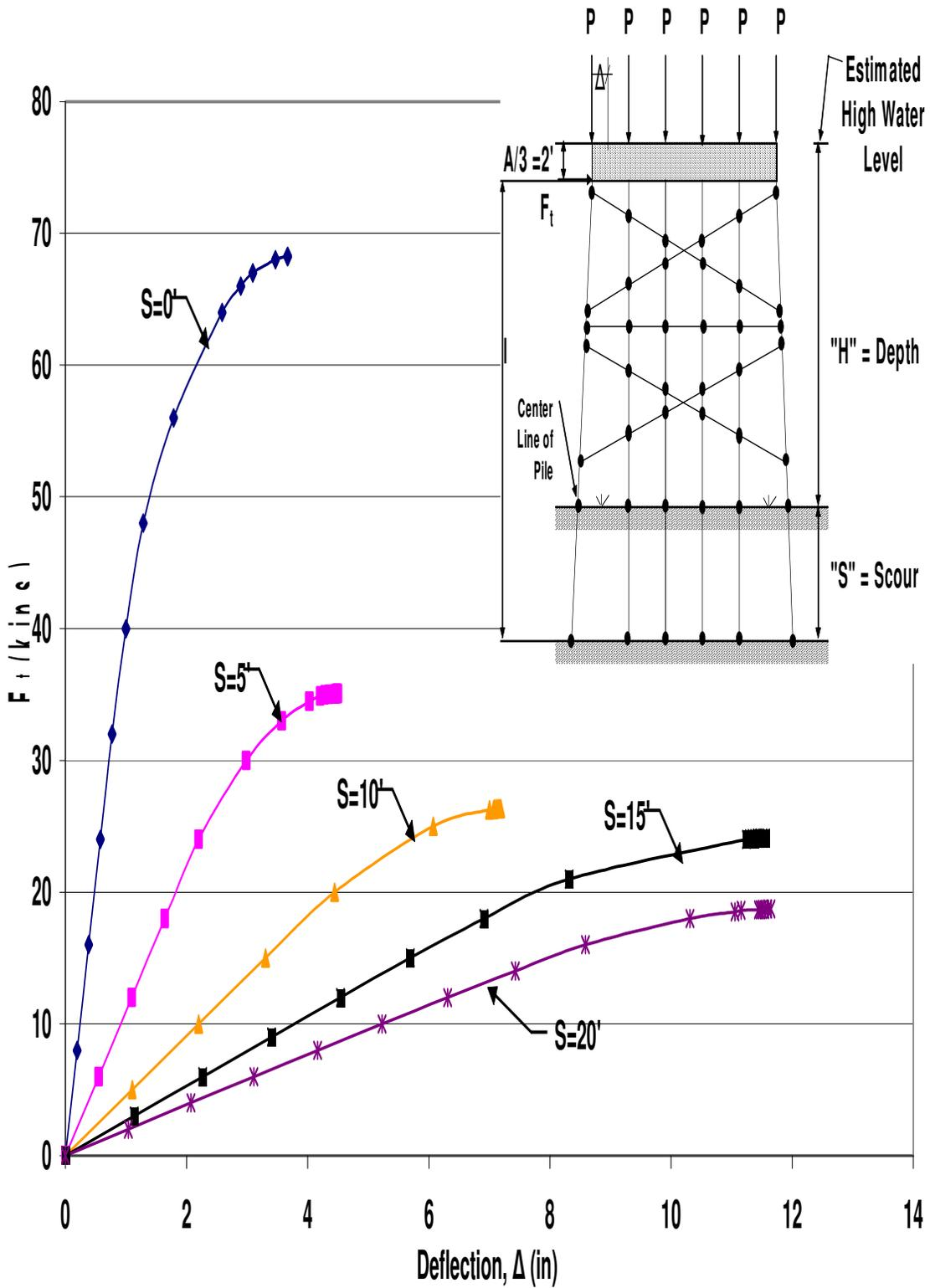
Figure A.97 HP10x42 Two-Story Single X-Braced 6-Pile Bent with  $H=21'$ ,  $P=100$ kips and  $A=6'$  Pushover Analysis Results
