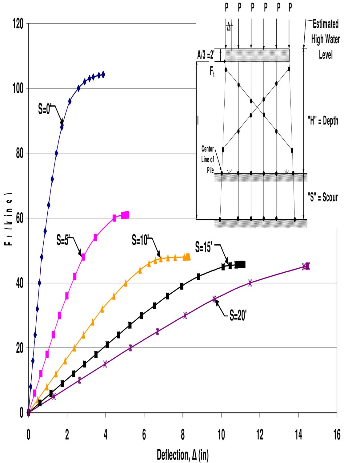
Figure B.81 HP12x53 Single X-Braced 6-Pile Bent with  $H=13'$ ,  $P=100$  kips and  $A=6'$
