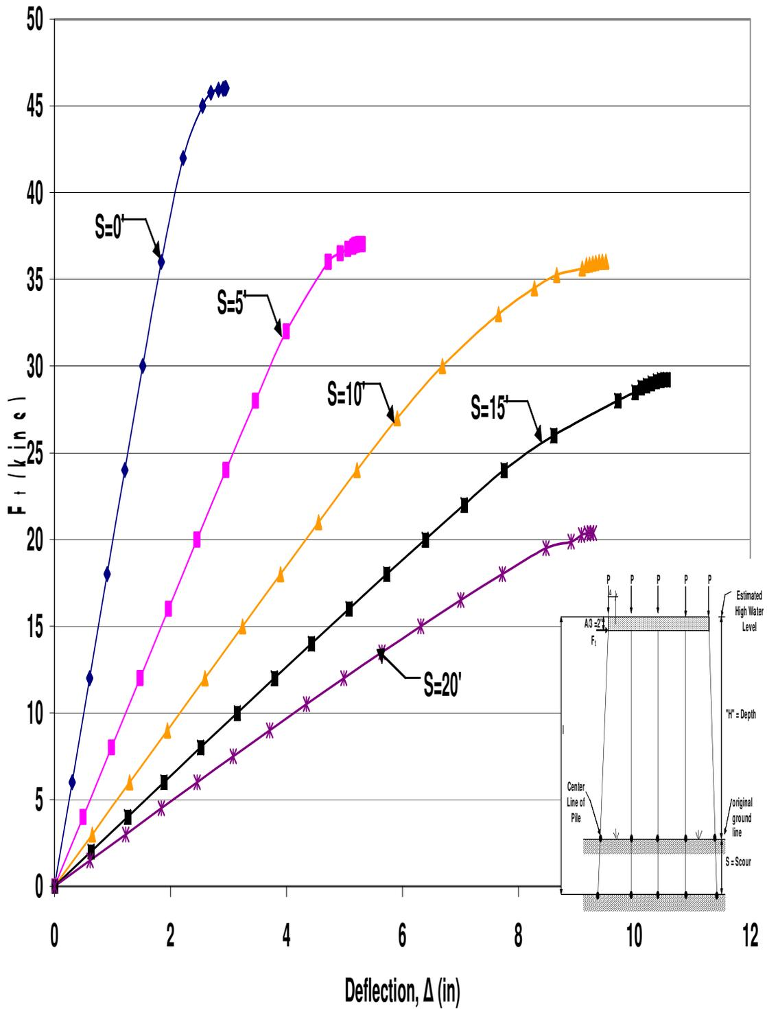
Figure B.56 HP12x53 Unbraced 5-Pile Bent with  $H=13'$ ,  $P=160$ kips and  $A=6'$
