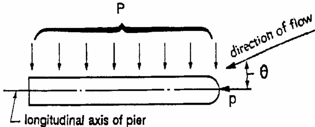
Figure 2.8 Plan View of Pier Showing Stream Flow Pressure (AASHTO 3.7.3.2-1)
