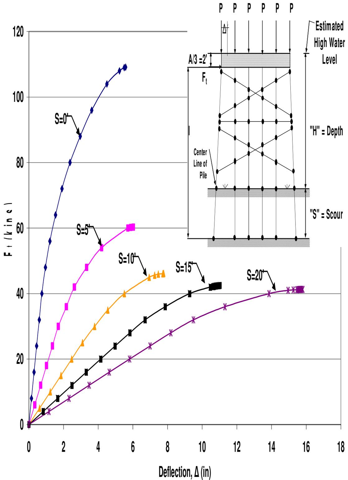
Figure B.97 HP12x53 Two-Story Single X-Braced 6-Pile Bent with  $H=21'$ ,  $P=100$ kips and  $A=6'$  Pushover Analysis Results
