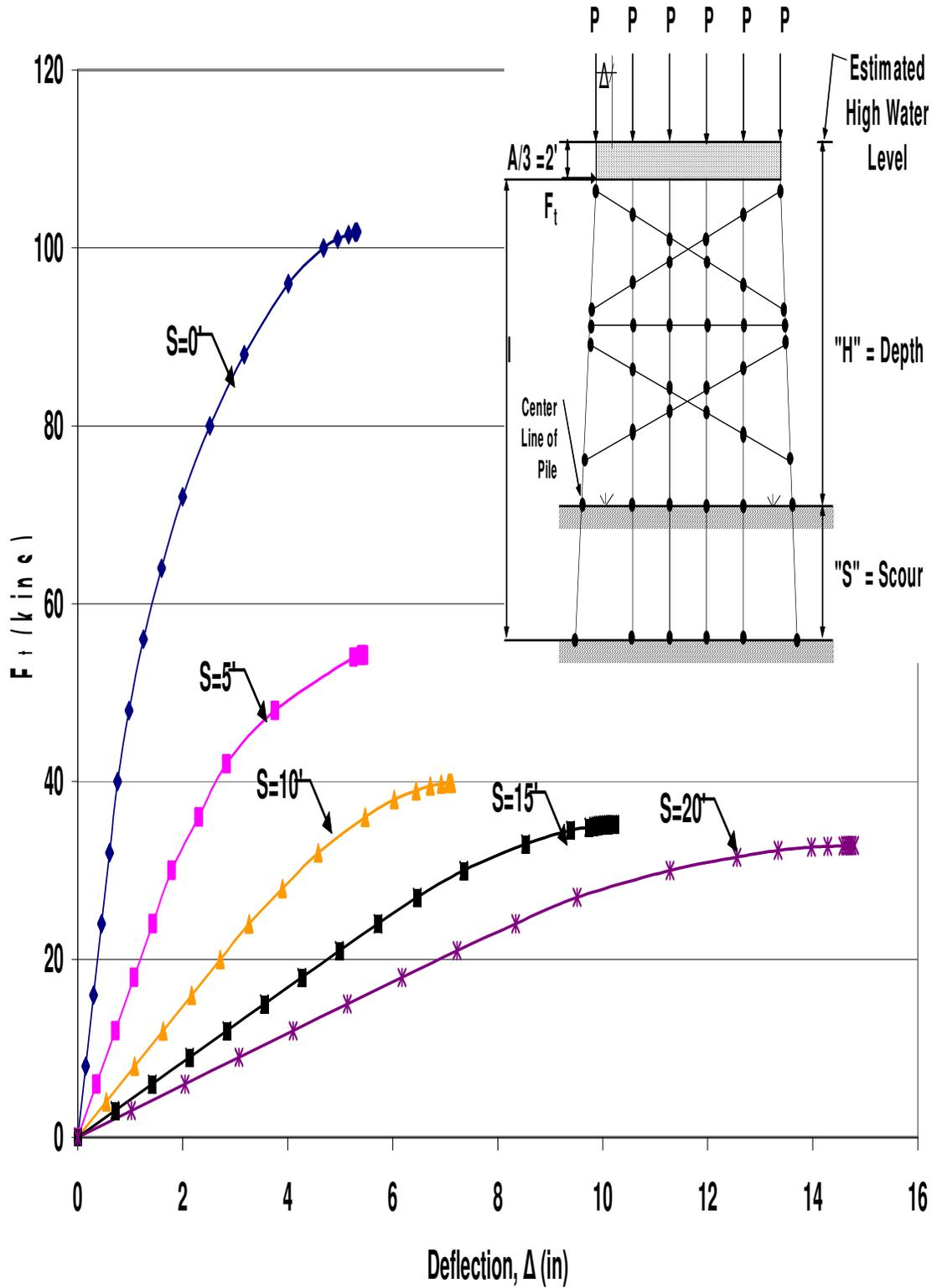
Figure B.98 HP12x53 Two-Story Single X-Braced 6-Pile Bent with  $H=21'$ ,  $P=120$ kips and  $A=6'$  Pushover Analysis Results
