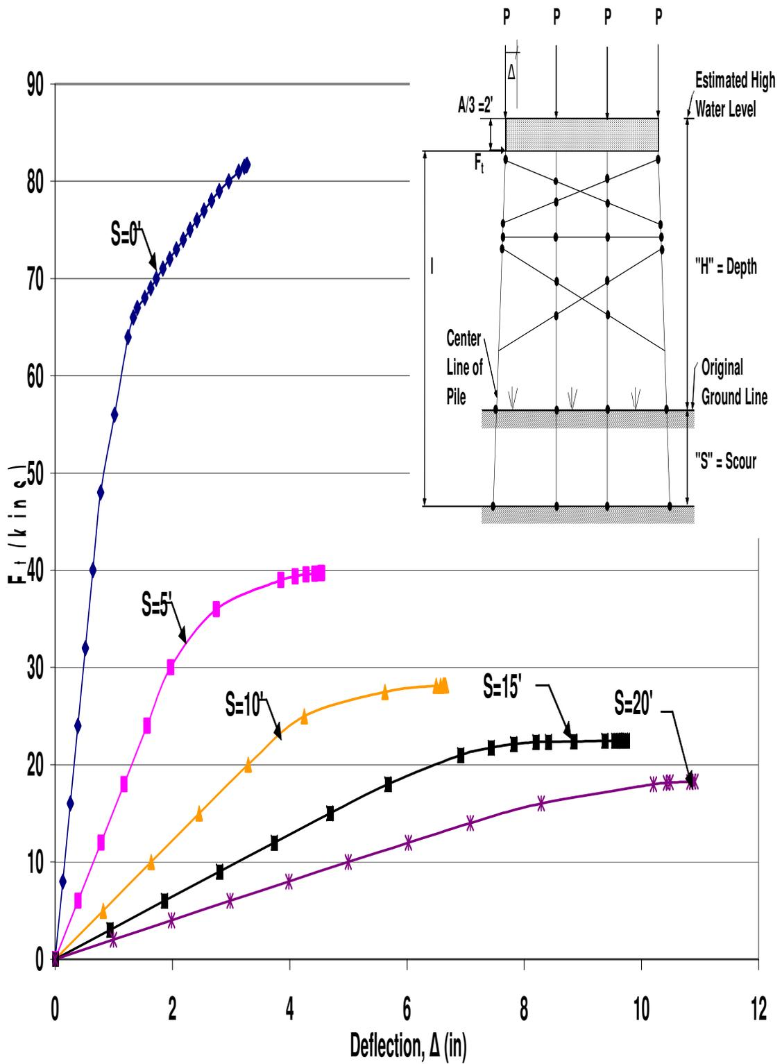
Figure B.45 HP12x53 Two-Story X-Braced 4-Pile Bent with  $H=25'$ ,  $P=100$  kips and  $A=6'$
