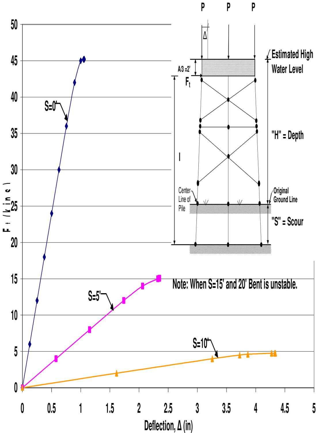
Figure A.21 HP10x42 Two-Story X-Braced 3-Pile Bent with  $H=25'$ ,  $P=100$ kips, and  $A=6'$
