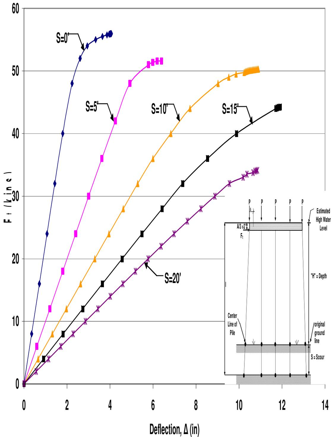
Figure B.53 HP12x53 Unbraced 5-Pile Bent with  $H=13'$ ,  $P=100$ kips and  $A=6'$
