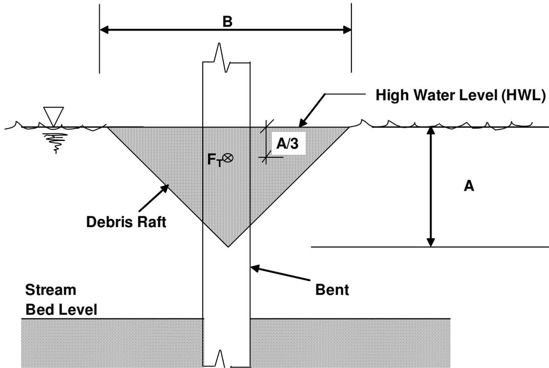
Figure 2.4 Debris Raft for Bent Design (AASHTO 1997)
