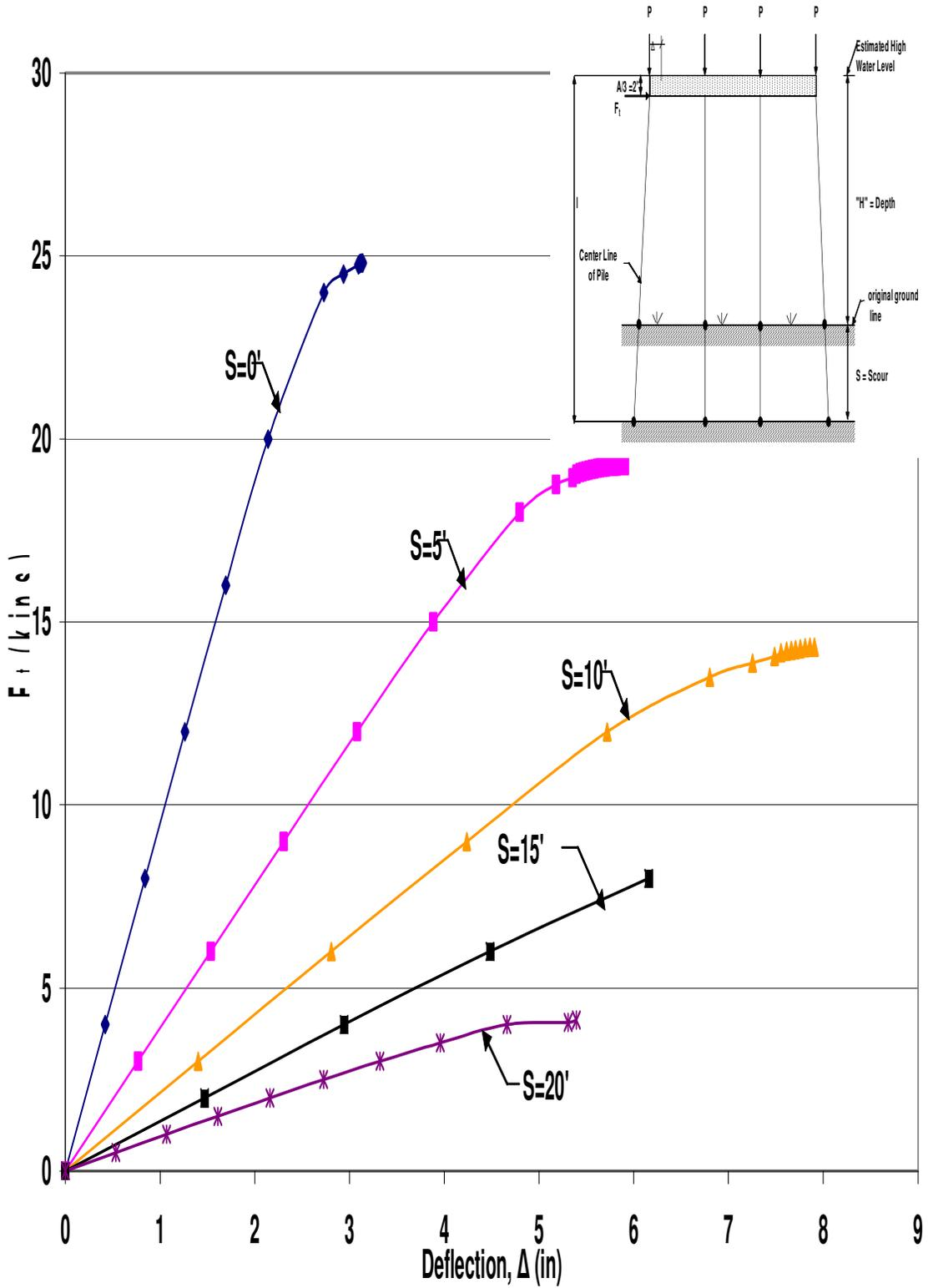
Figure A.31 HP10x42 Unbraced 4-Pile Bent with  $H=13'$ ,  $P=140$ kips and  $A=6'$
