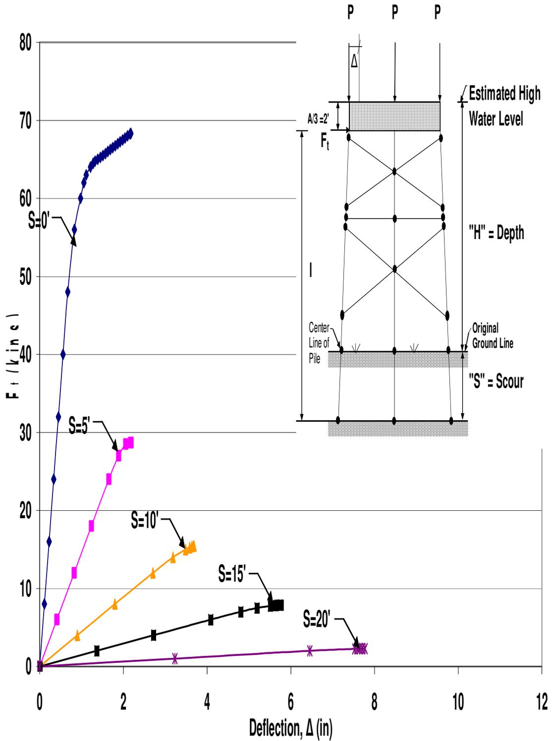
Figure B.21 HP12x53 Two-Story X-Braced 3-Pile Bent with H=25', P=100kips and A=6'
