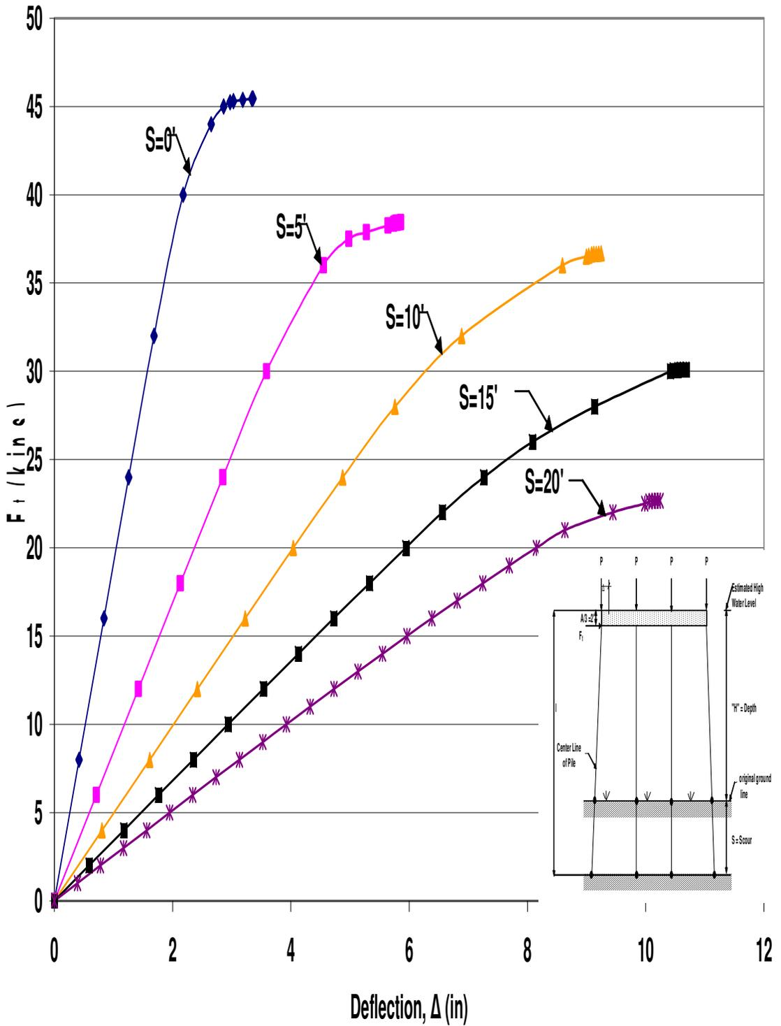
Figure B.29 HP12x53 Unbraced 4-Pile Bent with  $H=13'$ ,  $P=100$ kips, and  $A=6'$
