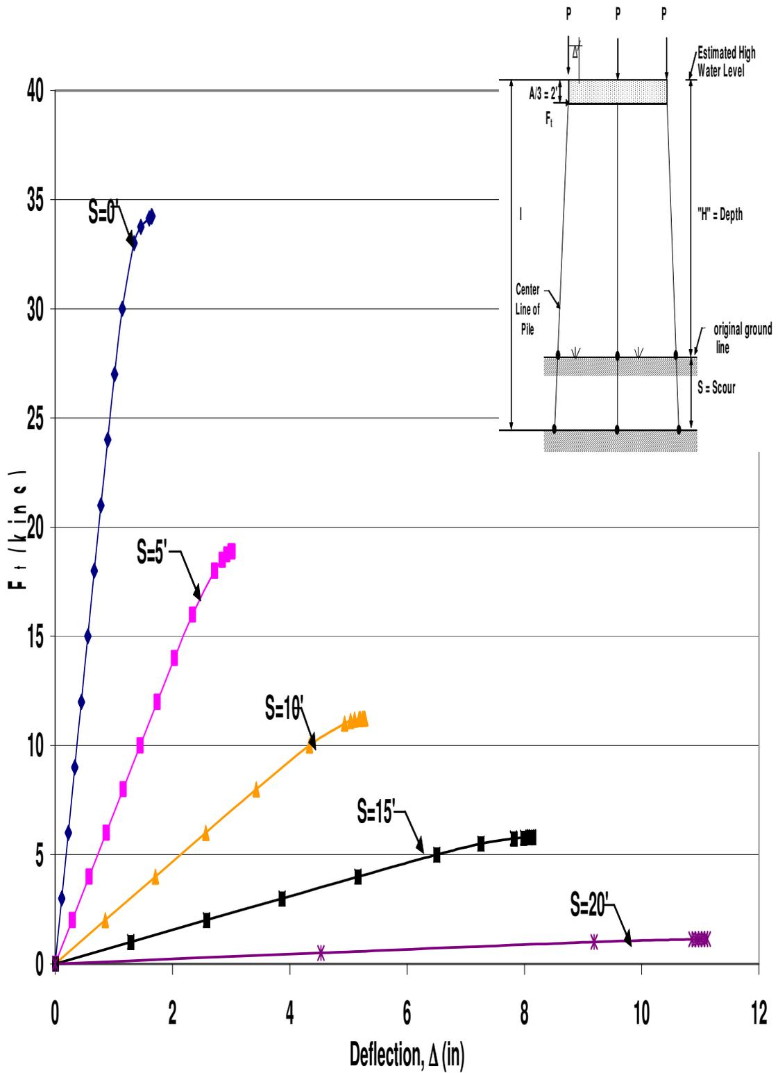
Figure B.2 HP12x53 Unbraced 3-Pile Bent with  $H=10'$ ,  $P=120$ kips and  $A=6'$ ,
