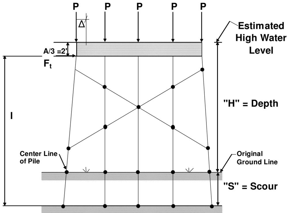
Figure 3.6 Typical X-braced Bent and Typical Loading Conditions
