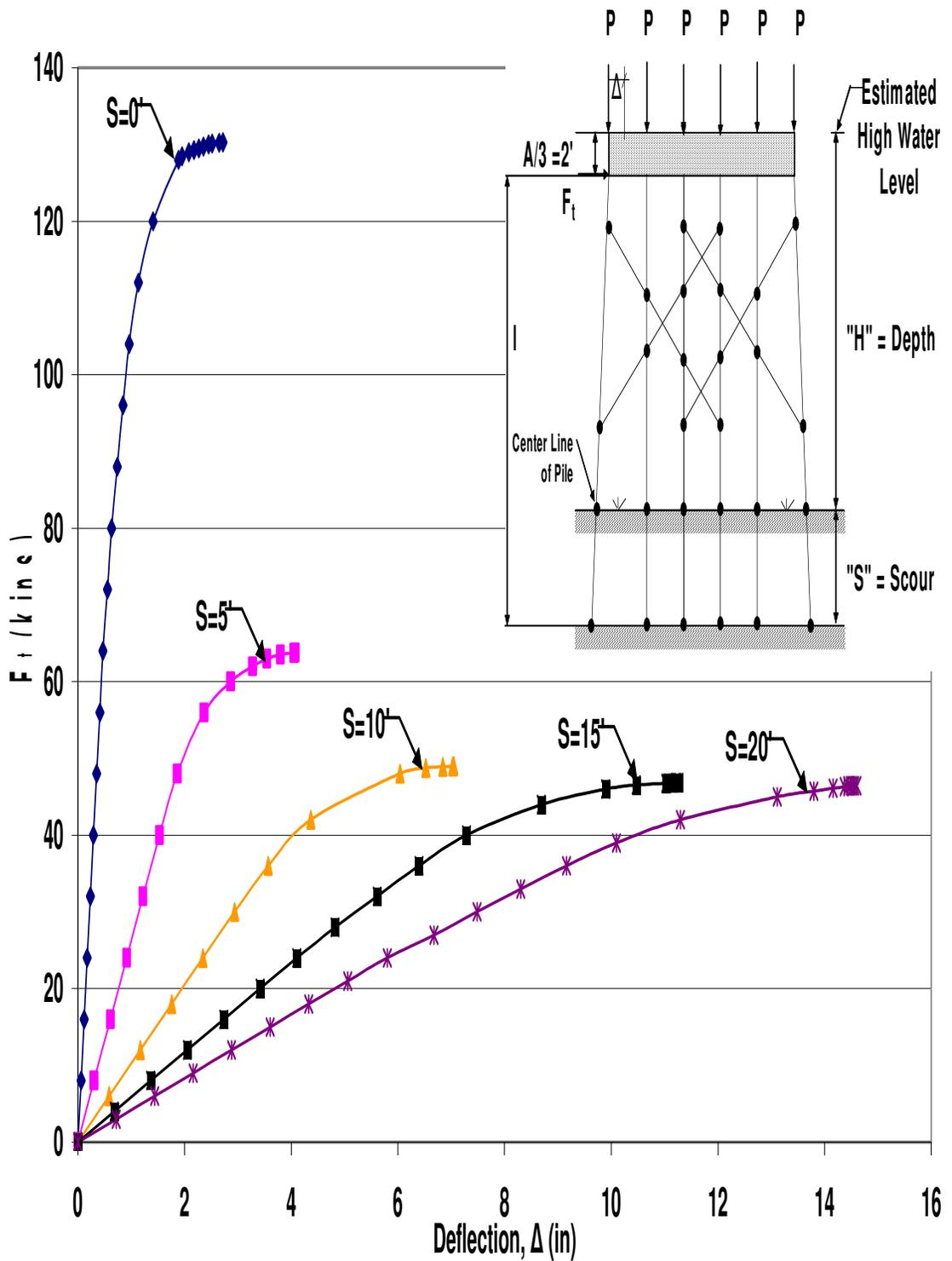
Figure B.89 HP12x53 Double X-Braced 6-Pile Bent with  $H=13'$ ,  $P=100$ kips and  $A=6'$
