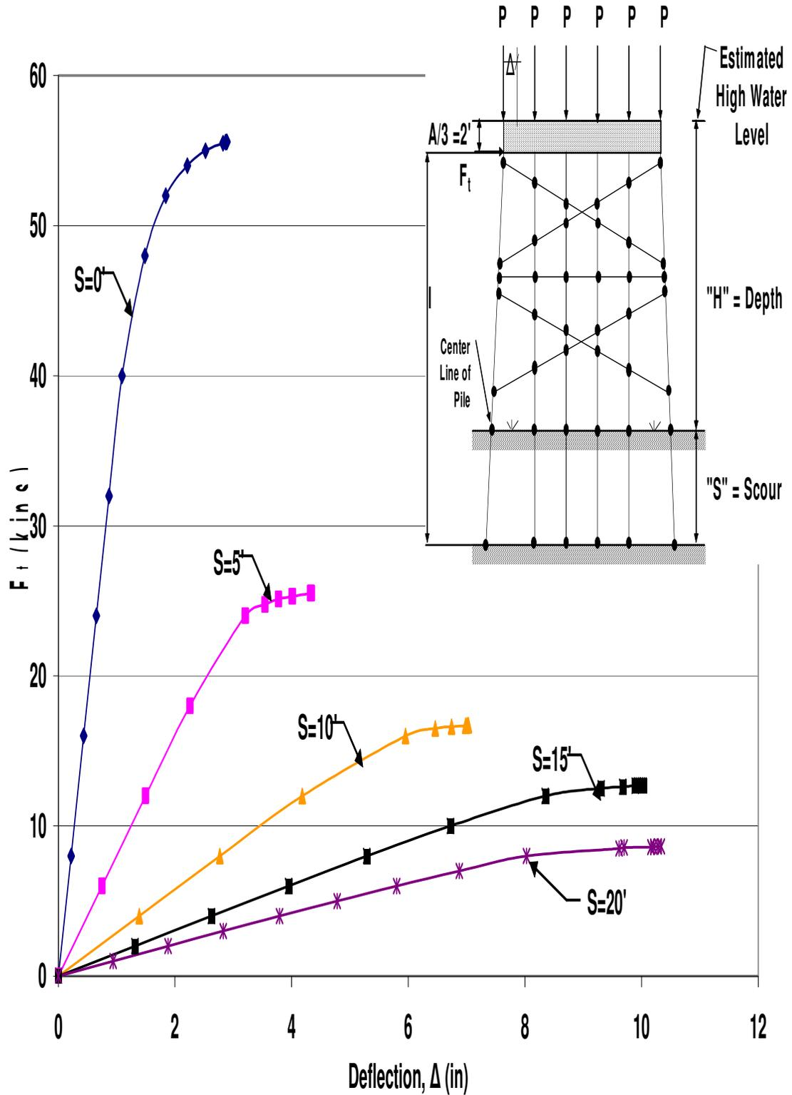
Figure A.102 HP10x42 Two-Story Single X-Braced 6-Pile Bent with  $H=25'$ ,  $P=120$ kips and  $A=6'$  Pushover Analysis Results
