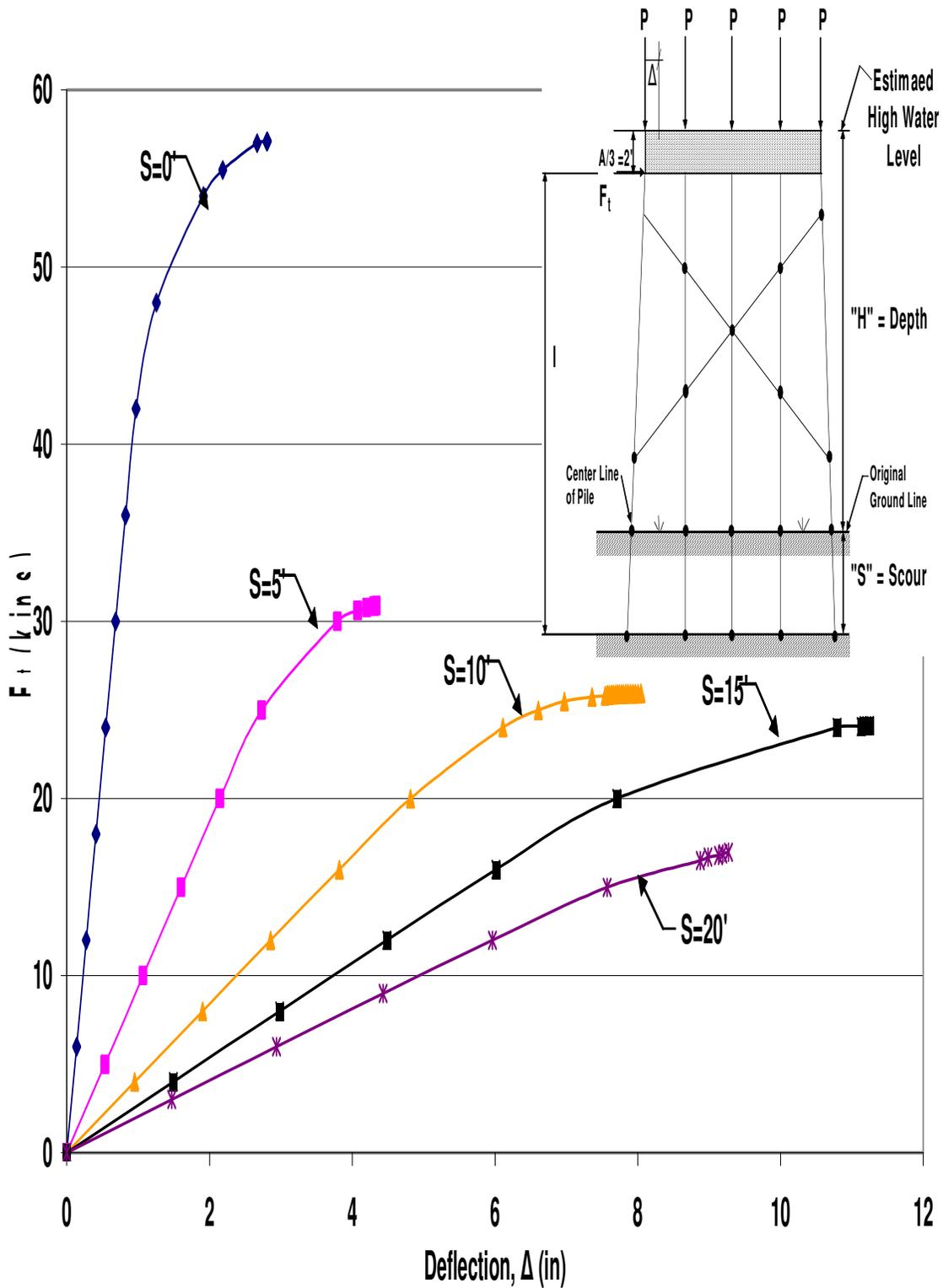
Figure A.61 HP10x42 X-Braced 5-Pile Bent with  $H=17'$ ,  $P=100$  kips and  $A=6'$
