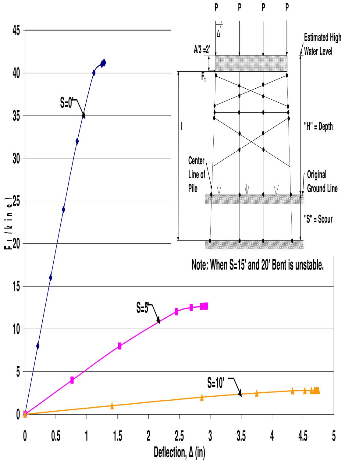
Figure A.48 HP10x42 Two-Story X-Braced 4-Pile Bent with  $H=25'$ ,  $P=160$  kips, and  $A=6'$
