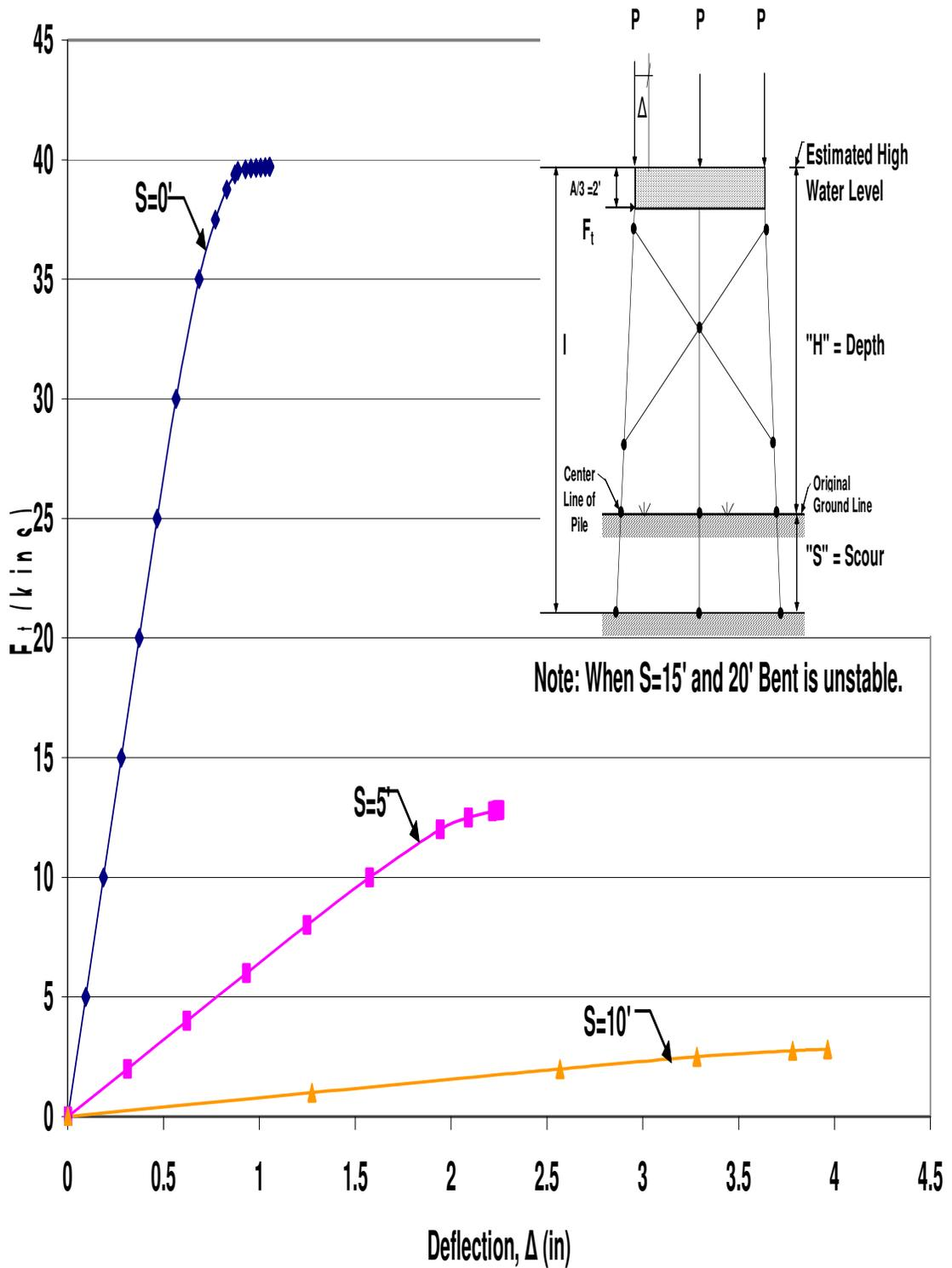
Figure A.11 HP10x42 X-Braced 3-Pile Bent with H=13', P=140kips and A=6'
