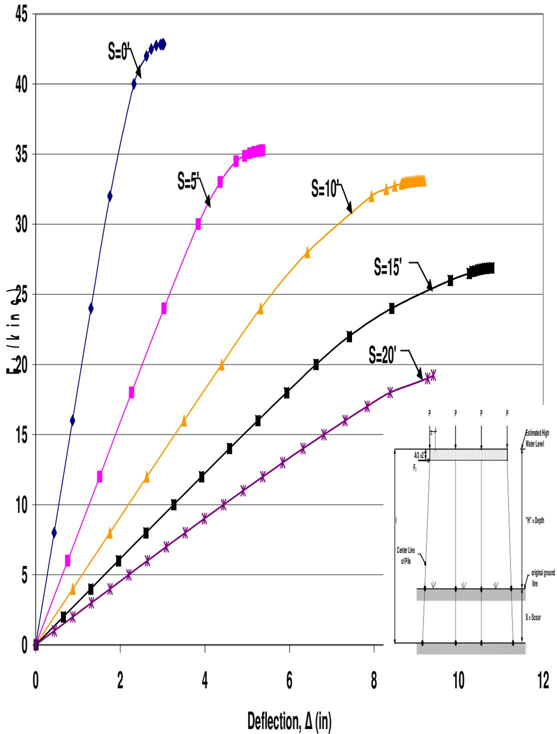
Figure B.30 HP12x53 Unbraced 4-Pile Bent with H=13', P=120kips, and A=6'
