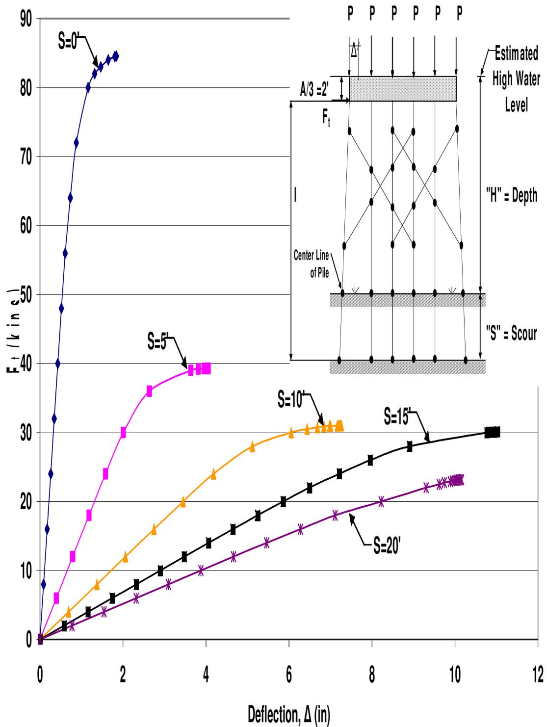
Figure A.89 HP10x42 Double X-Braced 6-Pile Bent with  $H=13'$ ,  $P=100$  kips and  $A=6'$
