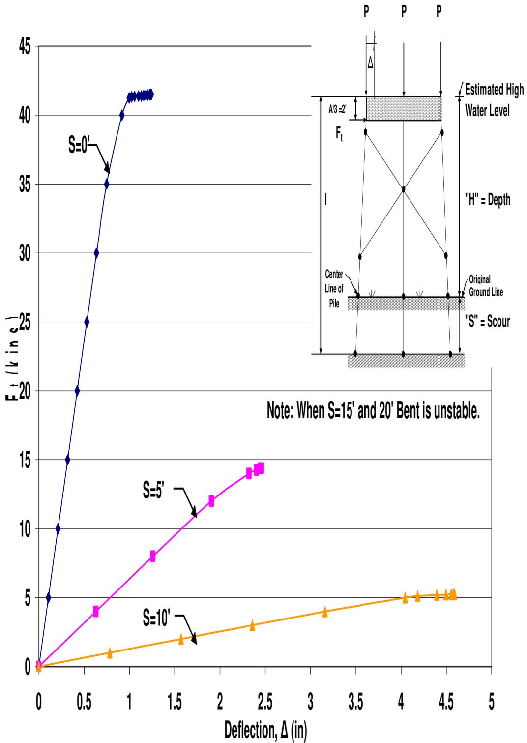
Figure A.13 HP10x42 X-Braced 3-Pile Bent with H=17', P=100kips and A=6'
