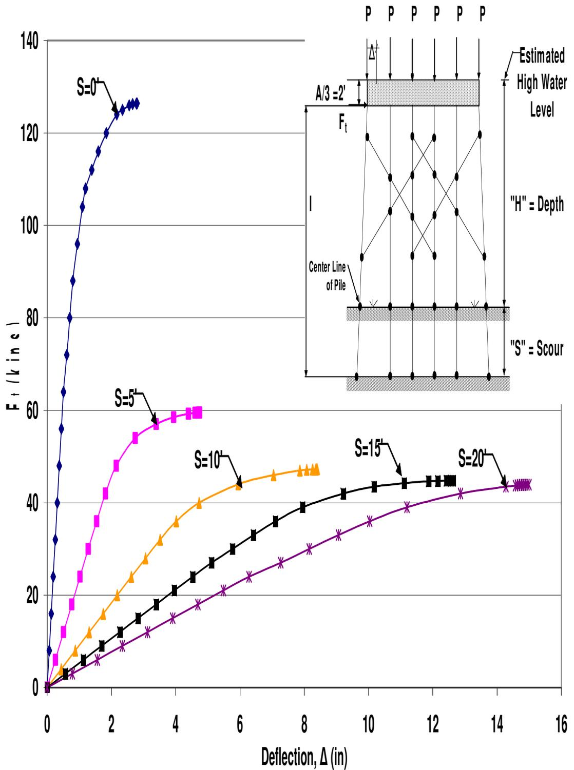
Figure B.93 HP12x53 Double X-Braced 6-Pile Bent with  $H=17'$ ,  $P=100$ kips and  $A=6'$
