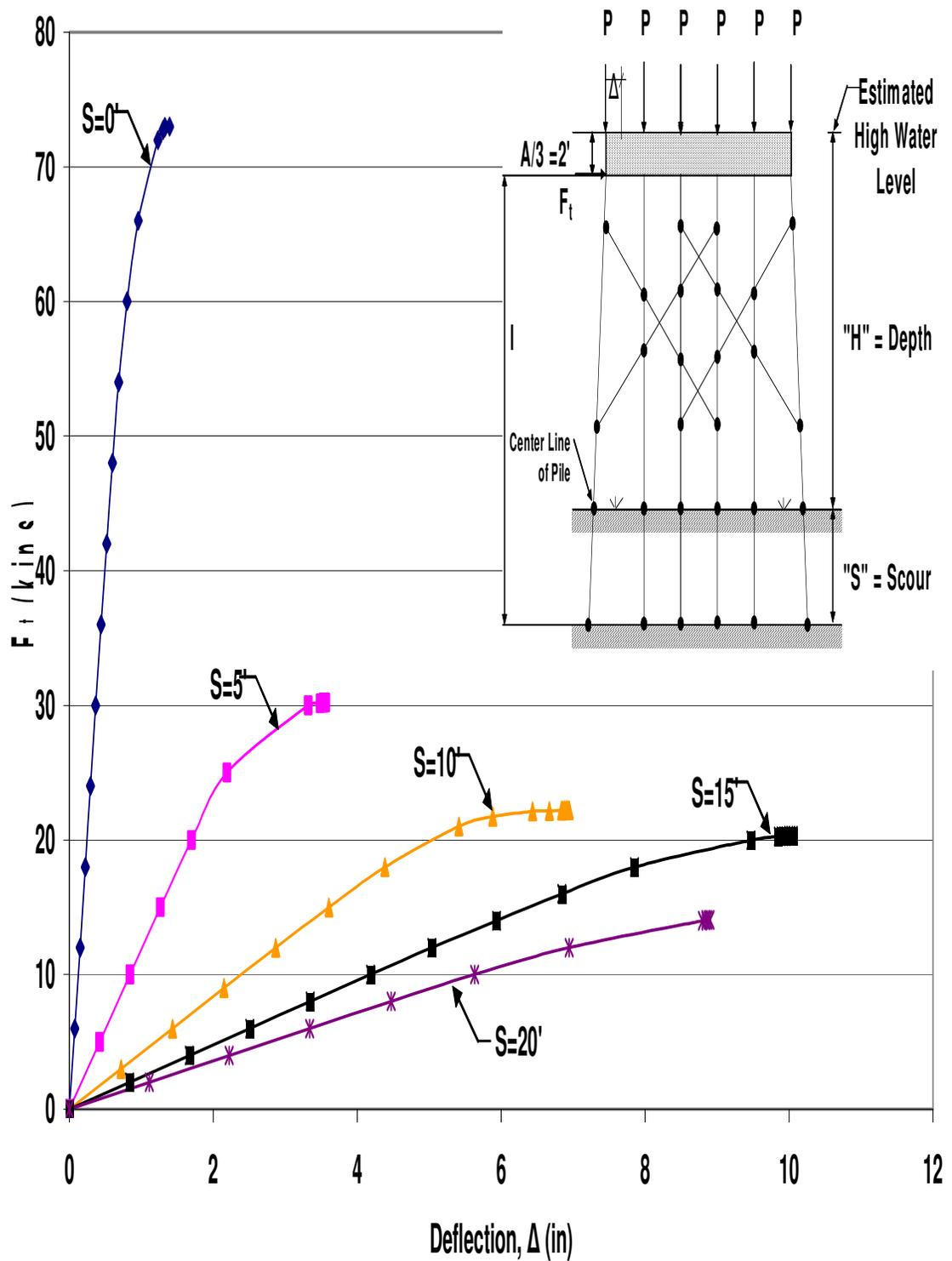
Figure A.94 HP10x42 Double X-Braced 6-Pile Bent with  $H=17'$ ,  $P=120$ kips and  $A=6'$
