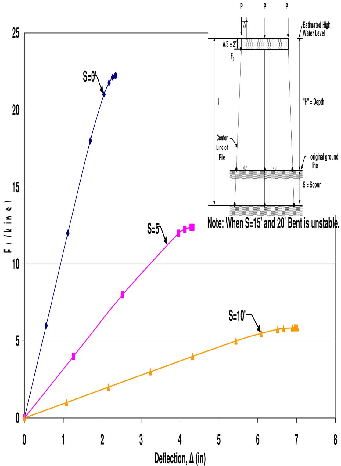
Figure B.7 HP12x53 Unbraced 3-Pile Bent with  $H=13'$ ,  $P=140$  kips and  $A=6'$
