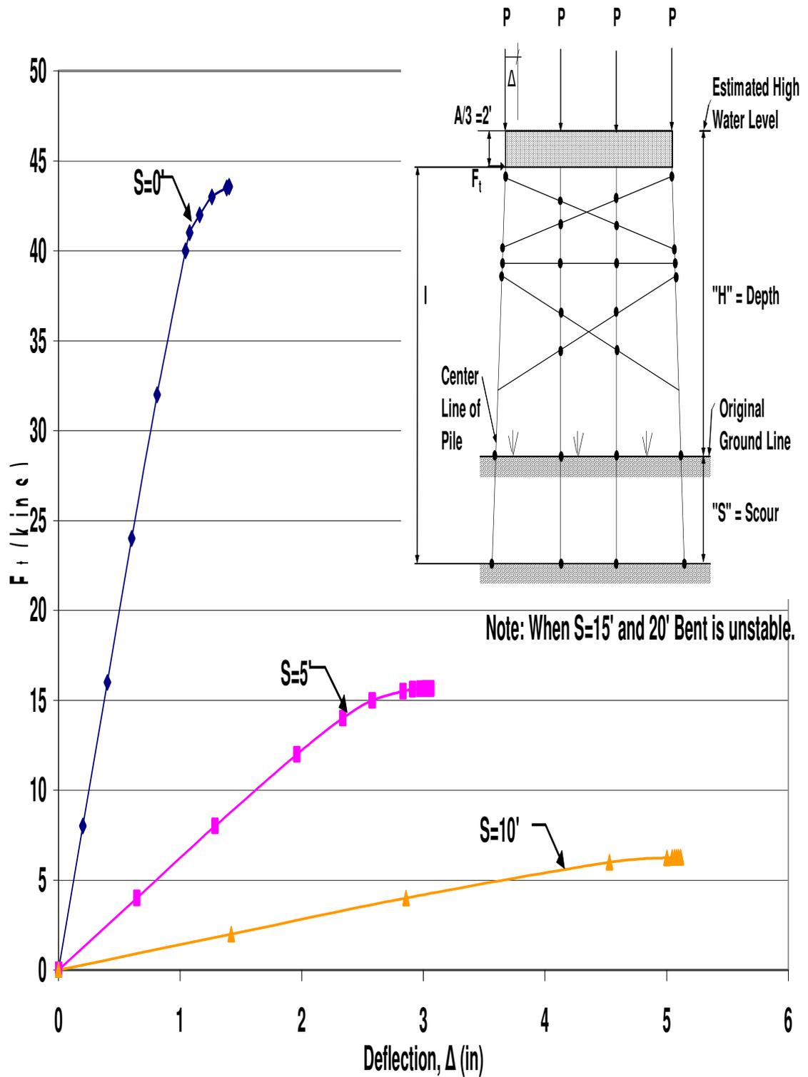
Figure A.47 HP10x42 Two-Story X-Braced 4-Pile Bent with  $H=25'$ ,  $P=140$ kips, and  $A=6'$
