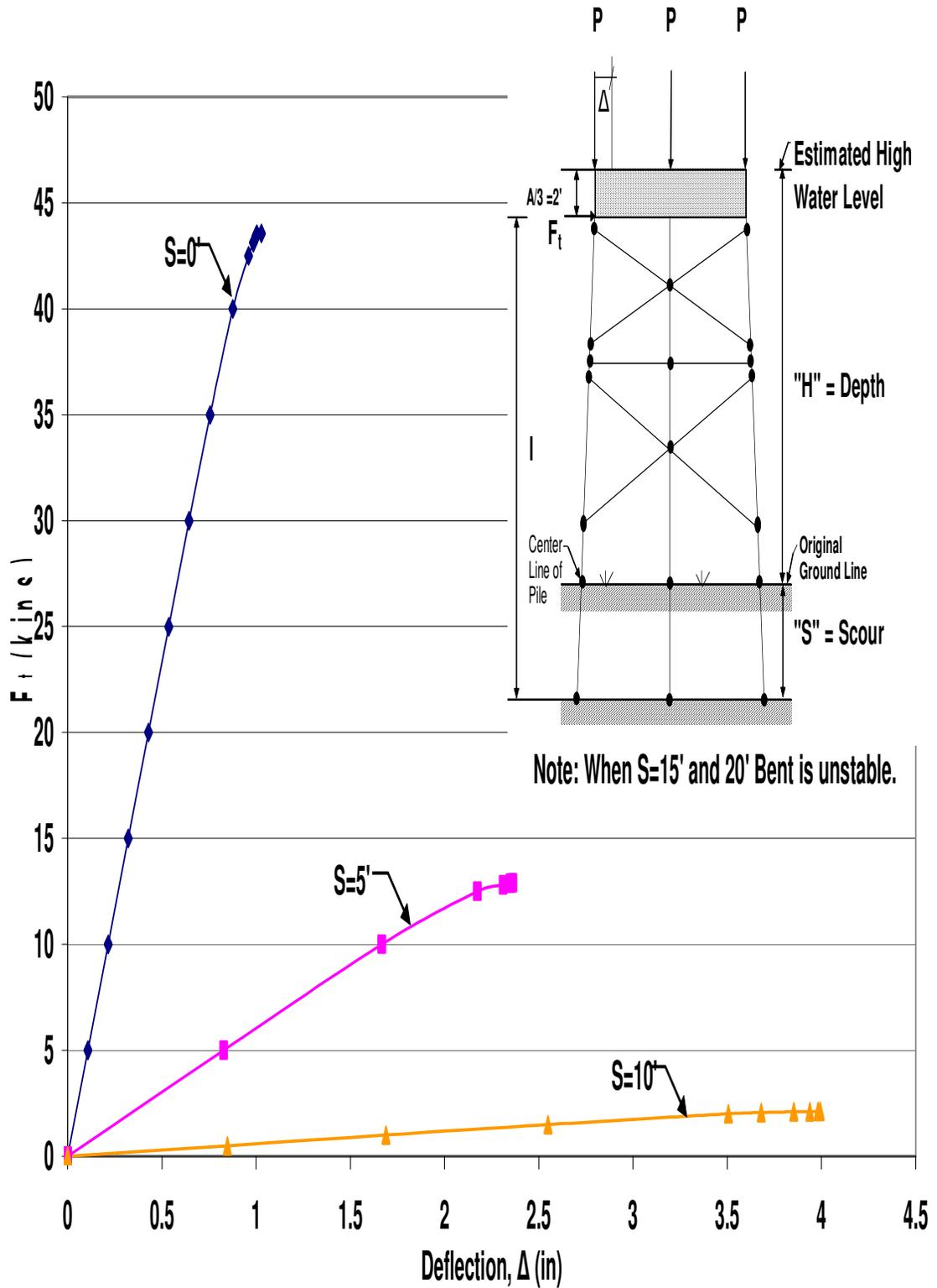
Figure A.22 HP10x42 Two-Story X-Braced 3-Pile Bent with H=25', P=120kips, and A=6'
