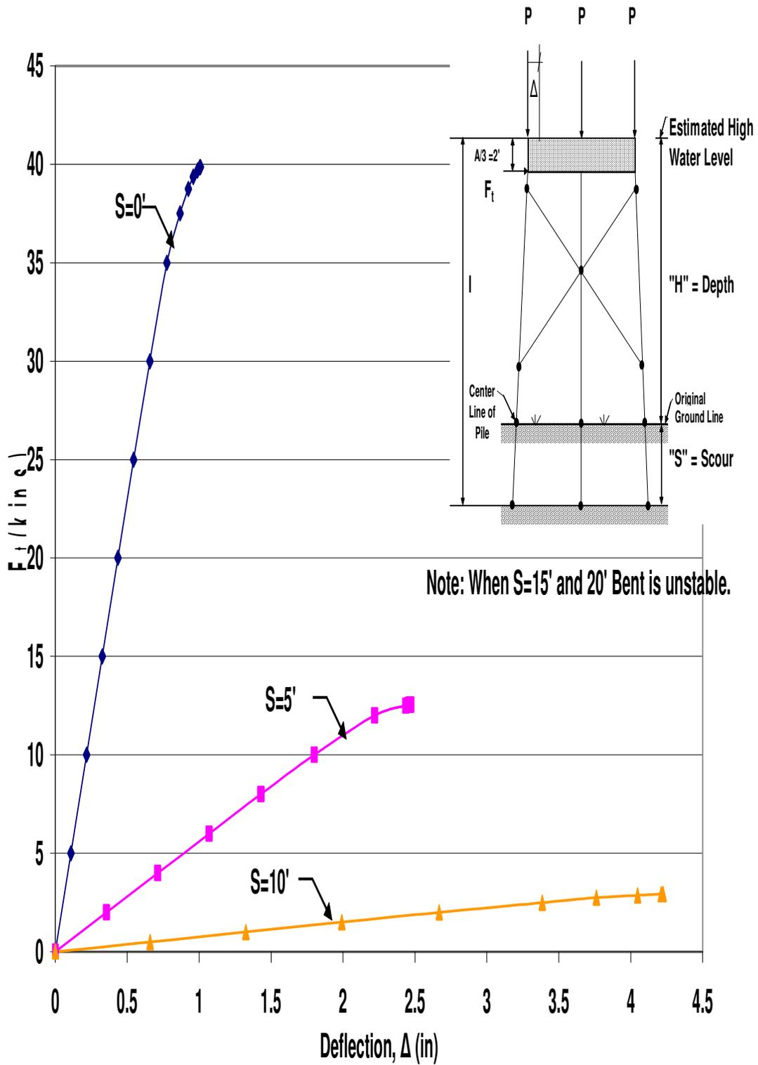
Figure A.14 HP10x42 X-Braced 3-Pile Bent with H=17', P=120kips and A=6'
