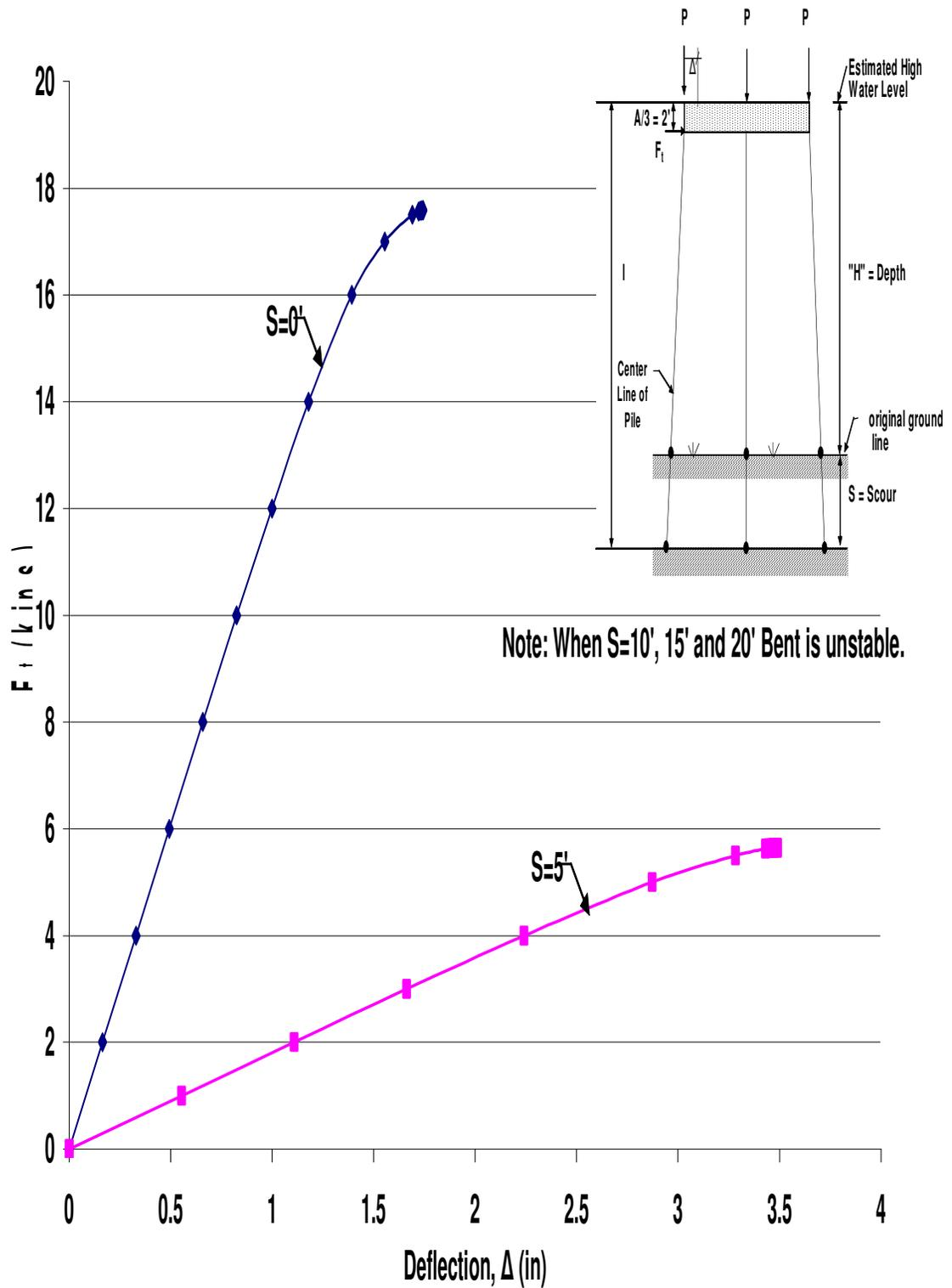
Figure A.4 HP10x42 Unbraced 3-Pile Bent with H=10', P=160kips, and A=6'
