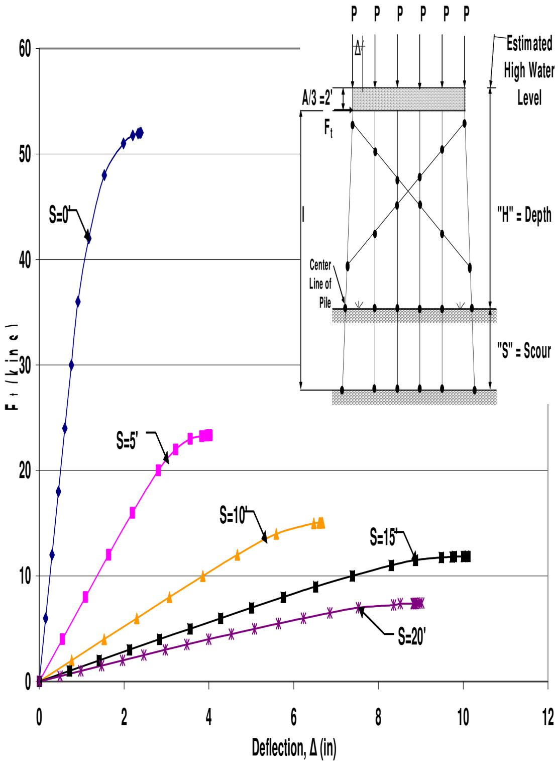
Figure A.87 HP10x42 Single X-Braced 6-Pile Bent with  $H=17'$ ,  $P=140$  kips and  $A=6'$
