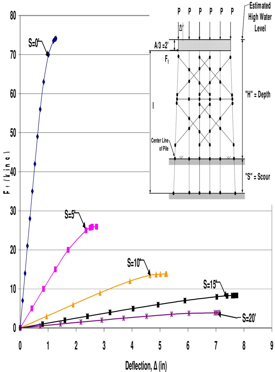
Figure A.108 HP10x42 Two-Story Double X-Braced 6-Pile Bent with  $H=21'$ ,  $P=160$ kips and  $A=6'$  Pushover Analysis Results
