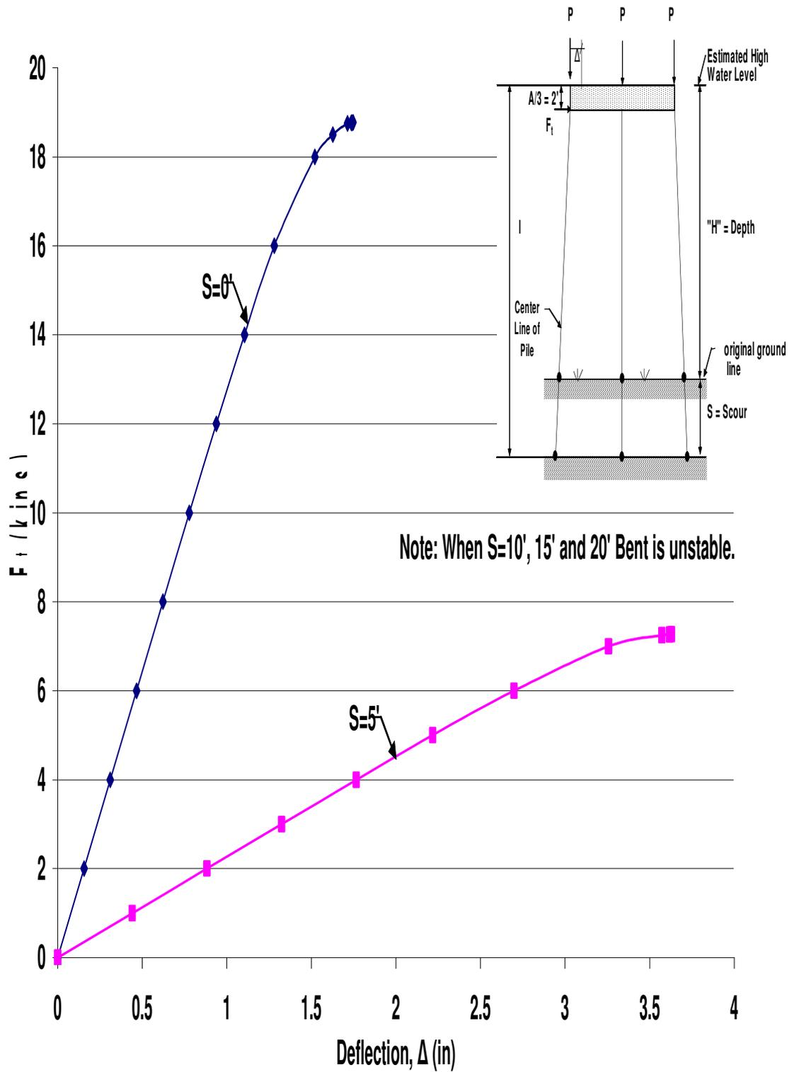
Figure A.3 HP10x42 Unbraced 3-Pile Bent with H=10', P=140kips, and A=6'
