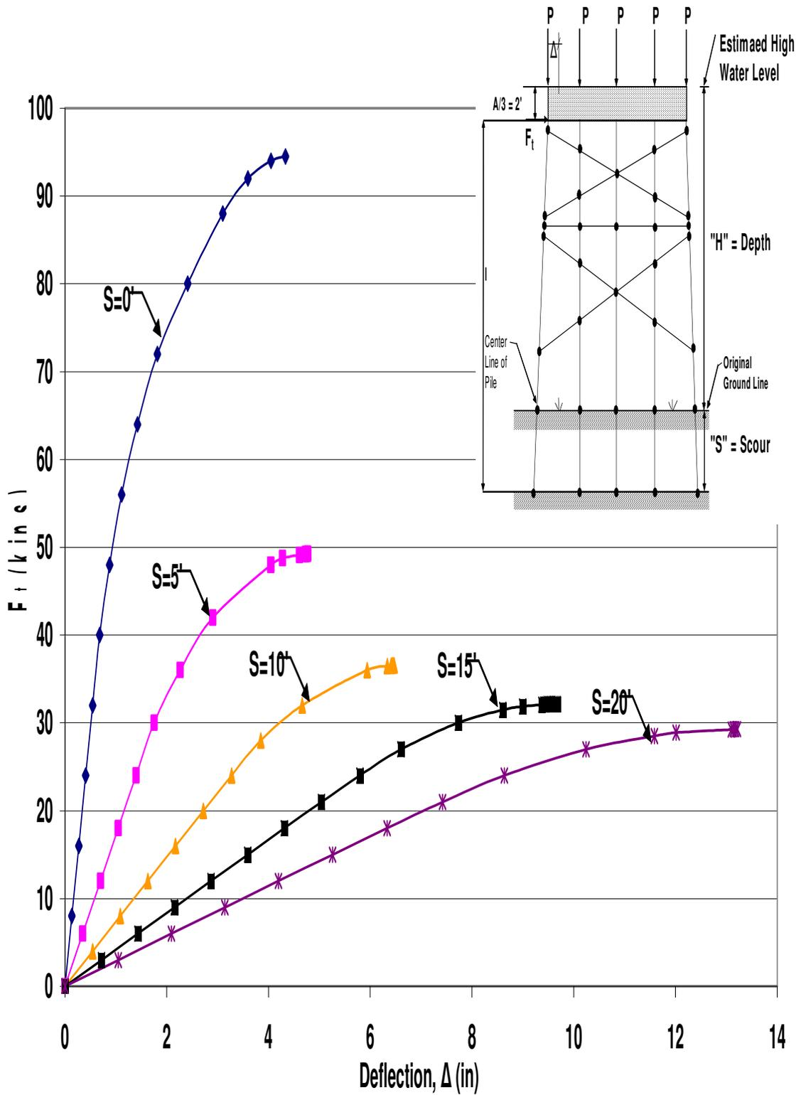
Figure B.66 HP12x53 Two-Story X-Braced 5-Pile Bent with  $H=21'$ ,  $P=120$ kips and  $A=6'$
