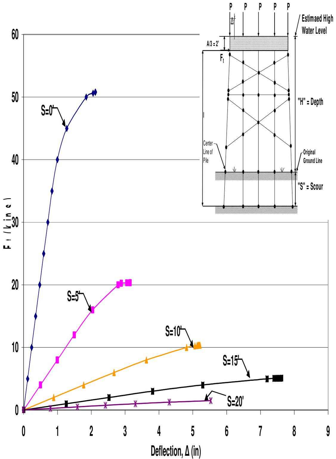
Figure A.68 HP10x42 Two-Story X-Braced 5-Pile Bent with H=21', P=160kips and A=6'
