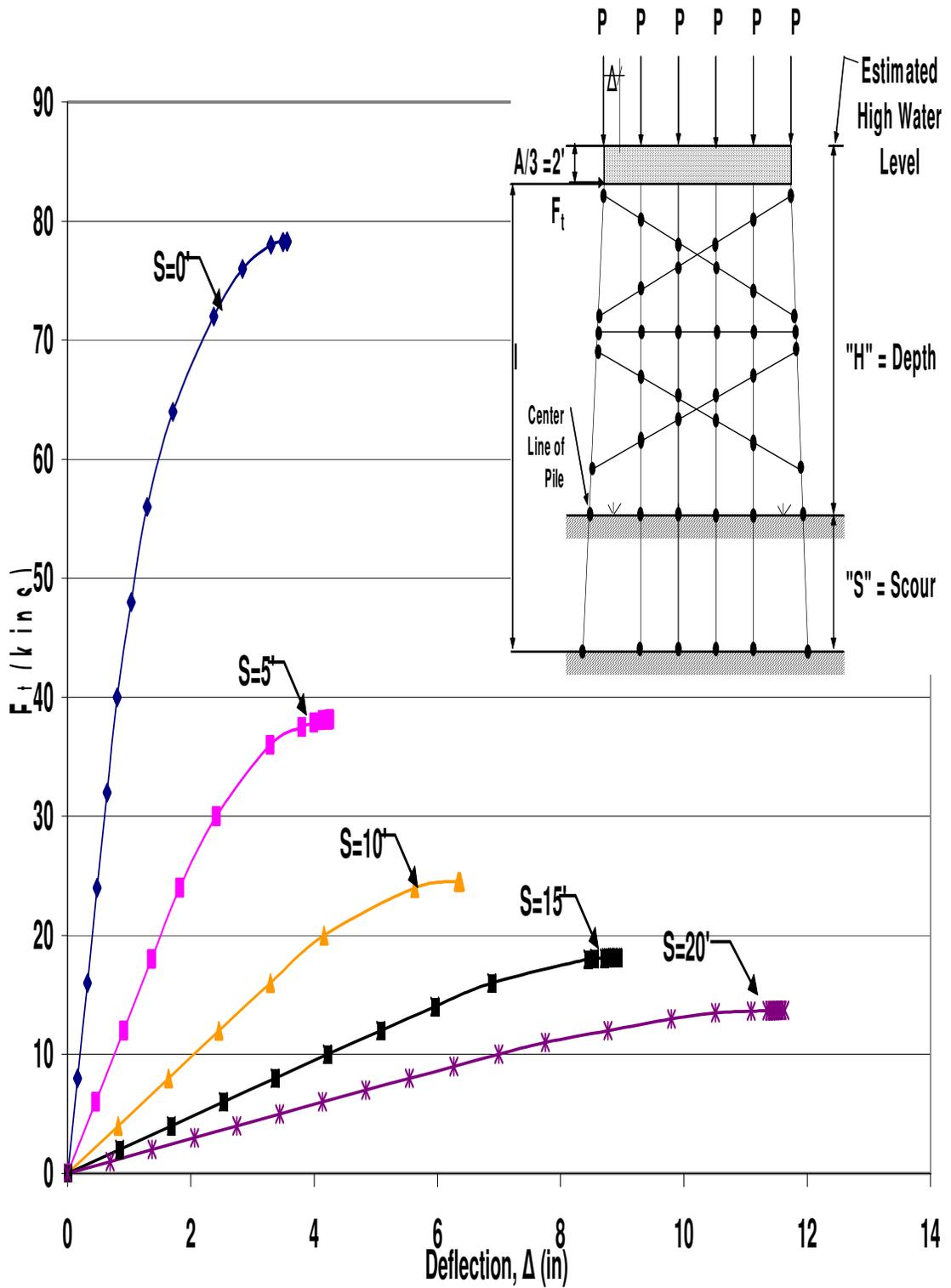
Figure B.104 HP12x53 Two-Story Single X-Braced 6-Pile Bent with  $H=25'$ ,  $P=160$ kips and  $A=6'$  Pushover Analysis Results
