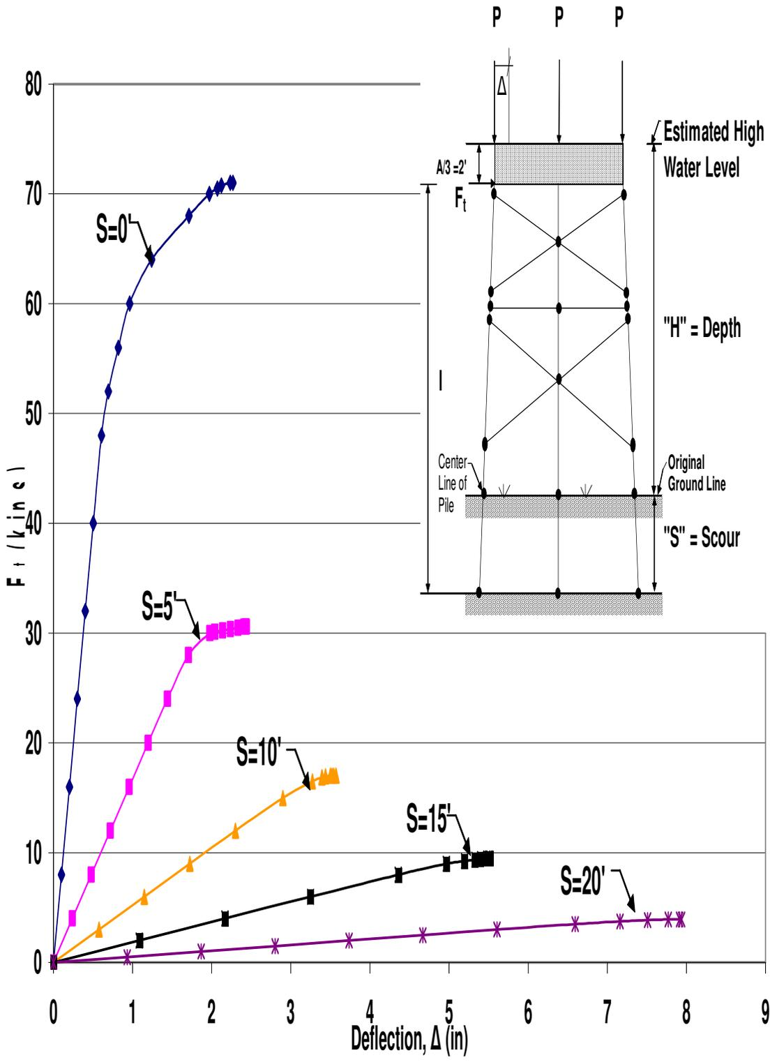
Figure B.17 HP12x53 Two-Story X-Braced 3-Pile Bent with  $H=21'$ ,  $P=100$ kips and  $A=6'$
