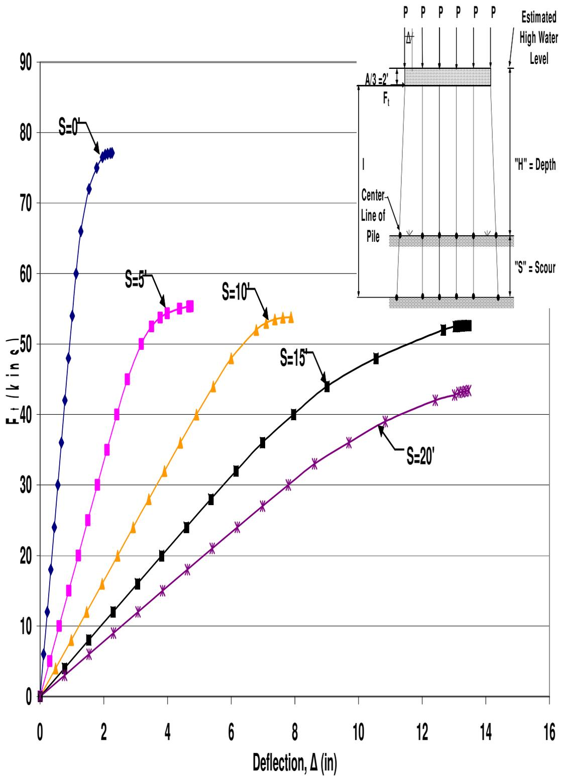
Figure B.73 HP12x53 Unbraced 6-Pile Bent with  $H=10'$ ,  $P=100$ kips and  $A=6'$
