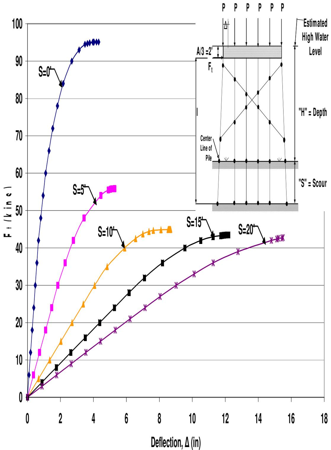
Figure B.85 HP12x53 Single X-Braced 6-Pile Bent with  $H=17'$ ,  $P=100$ kips and  $A=6'$
