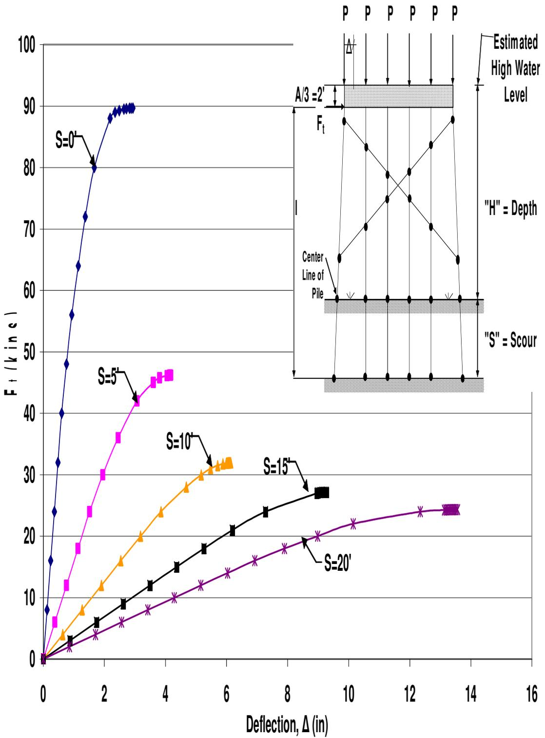
Figure B.84 HP12x53 Single X-Braced 6-Pile Bent with  $H=13'$ ,  $P=160$ kips and  $A=6'$
