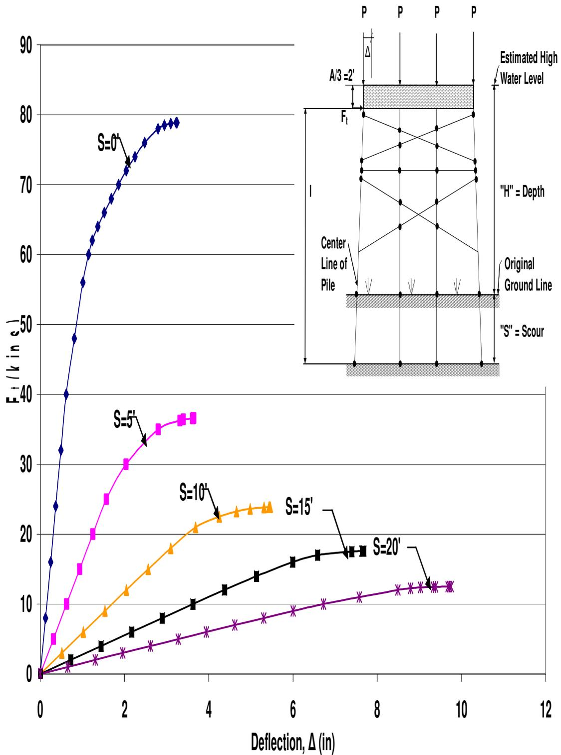
Figure B.43 HP12x53 Two-Story X-Braced 4-Pile Bent with  $H=21'$ ,  $P=140$ kips and  $A=6'$
