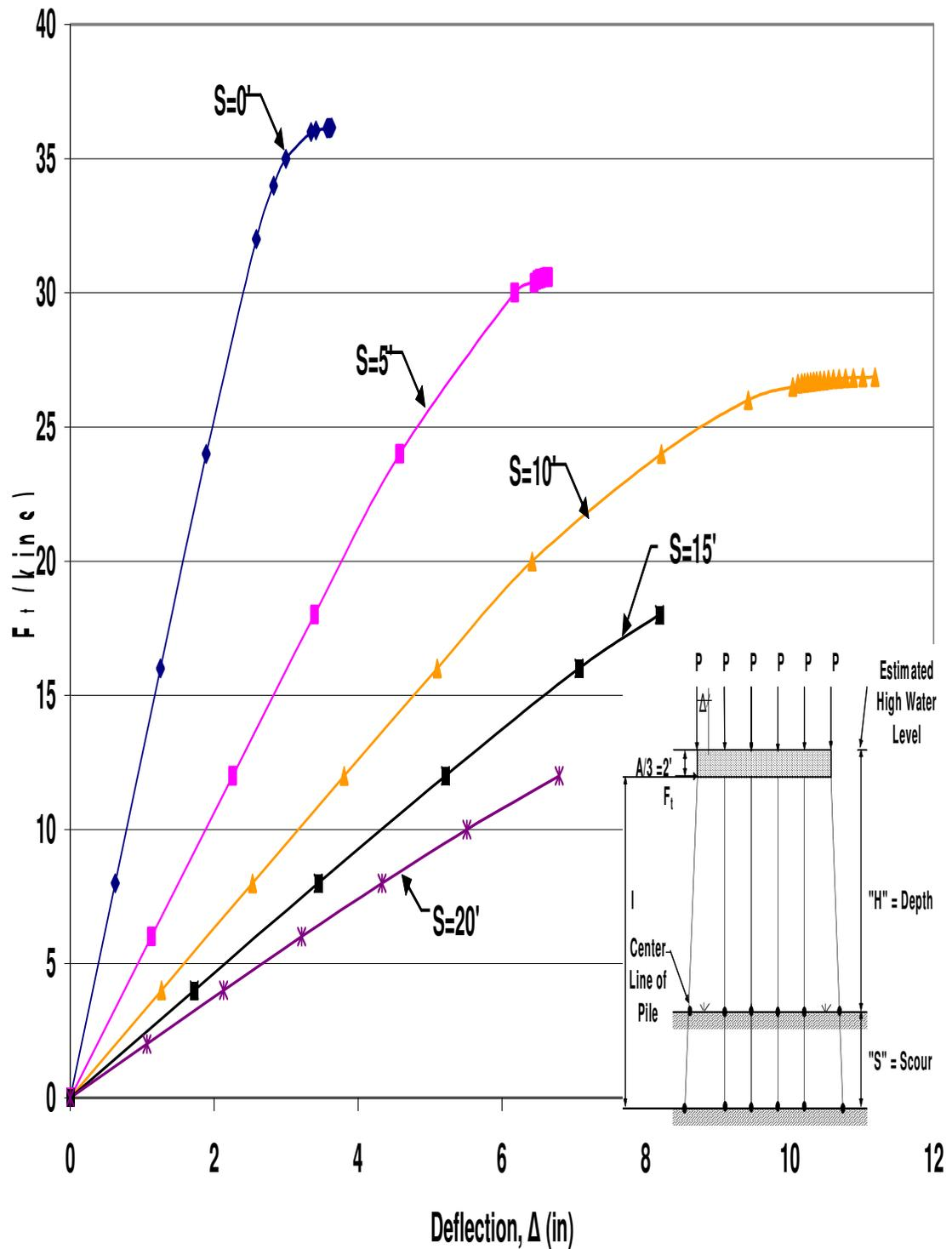
Figure A.78 HP10x42 Unbraced 6-Pile Bent with  $H=13'$ ,  $P=120$  kips and  $A=6'$
