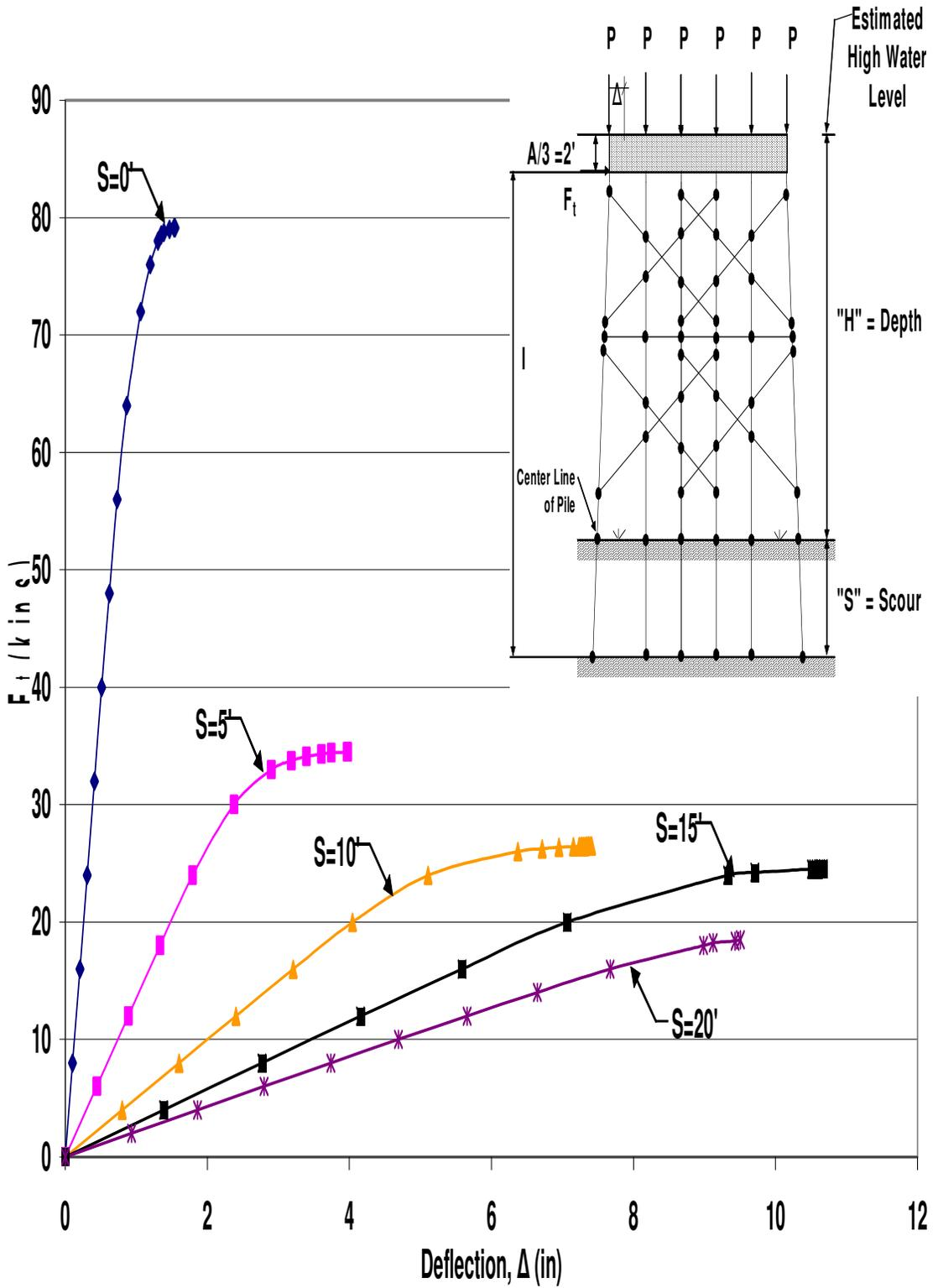
Figure A.109 HP10x42 Two-Story Double X-Braced 6-Pile Bent with  $H=25'$ ,  $P=100$  kips and  $A=6'$  Pushover Analysis Results
