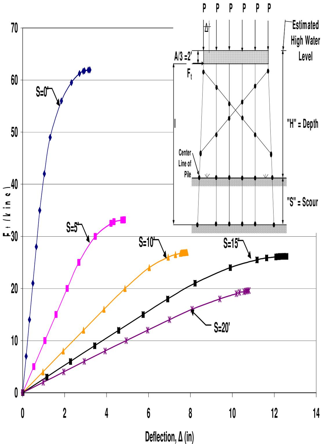
Figure A.85 HP10x42 Single X-Braced 6-Pile Bent with  $H=17'$ ,  $P=100$ kips and  $A=6'$
