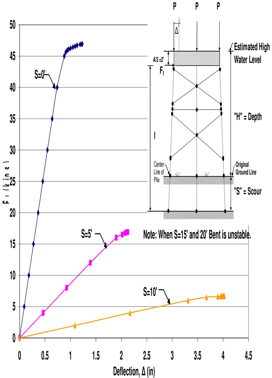
Figure A.17 HP10x42 Two-Story X-Braced 3-Pile Bent with  $H=21'$ ,  $P=100$ kips, and  $A=6'$
