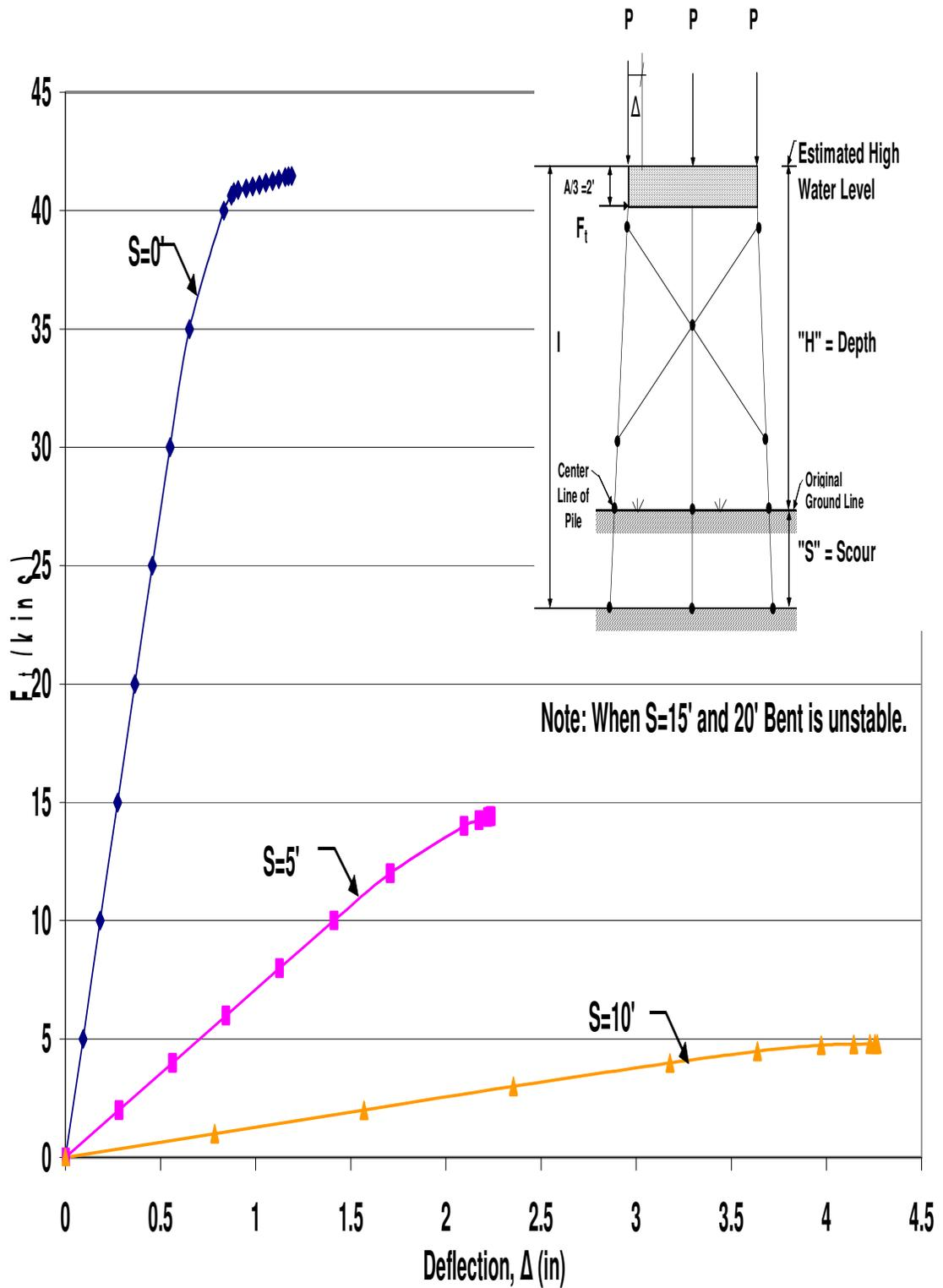
Figure A.10 HP10x42 X-Braced 3-Pile Bent with H=13', P=120kips and A=6'
