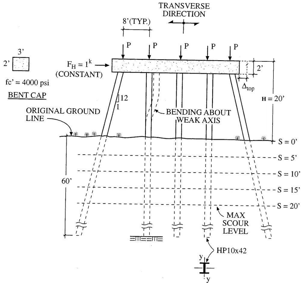
Figure 2.14 Pile Bent Analyzed to Determine  $P-\Delta_{top}$  Curve in Transverse Direction
