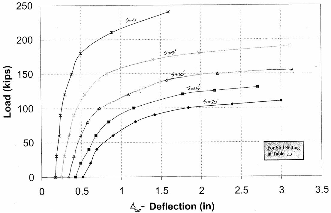
Figure 2.15 P- $\Delta_{top}$  Curves in Transverse Direction for HP10x42 Pile Bent in Figure 2.14 (Brown and Ramey 2003)
