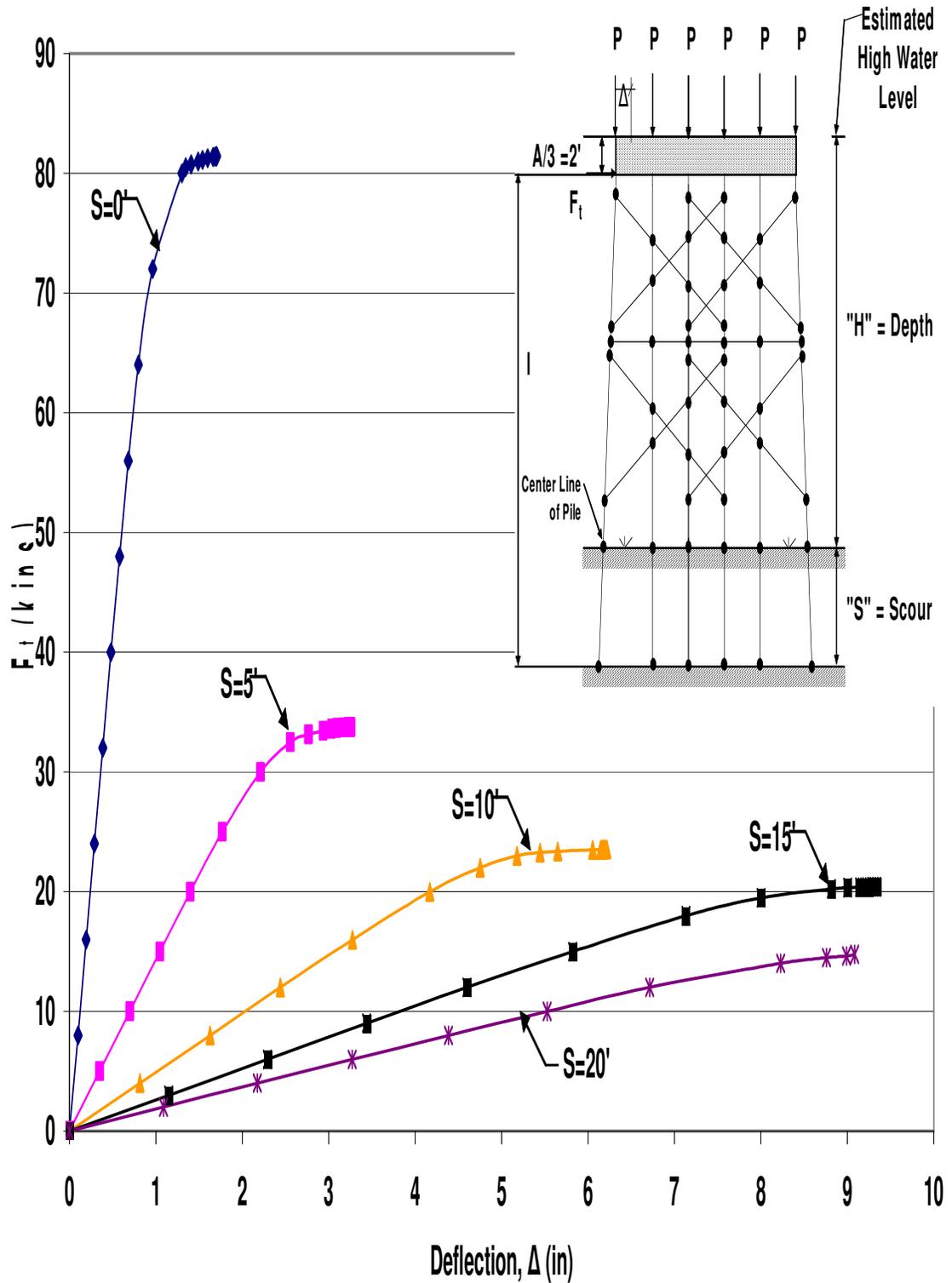
Figure A.106 HP10x42 Two-Story Double X-Braced 6-Pile Bent with  $H=21'$ ,  $P=120$ kips and  $A=6'$  Pushover Analysis Results
