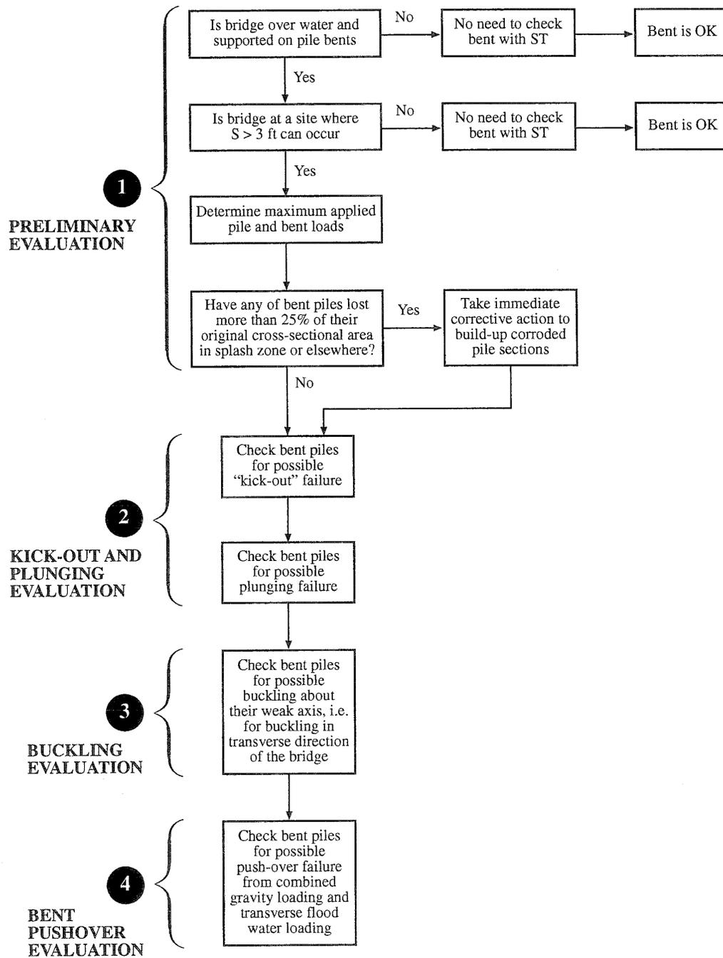
Fig. 6.1. Screening Tool (ST) Macro Flowchart
