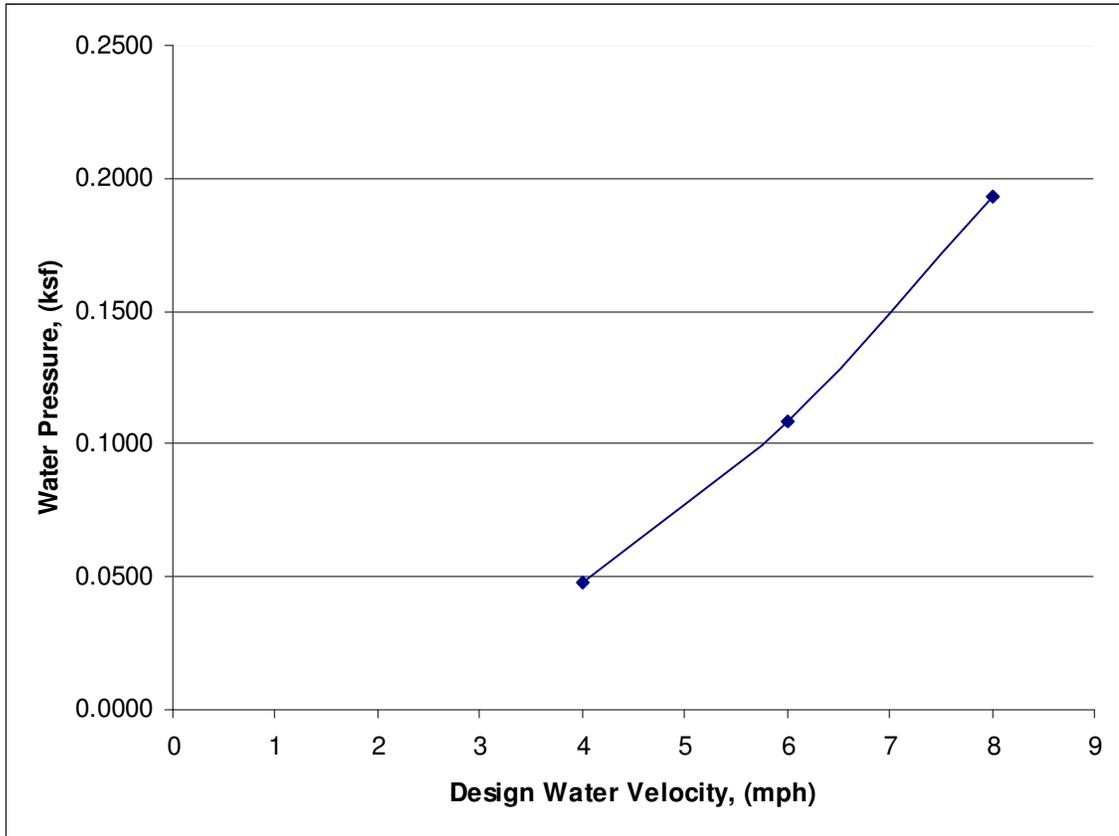
Figure 2.3 Relationship Between Water Pressure and Design Water Velocity for  $C_D = 1.4$
