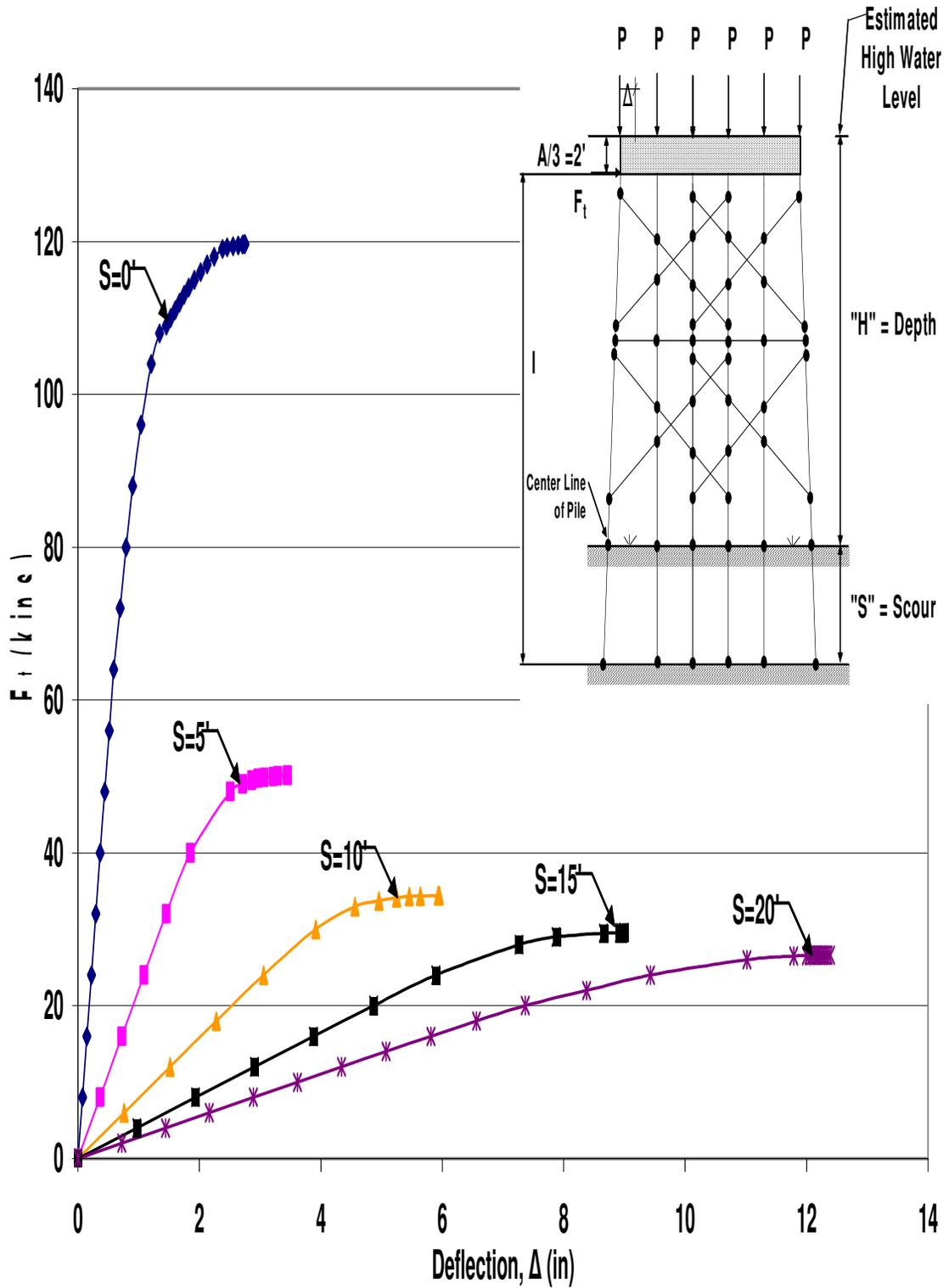
Figure B.111 HP12x53 Two-Story Double X-Braced 6-Pile Bent with  $H=25'$ ,  $P=140$ kips and  $A=6'$  Pushover Analysis Results
