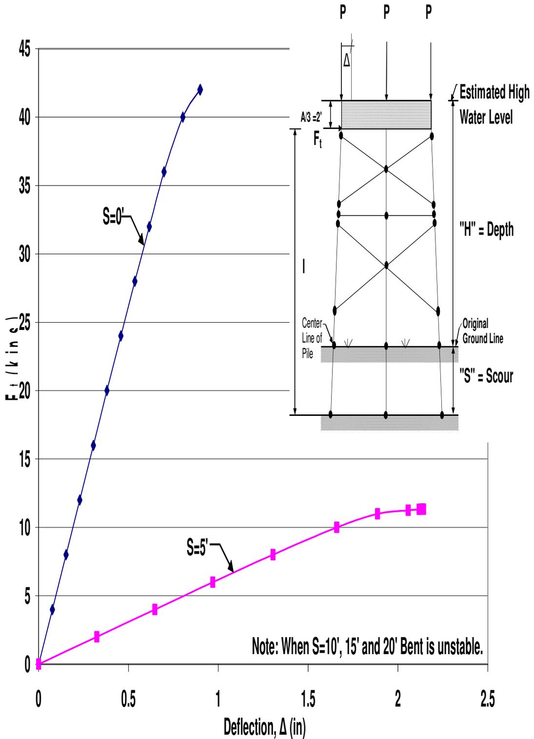
Figure A.20 HP10x42 Two-Story X-Braced 3-Pile Bent with  $H=21'$ ,  $P=160$ kips, and  $A=6'$
