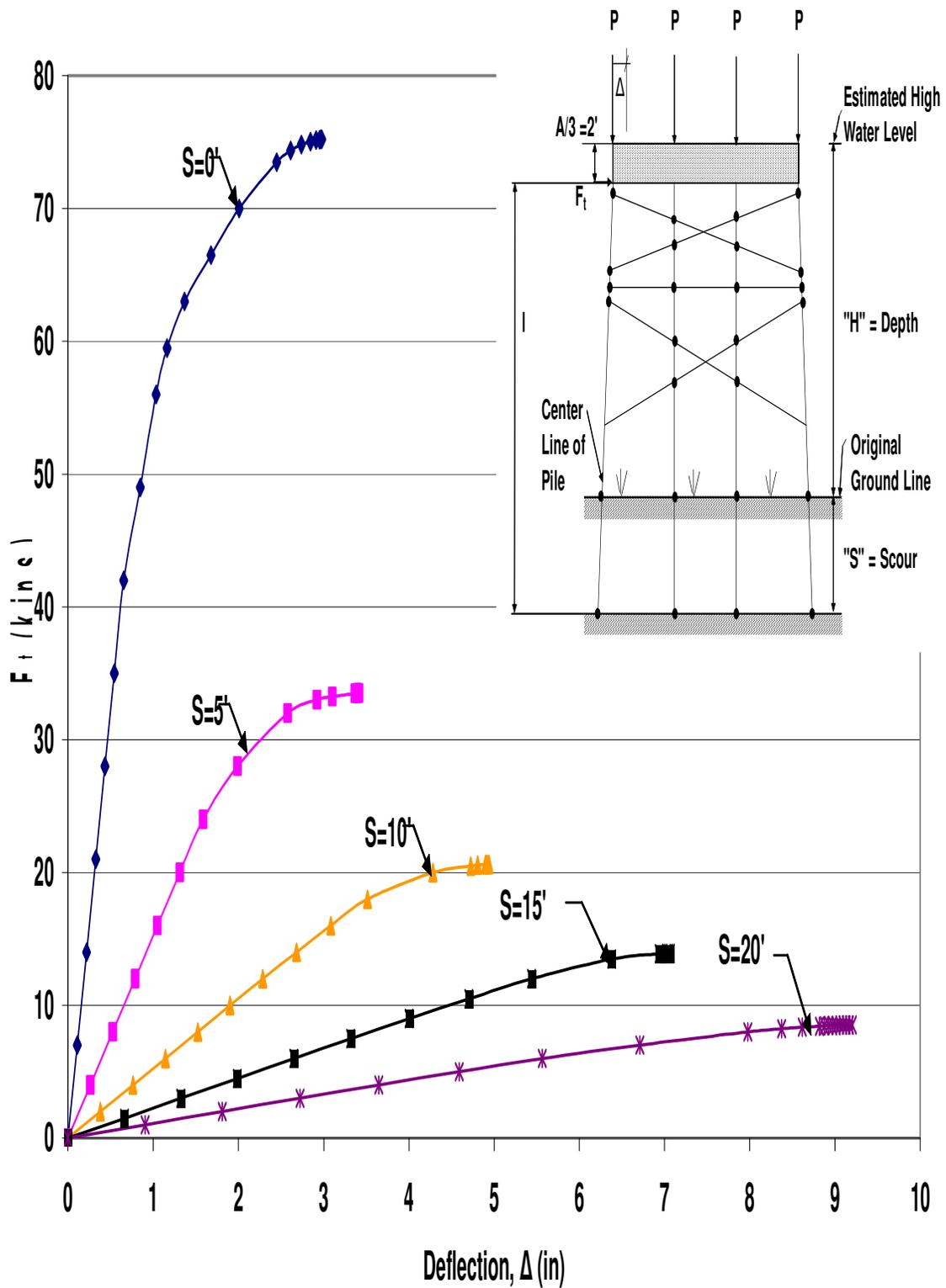
Figure B.44 HP12x53 Two-Story X-Braced 4-Pile Bent with  $H=21'$ ,  $P=160$ kips and  $A=6'$
