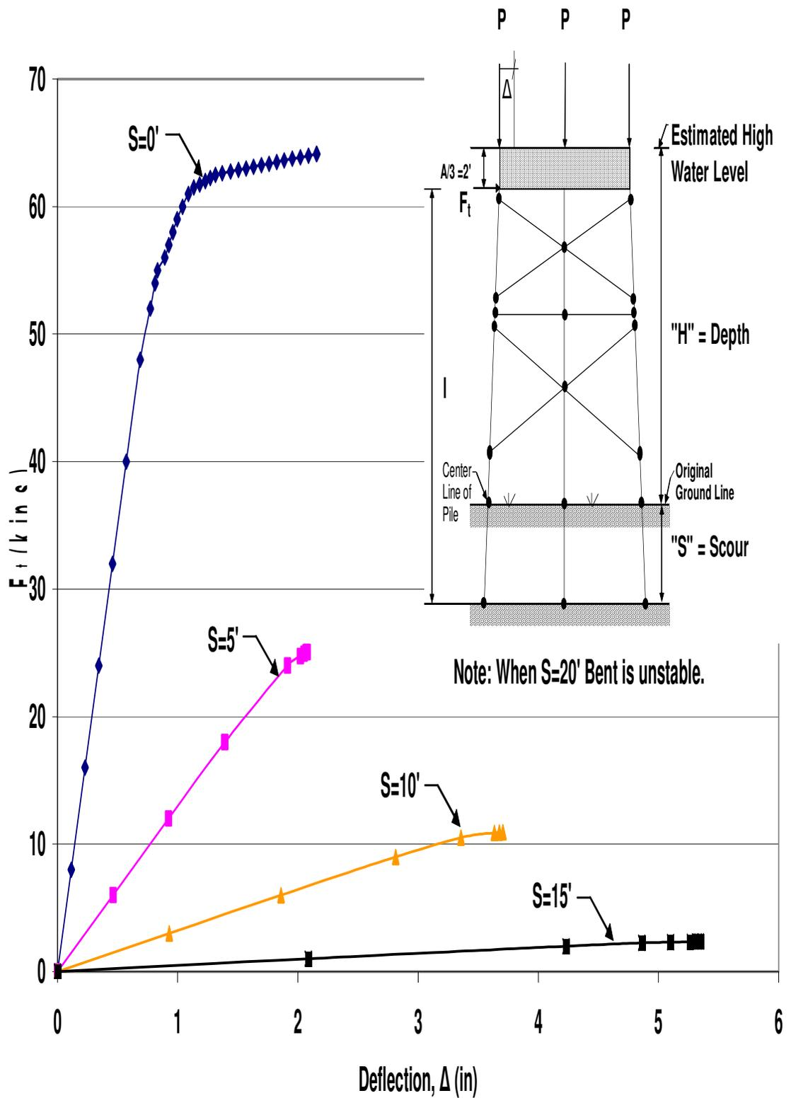
Figure B.23 HP12x53 Two-Story X-Braced 3-Pile Bent with H=25', P=140kips and A=6'
