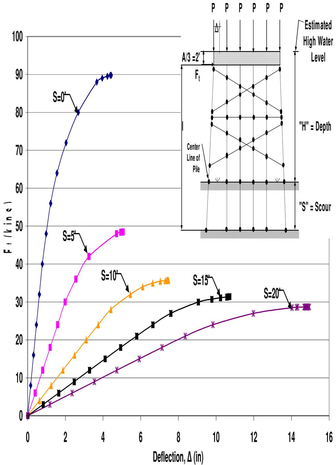
Figure B.102 HP12x53 Two-Story Single X-Braced 6-Pile Bent with  $H=25'$ ,  $P=120$ kips and  $A=6'$  Pushover Analysis Results
