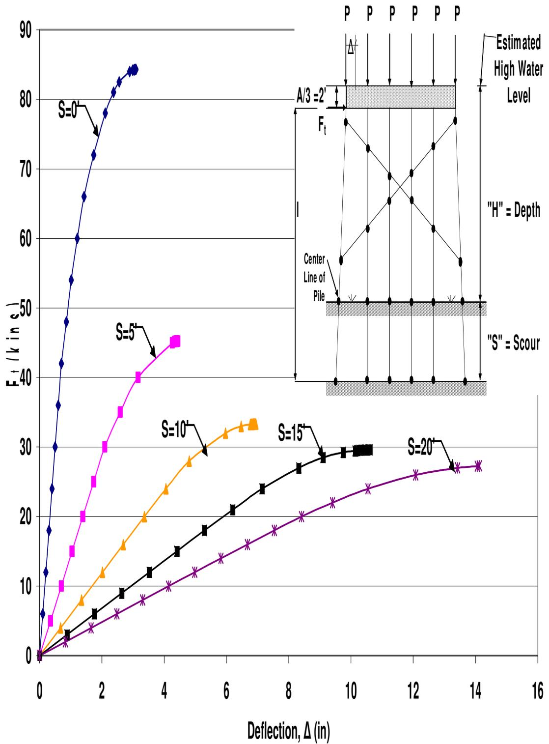
Figure B.87 HP12x53 Single X-Braced 6-Pile Bent with  $H=17'$ ,  $P=140$  kips and  $A=6'$
