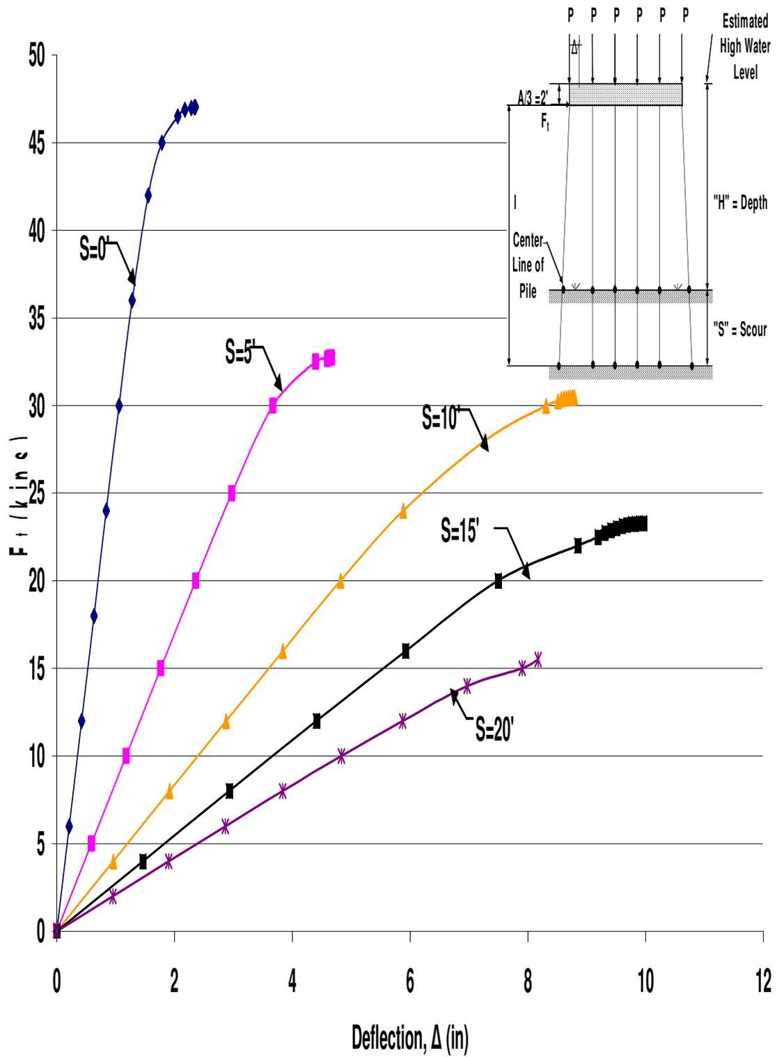
Figure A.74 HP10x42 Unbraced 6-Pile Bent with  $H=10'$ ,  $P=120$ kips and  $A=6'$
