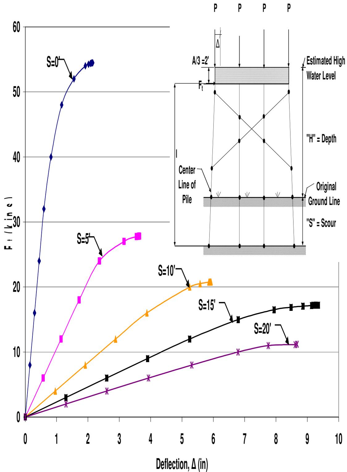
Figure A.33 HP10x42 X-Braced 4-Pile Bent with  $H=13'$ ,  $P=100$ kips and  $A=6'$
