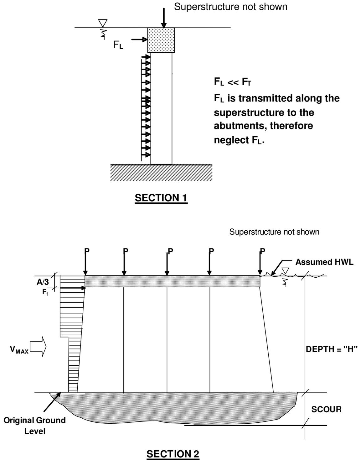
Figure 2.7 Sections Showing Longitudinal And Transverse Flood Water Loading on Bent (see Fig. 2.6)
