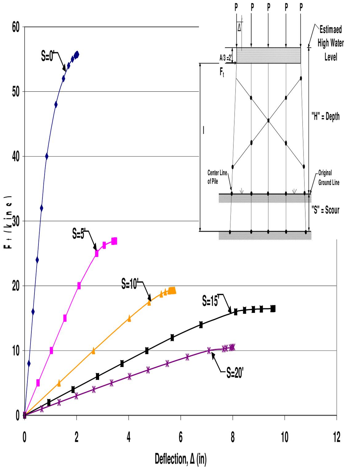
Figure A.59 HP10x42 X-Braced 5-Pile Bent with  $H=13'$ ,  $P=140$  kips and  $A=6'$
