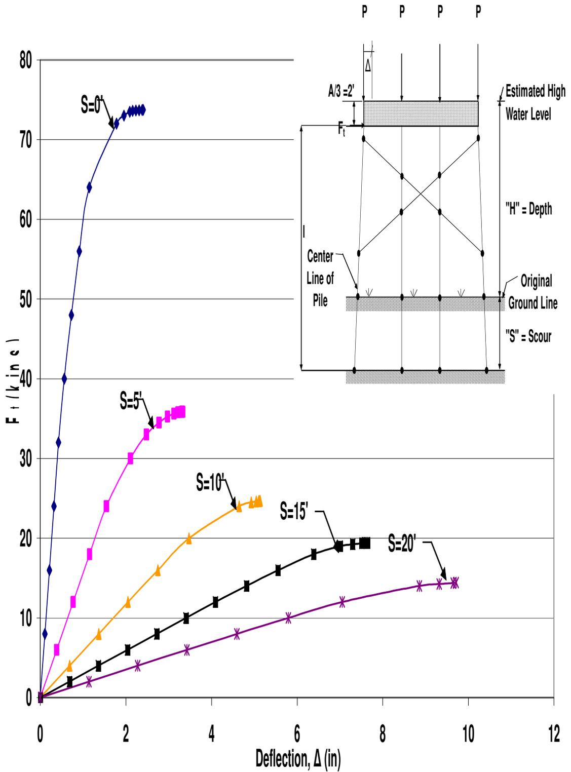
Figure B.36 HP12x53 X-Braced 4-Pile Bent with  $H=13'$ ,  $P=160$  kips and  $A=6'$
