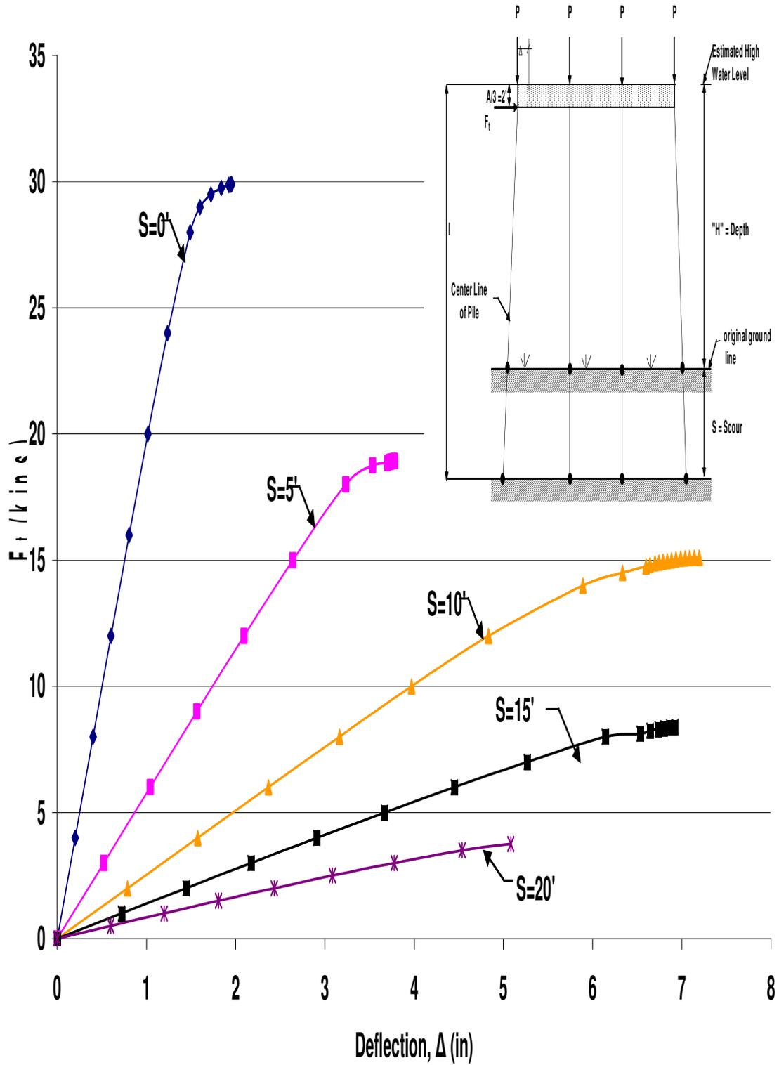
Figure A.28 HP10x42 Unbraced 4-Pile Bent with  $H=10'$ ,  $P=160$ kips, and  $A=6'$
