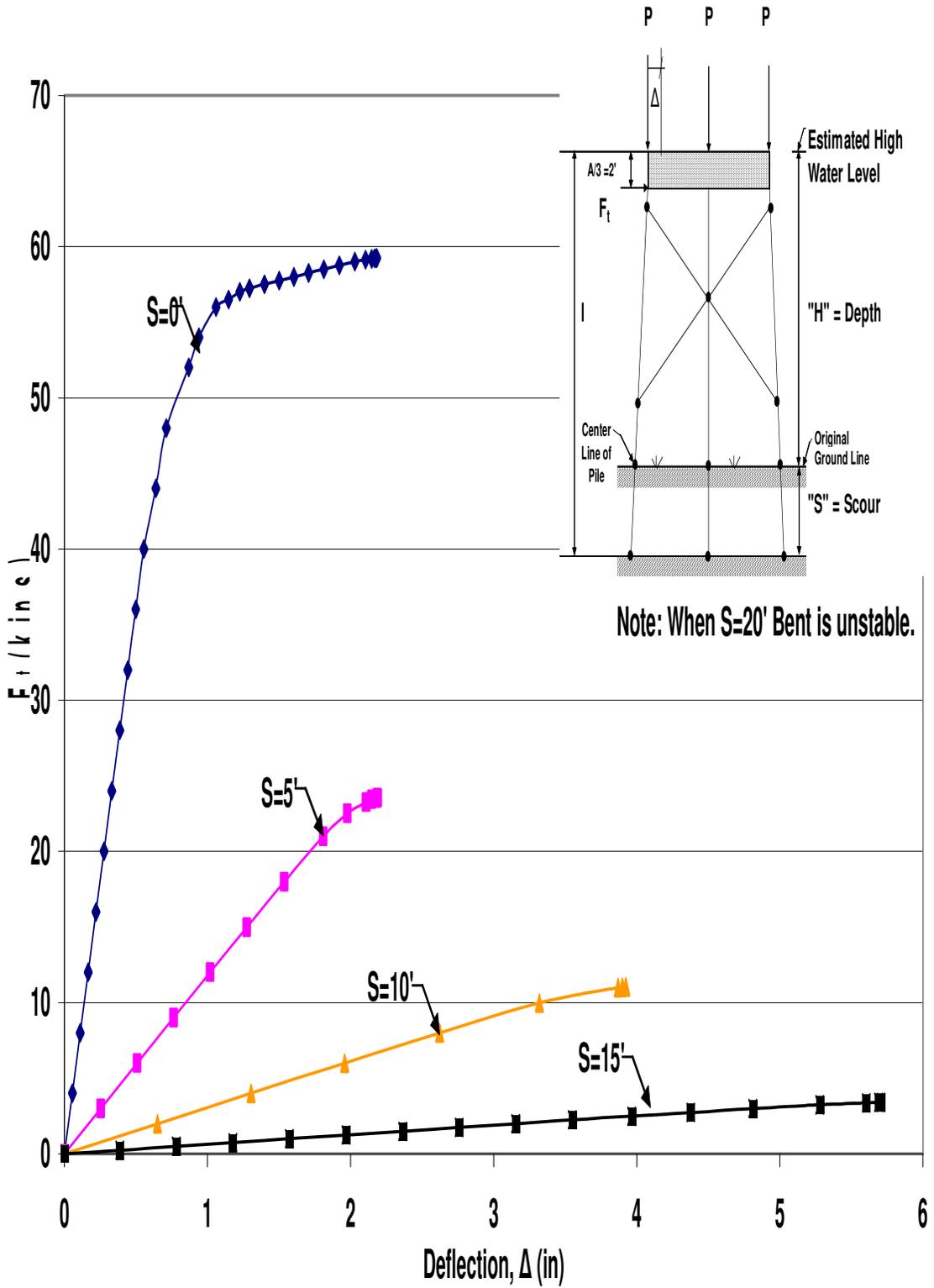
Figure B.15 HP12x53 X-Braced 3-Pile Bent with H=17', P=140 kips and A=6'
