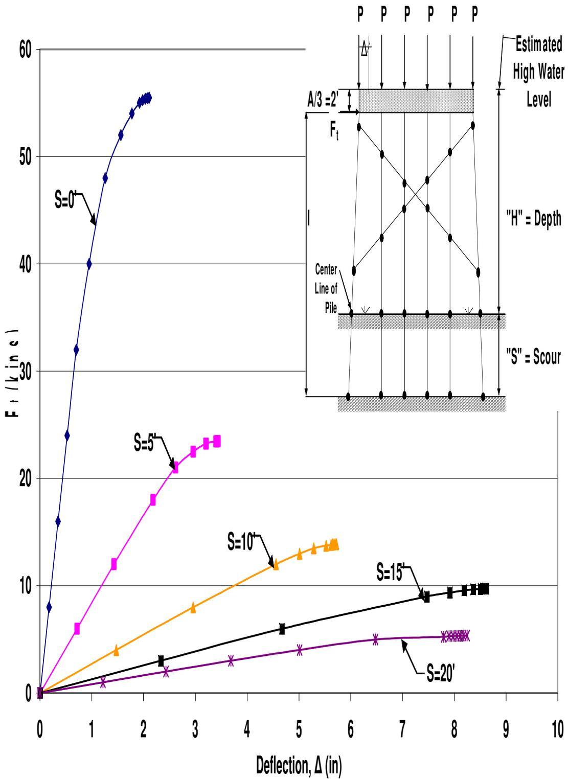
Figure A.84 HP10x42 Single X-Braced 6-Pile Bent with  $H=13'$ ,  $P=160$ kips and  $A=6'$
