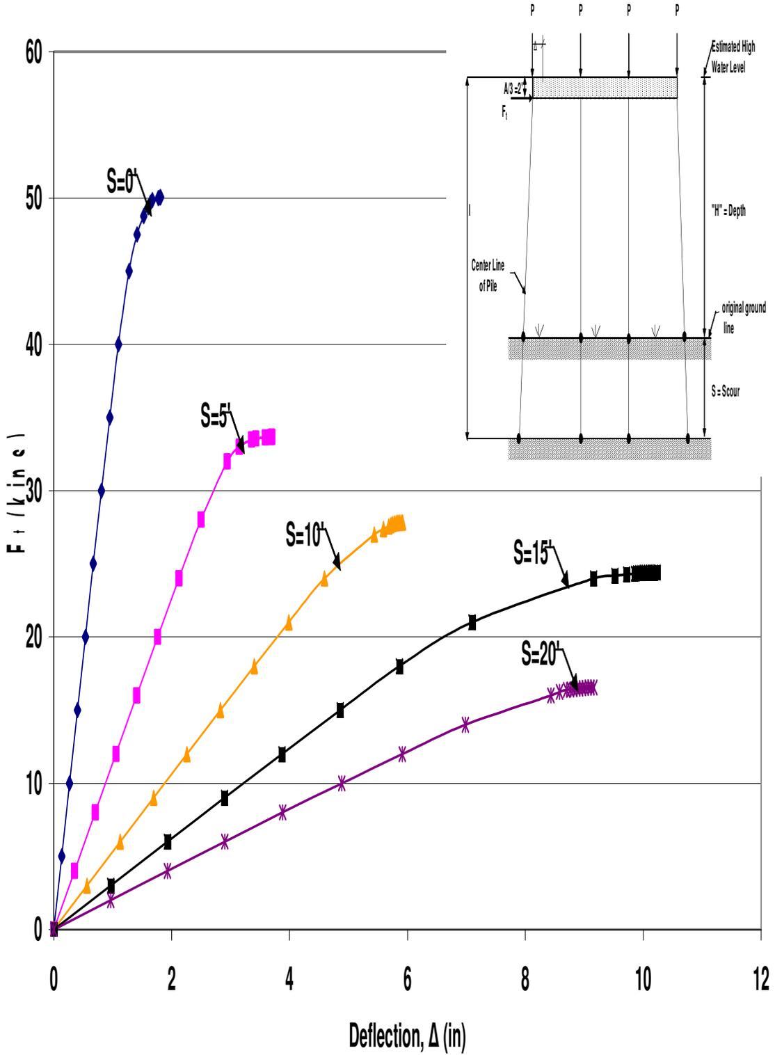
Figure B.28 HP12x53 Unbraced 4-Pile Bent with  $H=10'$ ,  $P=160$  kips and  $A=6'$
