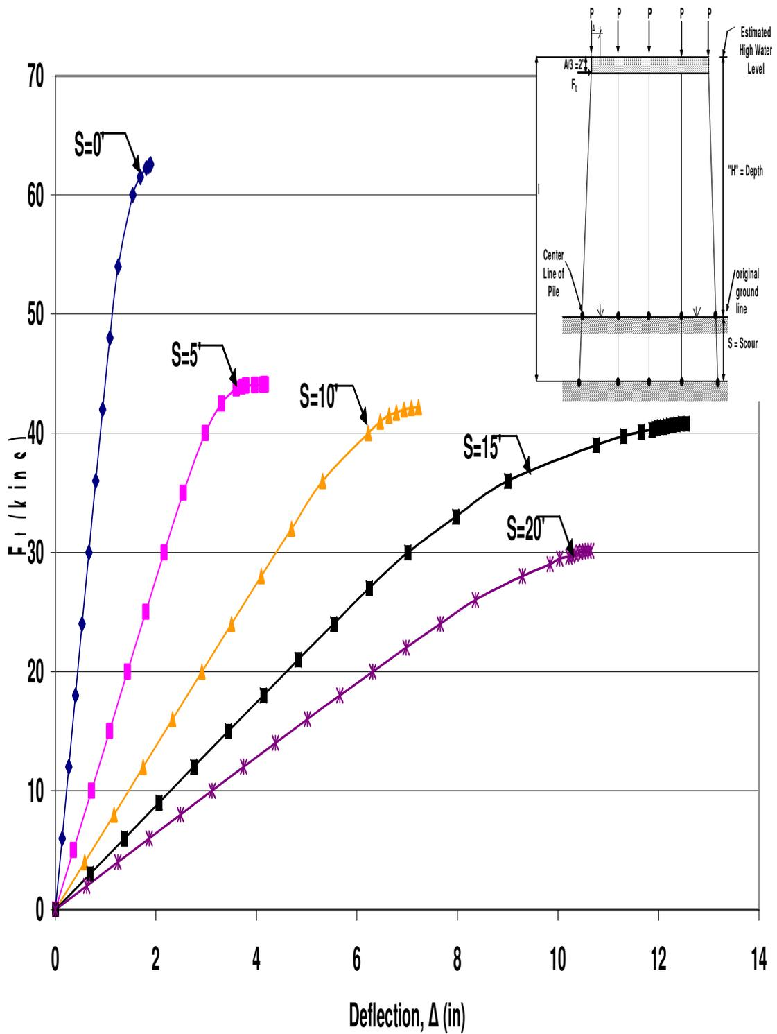
Figure B.51 HP12x53 Unbraced 5-Pile Bent with  $H=10'$ ,  $P=140$ kips and  $A=6'$
