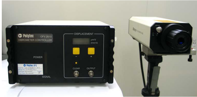
Figure 12: Non-contacting laser vibrometer system with sensor head and controller
