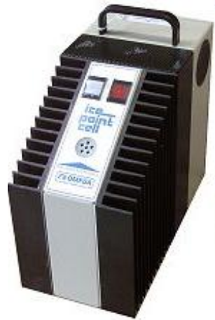
Figure 17: Ice point reference used to calibrate thermocouple
