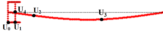
(a) The mode shape at 60Hz, around the first natural frequency
