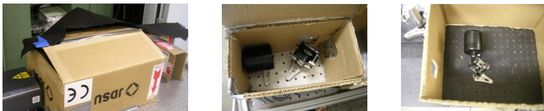
Figure 52: Cardboard Boxes to Block Ambient 532 nm Light
