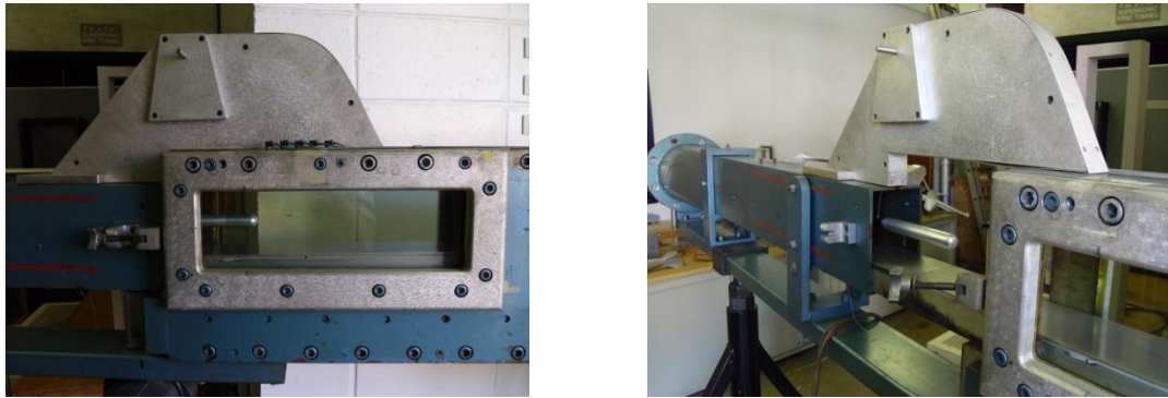
Figure 84: Easy Access to Supersonic Wind Tunnel Test Section
