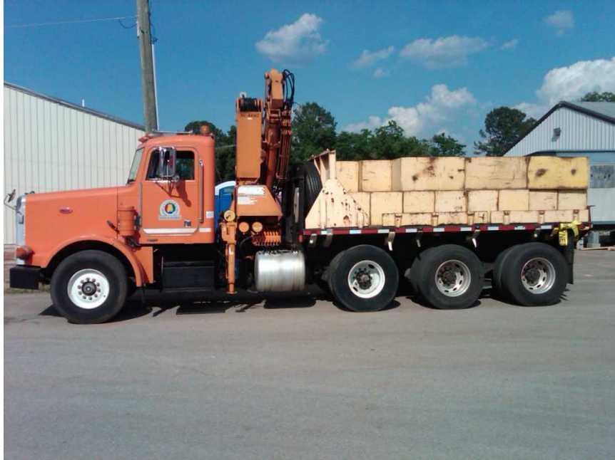
Figure 4-11: Standard load truck ST-6400 (pre-repair and post-repair)
