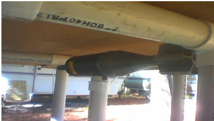
Figure 5.1 HEAT-T suspension in the test set-up
