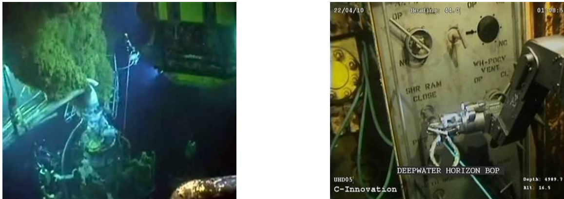
Figure 1.1: Underwater robots attempting to activate a blowout preventer.[10]
