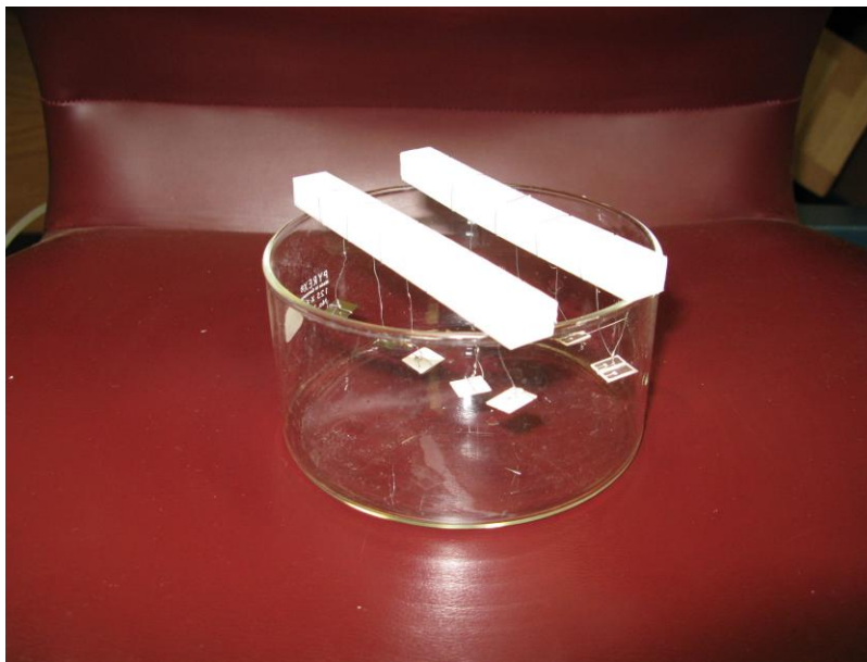
Figure 3.14 ZnO thin film coated substrates hang on the supporting bar by facing down
