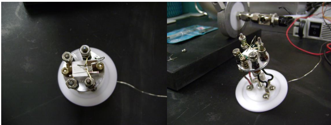
Figure 3.15 Hand-made apparatus to measure the resistance changes in a closed chamber.
