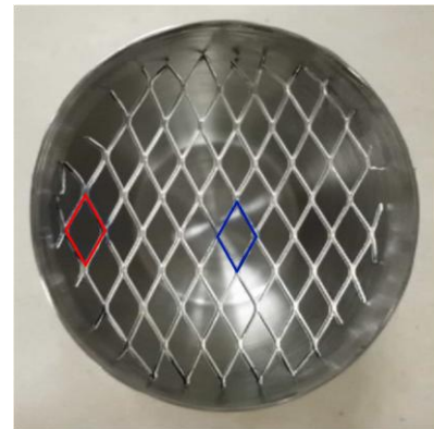
Figure 3.6: Holder to hold thermocouples in place.
