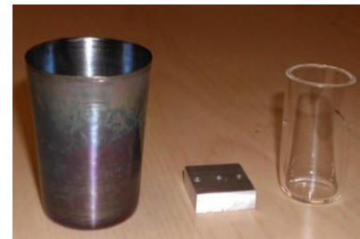
Figure 3.2: Steel crucible, Al slug, quartz crucible used in the experiments.
