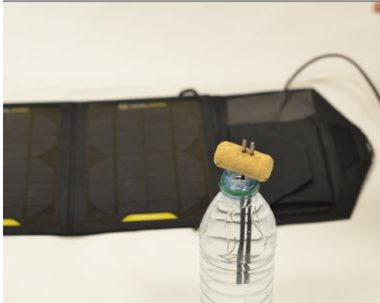
Figure A.7: Insert electrodes into bottle
