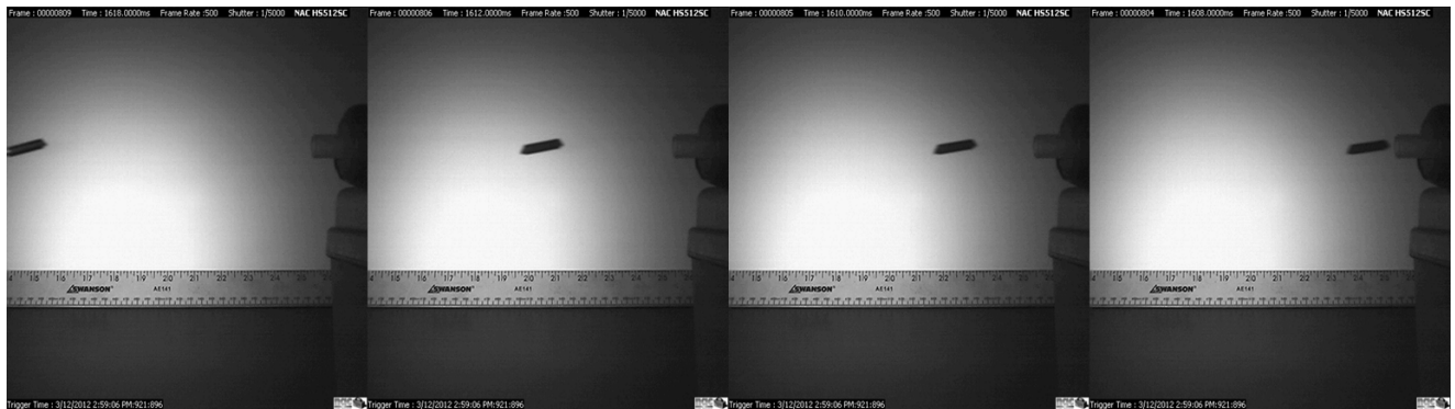
Figure 48: The flight path of the yarn carrier fired at 180 volts.
