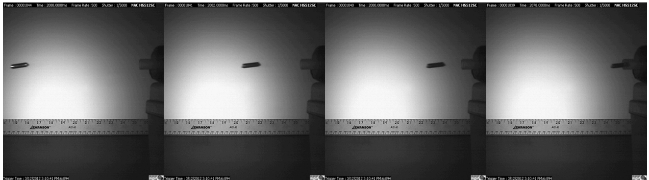
Figure 52: The flight path of the yarn carrier fired at 185 volts that flew straight.
