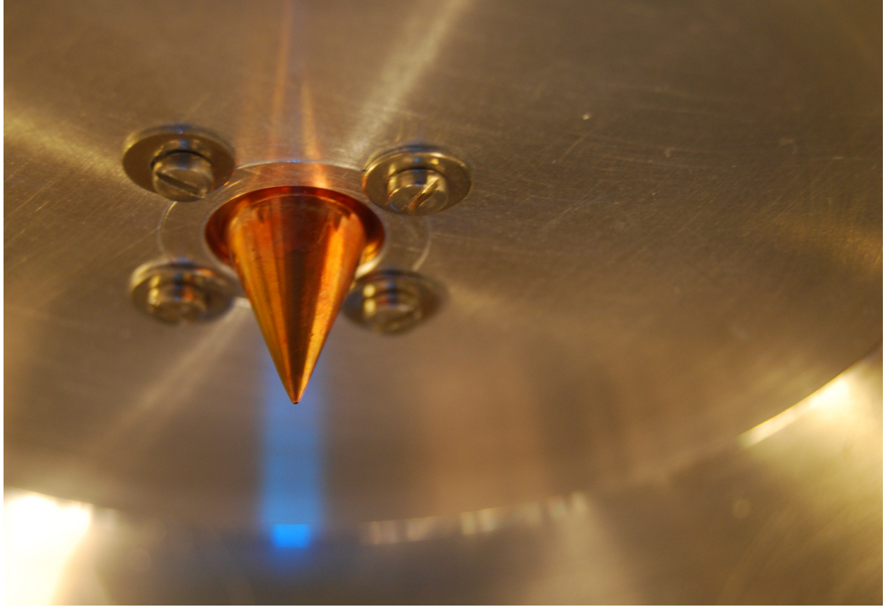
Figure 2.7: The skimmer used in the gas jet system.
