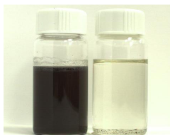
Figure 5.32: Effect of surface chemistry on SWNT dispersion. (left) Bingel SWNT filtered and (right) SP SWNT filtered.
