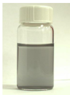
Figure 6.10: PVP (10 mg/mL) in water, tip sonicated for 30 min.
