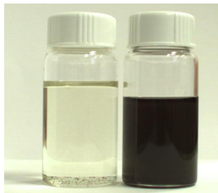
Figure 5.31: Effect of sonopolymer on SWNT dispersion. (left) SP SWNT filtered and (right) SP SWNT residue.
