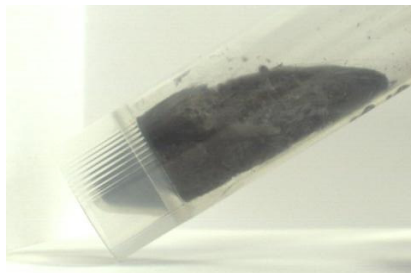
Figure 6.26: Freeze-dried PVP SWNT composite in 50 mL polypropylene centrifuge tube.
