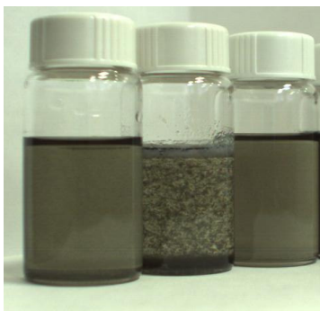
Figure 3.52: Lack of dispersion for styrene SWNT in UPR.
