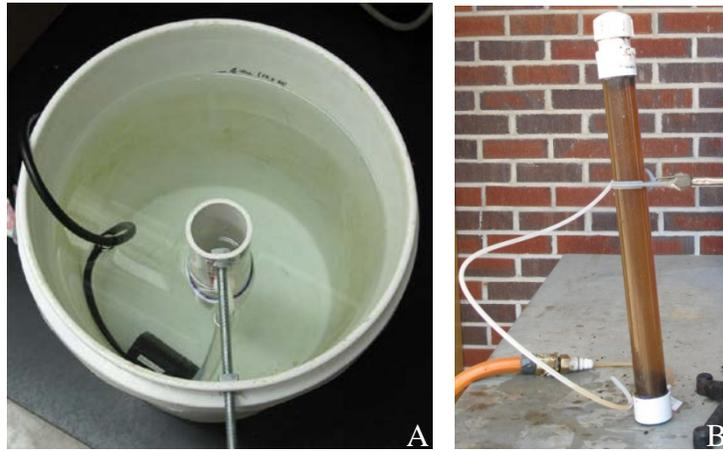
**Figure 1.** Tank mix model (A); Process column model (B).
