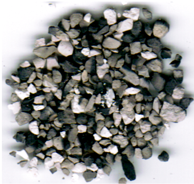
Figure 2.1: 4 wt% Ag/TiO 2 adsorbent - 2.5× magnification
