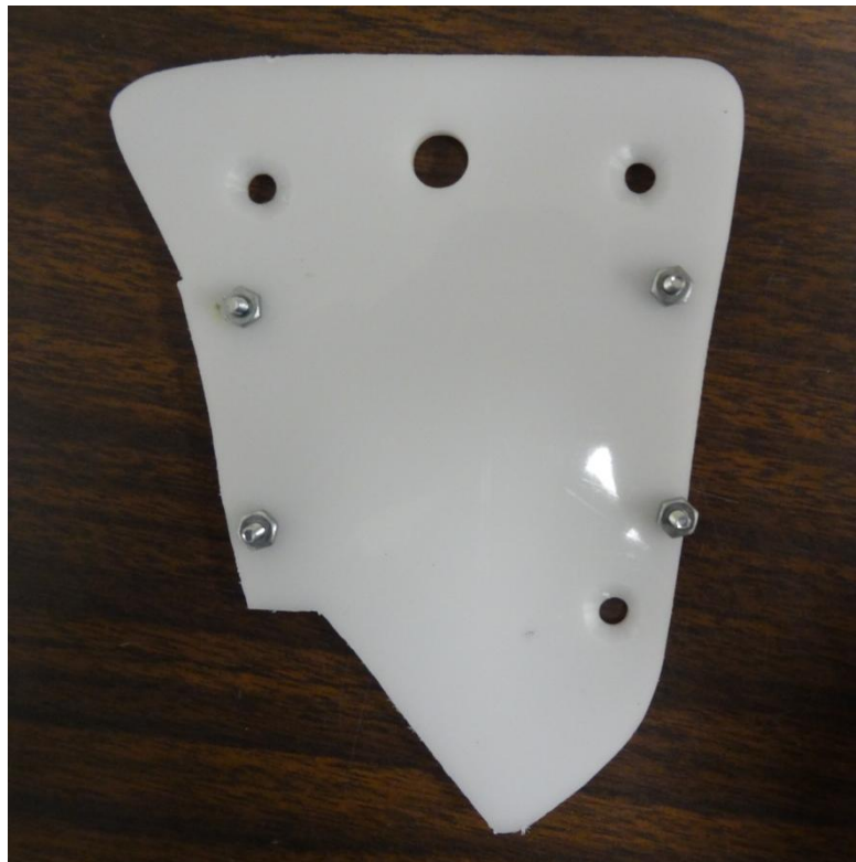
Figure 24 transmitter attachment plate
