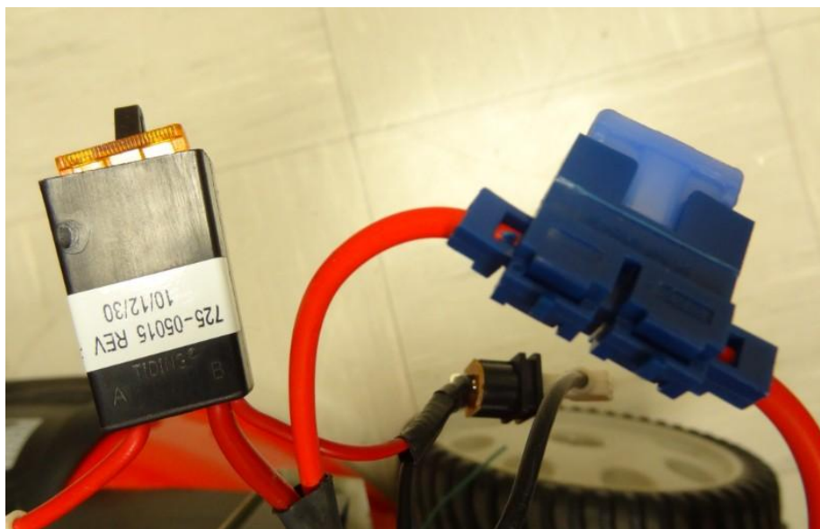
Figure 41 fuses to protect the battery
