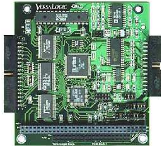
Figure A.3: Versalogue PC/104 data acquisition board [Versalogue, 2005b]
