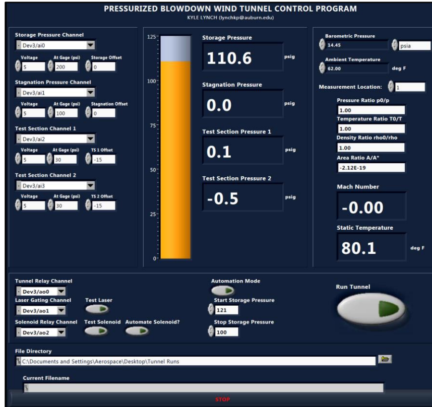
Figure 25: LabVIEW Visual User Interface for Tunnel Controller
