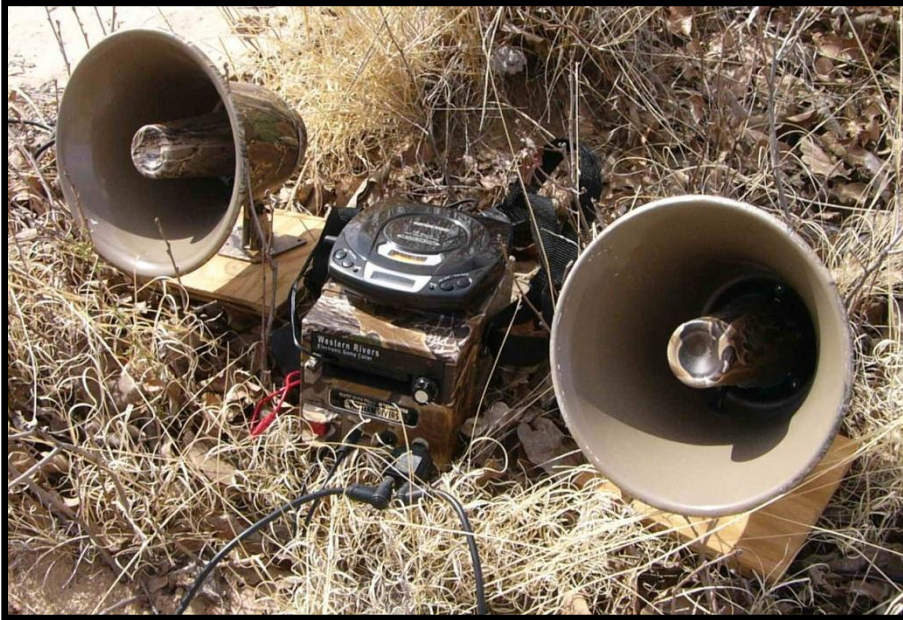
Figure 1.1—Audio system consisting of a modified, continuous-play, electronic, game caller, and two weatherproof speakers.
