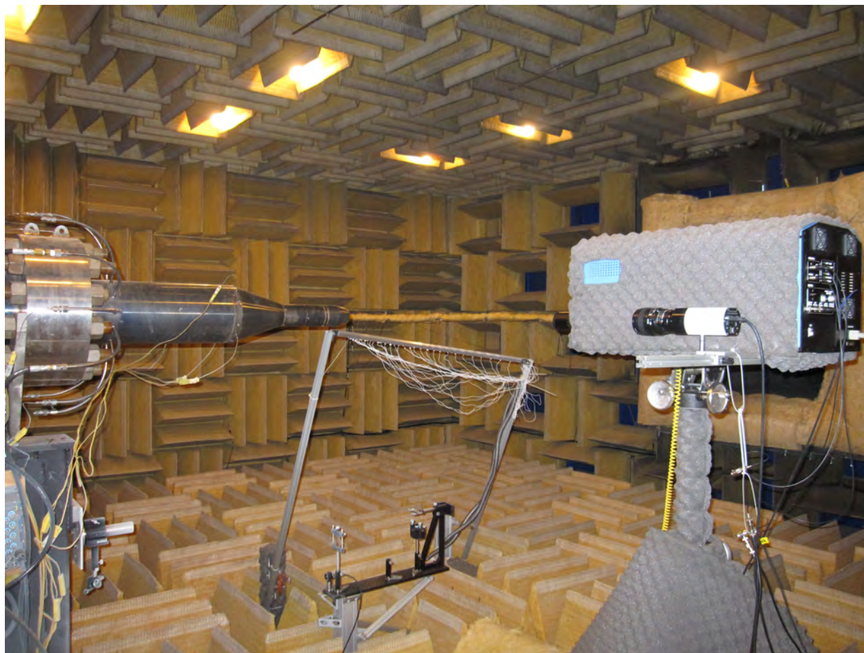
Figure 3.1: Experimental setup in the test chamber of the Anechoic Jet Laboratory (AJL).
