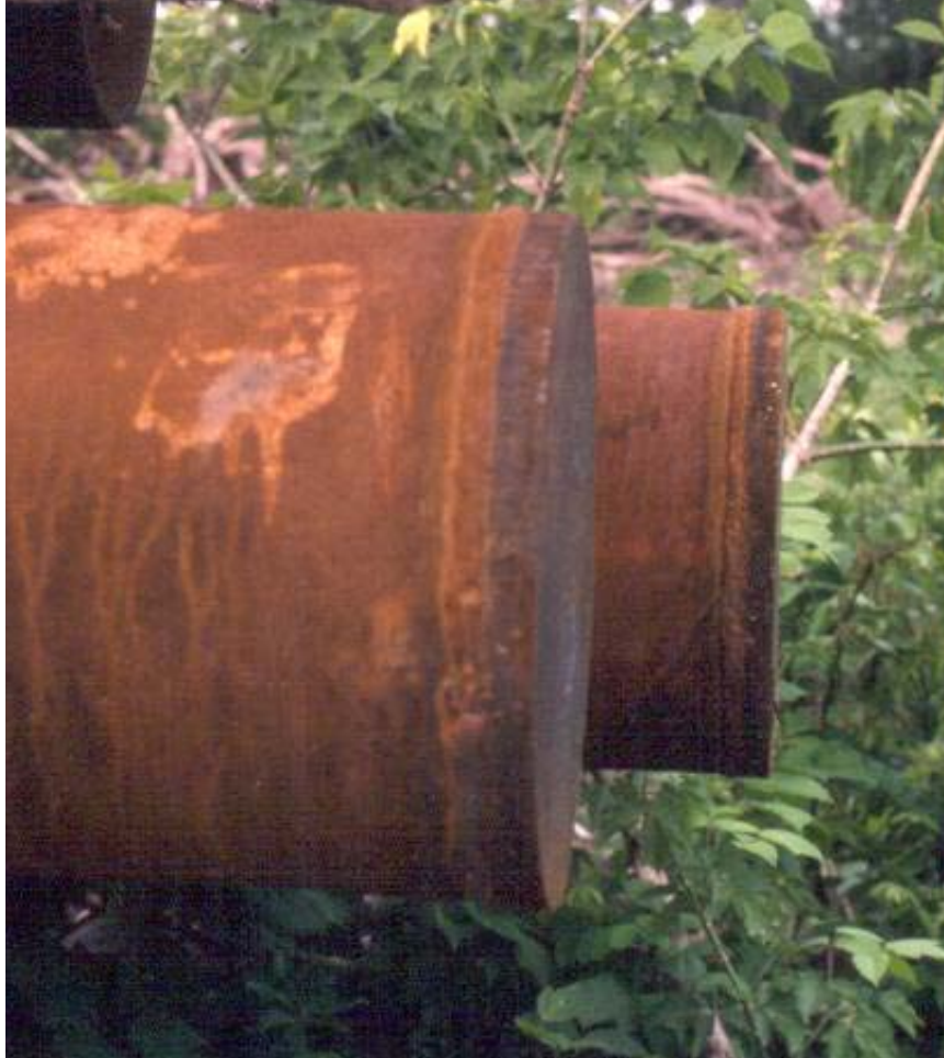
Figure 2.4. Closed-end steel pipe pile (Hannigan 2011)
