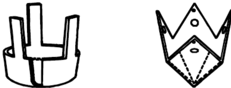
Figure 2.1. Pile toe protection devices (Hannigan et al. 2006)
