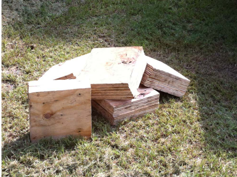
Figure 3.17. 6 in. (15 cm) plywood pile cushions
