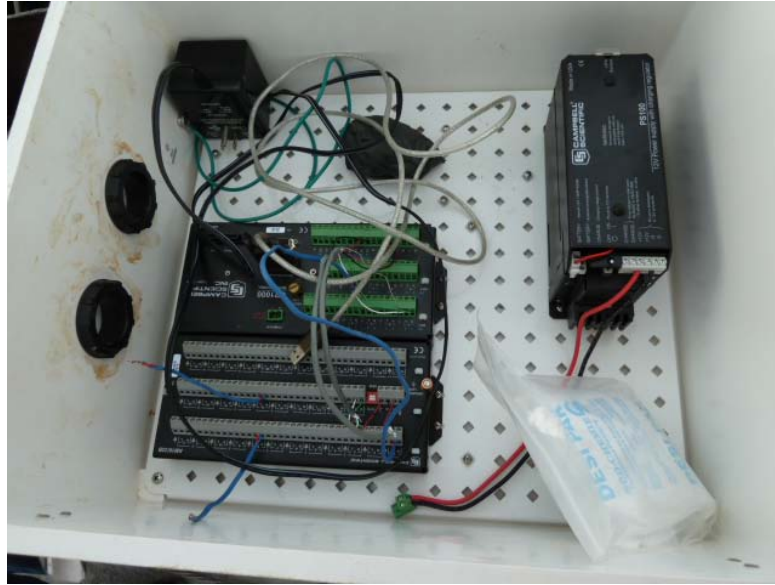
Figure 3.12. Datalogger with multiplexer for field cure thermocouples
