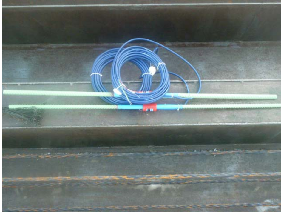
Figure 3.6. No. 4 sister-bar strain gages
