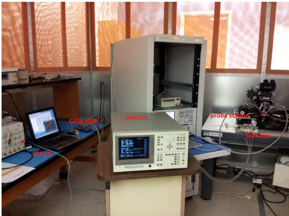
Figure A.1 DC measurement system setup
