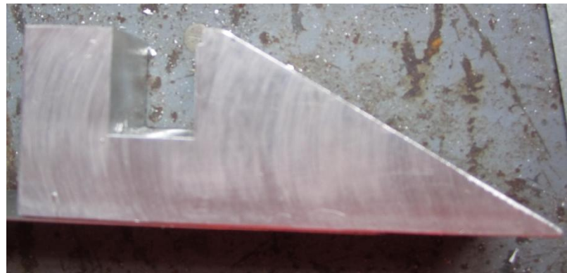
Figure 4.6. Hook-SH3 was triangular shaped, and acted as a wedge causing separation between individual slips.
