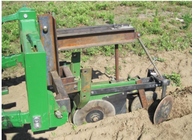
Figure D.1. Side view of the designed disc mechanism used to open and close the furrow around the slip.
