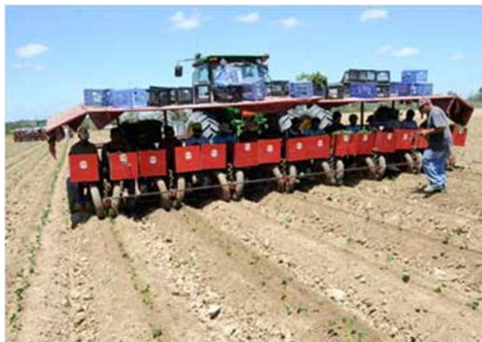
Figure 1.1. An 8-row sweet potato transplanter requires one tractor operator and two operators per row that alternate feeding slips.
