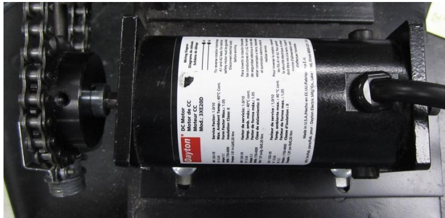
Figure A.1. A Dayton DC motor, (3XE20D) mounted to Prototype-2, mechanizing the range of motion of the hook mechanism.
