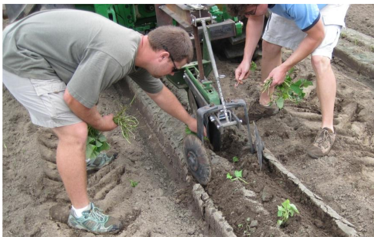
Figure D.3. Slips being manually transplanted between the discs of the prototype planter.
