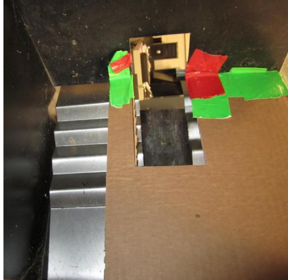
Figure 5.3. A view inside bin showing the front baffle. Note Baffle-2, the rippled baffle on the left, the ridges are visible due to the non-symmetric design of the front baffle which was required to due to volume slip leaves added.
