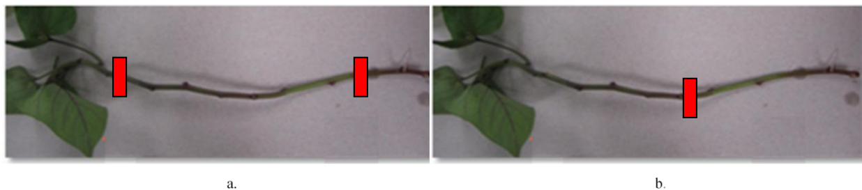
Figure 4.3. Illustration of the two contact configurations evaluated for singulating sweet potato slips; two contact points (a) versus one at the center (b).
