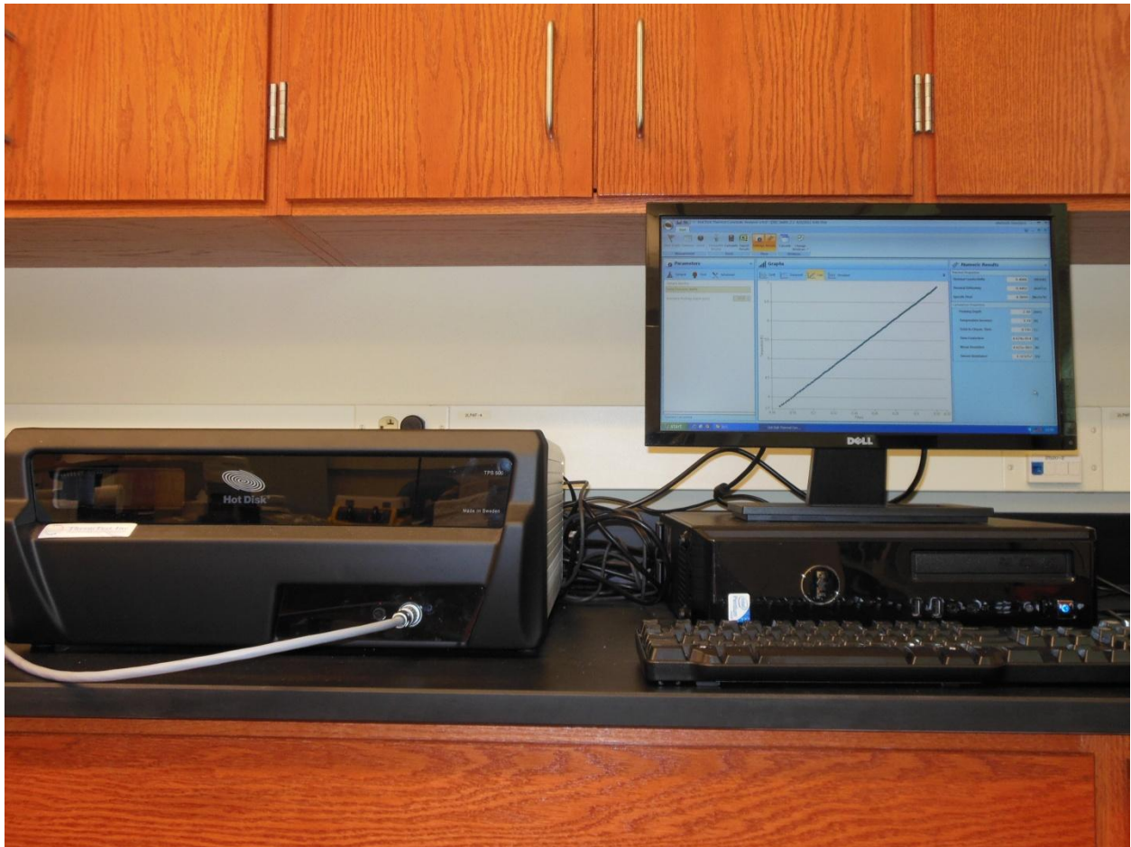
Figure 3.7 Photograph of the Hot Disk thermal constants analyzer (TPS 500, Hot Disk AB, Gothenburg, SWEDEN)
