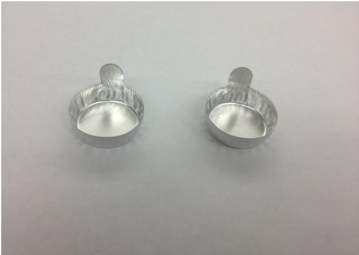
Figure 3.3 Photograph of pre-fabricated 1 inch in diameter aluminum foil molds (VWR ® International LLC., Model 611-1362)
