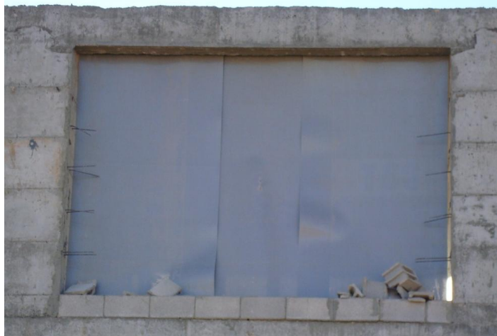
Figure 6.7: Post Test Wall (Johnson 2009)
