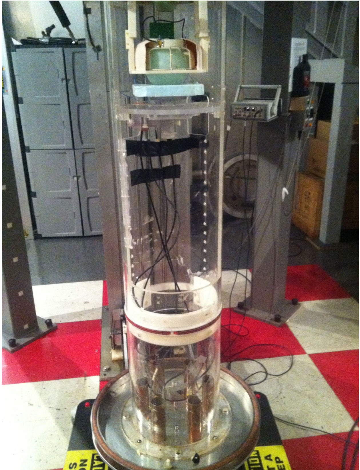
Figure 4.4 The birdcage coil and a water phantom inside the MRI scanner. (a) Front side view
