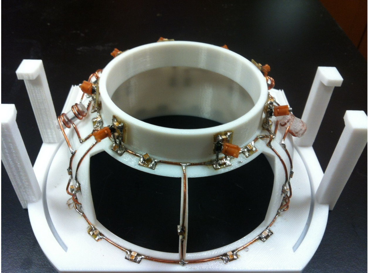
Figure 5.1 An 8-ch transmit and receive phased array coil
