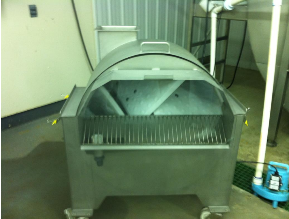
Figure 3. The picture of decontamination tank (COPE unit, Morris & Associates Inc., Garner, NC) used in this study.
