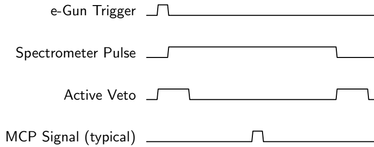
Figure 2.13: Timing diagram for the pulsing sequence. The electron gun trigger (width \sim 100 ns) is the reference point starting the timing sequence, setting the time zero. The spectrometer pulse is activated shortly after the electron gun pulse (lasting \sim 10 \mu s), and a signal veto covers the time during which the spectrometer pulse is turned on and off to ignore interference effects caused by the rapid pulsing of the spectrometer field. A typical MCP signal would arrive \sim 5 – 8 \mu s after the electron gun trigger.
