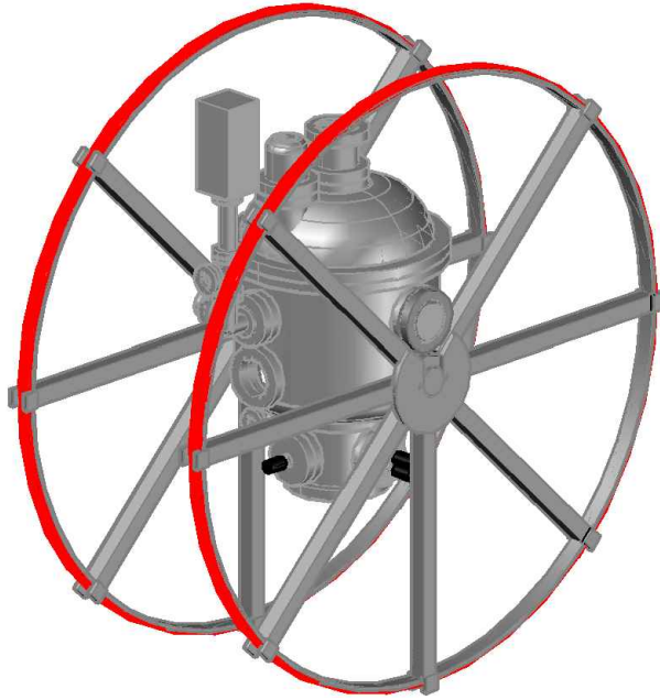
Figure 2.9: Illustration of the apparatus with Helmholtz coils attached. The coils are attached to the chamber around the electron gun feedthrough, approximately coaxial with the electron beam.
